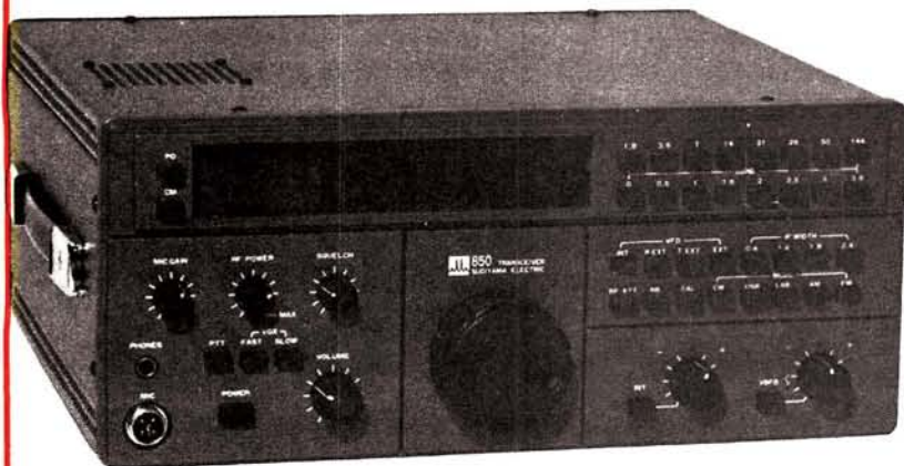
Front panel view of the F850 showing the various controls and indicators. The frequency is displayed as a digital readout with an analogue S meter to its left
