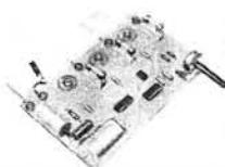
**KS262 10 CHANNEL CHASE LIGHT CONTROL UNIT.** 350W per channel, variable speed, operates from 240V A.C., uses 10 x triacs, 10 x BC208-B, 2 x I.C.s. £18.63 Inc VAT
