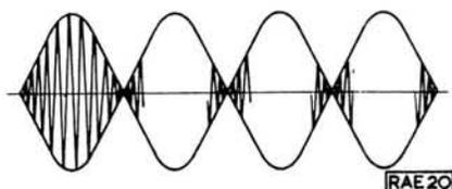
**Fig. 69: Oscilloscope display of an s.s.b. signal modulated by two sinusoidal tones of equal amplitude**
