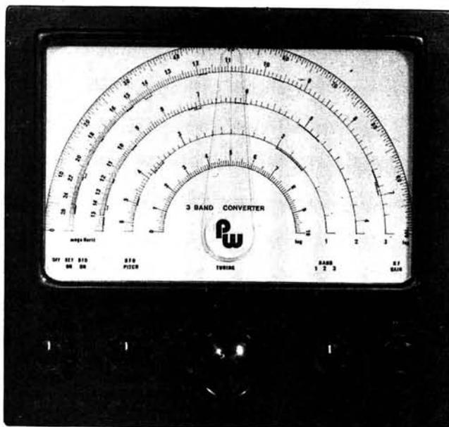
Fig. 7: Showing the tuning scale
