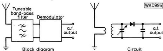
**Fig. 70: "Crystal Set"—absorption wavemeter**
