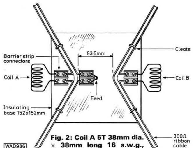
Fig. 2: Coil A 5T 38mm dia. x 38mm long 16 s.w.g.,
