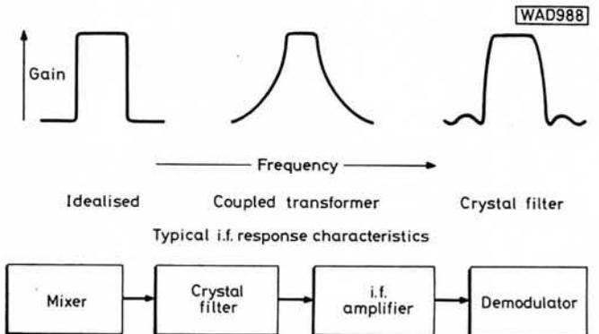
Fig. 75: Using a crystal filter to obtain i.f. selectivity
