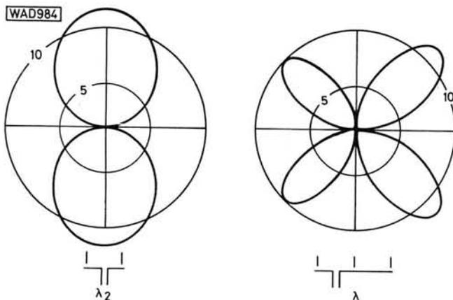
Fig. 1: Radiation patterns, (left) centre fed  $\lambda/2$ , (right) offset fed  $\lambda$
