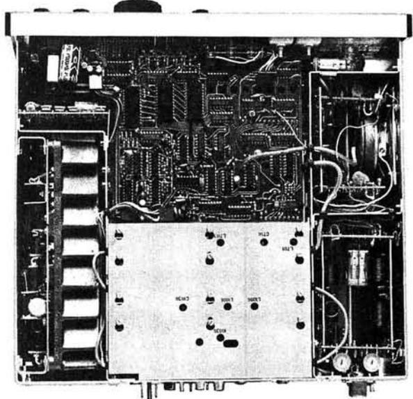
Front and rear views of the TR-7 and PS-7, and what they look like inside. The p.a. heatsink is mounted internally, to allow forced draught cooling by the optional fan
