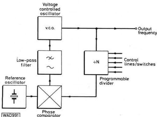
Fig. 74: Basic variable frequency synthesiser
