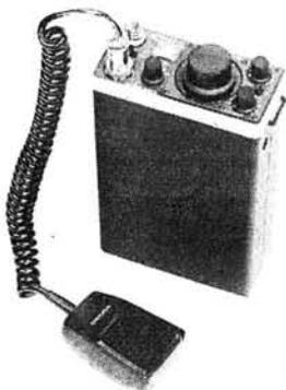
For those of you who enthuse over portable SSB operation on the hills and mountains of the UK, or wish to chat to the local lads whilst seated by your fireside, then the Mizuho SB2X 2 metre SSB portable is the rig for you. One watt output on the SSB frequencies 144.000 to 144.600 and the ability to listen to the beacon frequencies from 144.800 to 145.000 (also transmit).
