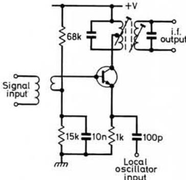
Fig. 73(a):  $\blacktriangle$  Transistor mixer stage
