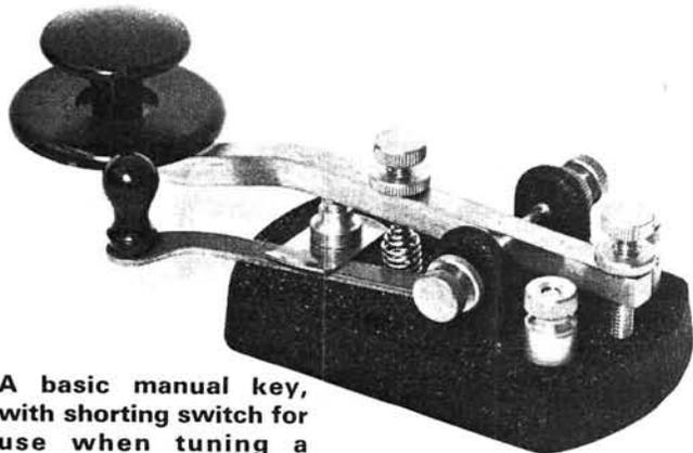
A basic manual key, with shorting switch for use when tuning a transmitter
