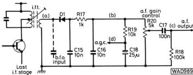
Fig. 76: Circuit of a basic a.m. (envelope) demodulator
