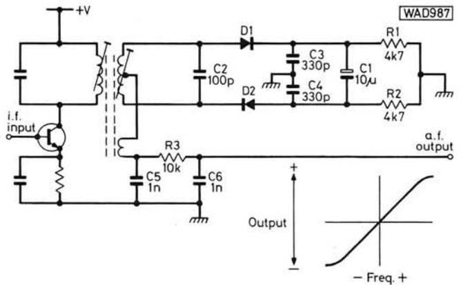
Fig. 78: Ratio detector f.m. demodulator
