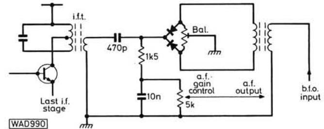
Fig. 77: The balanced demodulator
