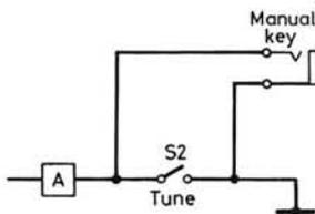
**Fig. 3 (right): A socket for a manual key can be connected across the TUNE switch**
