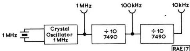
**Fig. 66: Block diagram of a crystal calibrator unit**
