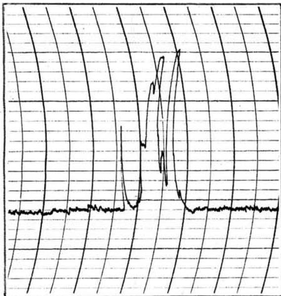
**Fig. 1: One of the many one-minute duration solar bursts recorded by the author in November**
