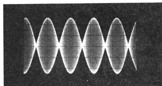
Fig. 2: Two tones of equal amplitude on s.s.b.
