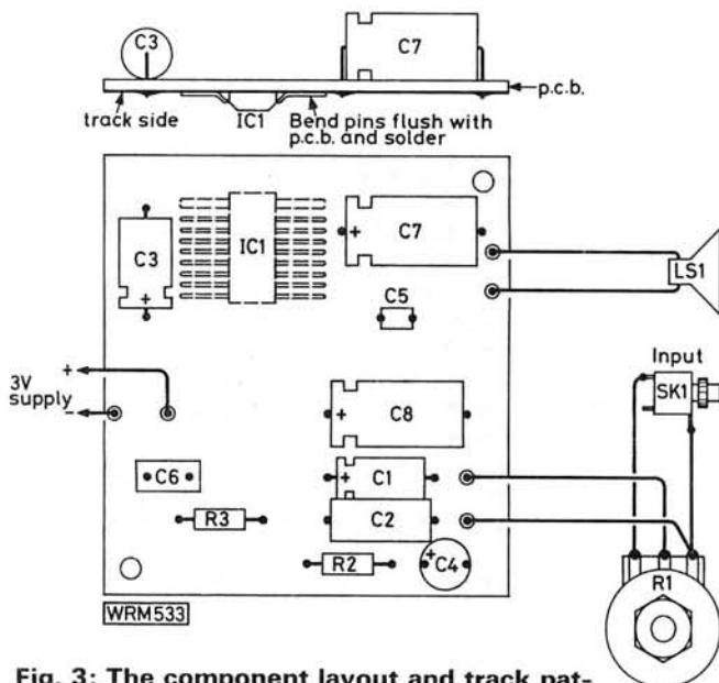
Fig. 3: The component layout and track pattern shown full size
