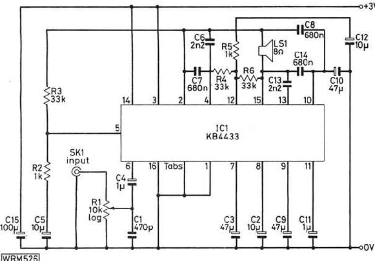
**Fig. 5: The circuit diagram of the 250mW bridge amplifier**
