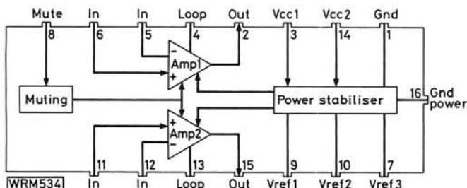
Fig. 1: Block diagram of the KB4433
