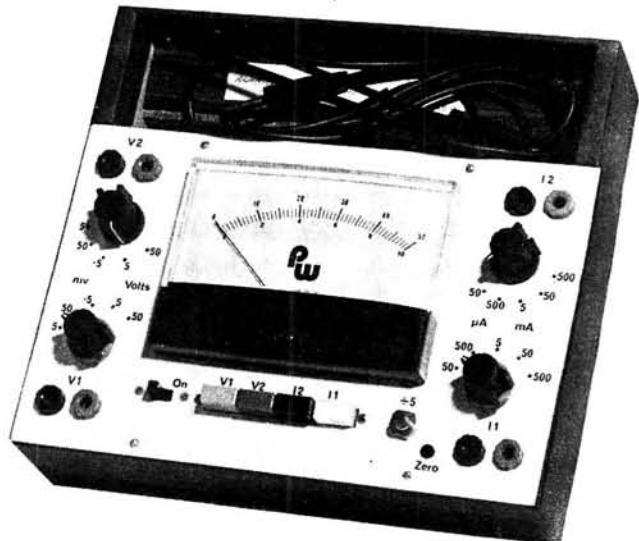
Each t.p. would have to be completely isolated by the 4-way selector switch, so that they could be scattered anywhere around a circuit, and be at different potentials.
