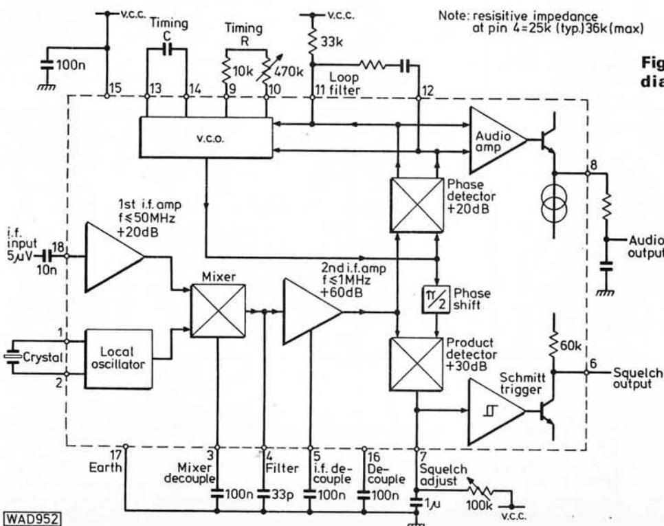
**Fig. 3: SL6600C internal block diagram with basic external components**
