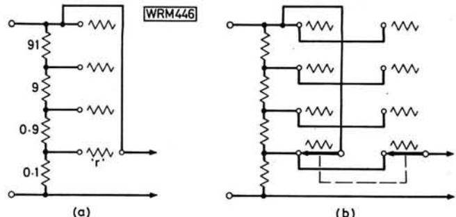
**Fig. 2: Overcoming problems due to switch contact resistance on the current ranges**
