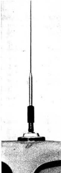
**A mag-mounted series-fed mobile CB antenna that meets the HO requirements. The design is similar to 1 (a) but the inductance is Ferrox cored**
