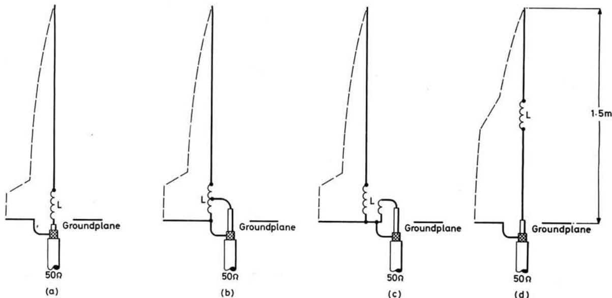
**Fig. 1:** (a) Series-fed antenna with inductive loading at the base. (b) Shunt-fed by tapping into the loading coil at the base. (c) Link coupled shunt-fed base coil. (d) Centre loaded series-fed (see text).
