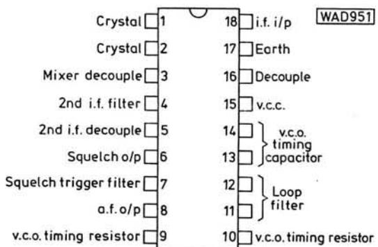
Fig. 2: Connections of the SL6600C
