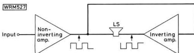
Fig. 4: A bridge amplifier drives the loudspeaker from antiphase outputs, thus increasing the maximum output power for a given supply voltage
