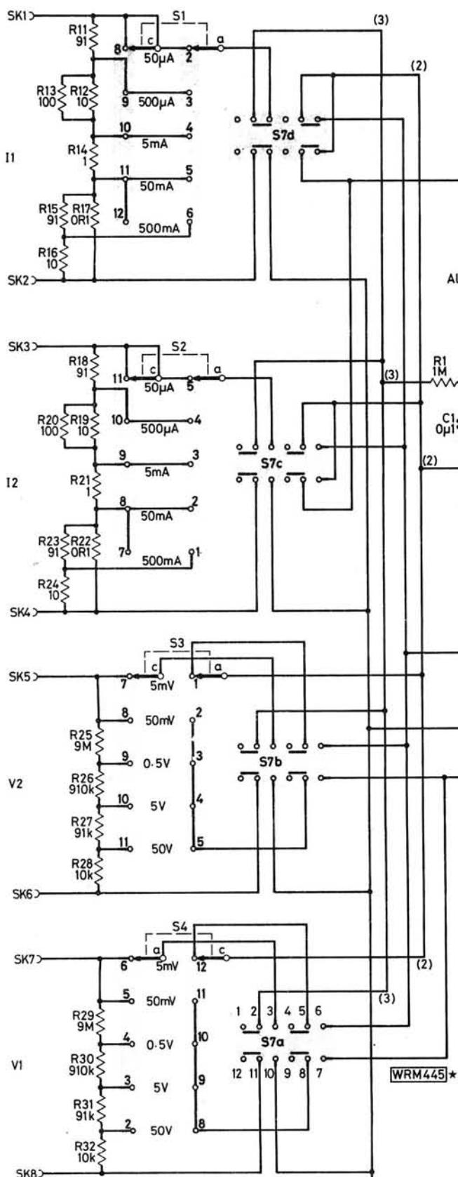
**Fig. 1: Complete circuit diagram of the Quadmeter. Note that resistors R33 and R34, both  $10\Omega$ , should be shown connected in parallel with R14 and R21 respectively**
