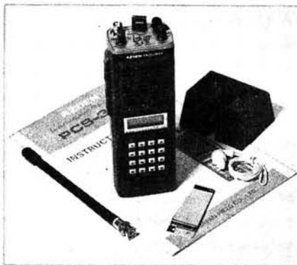
i.f.s. Receiver sensitivity is quoted as less than 0.2μV for 12dB SINAD over the complete bandwidth, with an audio output level of 200mW from the combined built-in speaker microphone.
