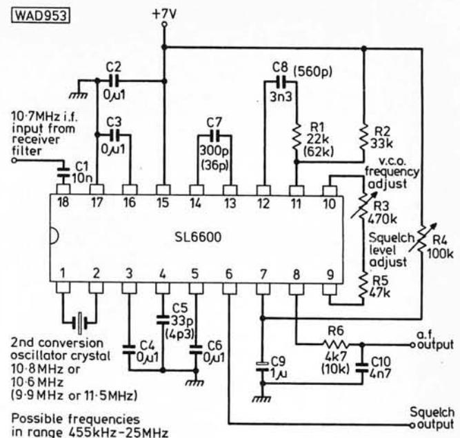
**Fig. 4: A narrow-band f.m. i.f./demodulator circuit using the SL6600C (wide-band component values in brackets)**
