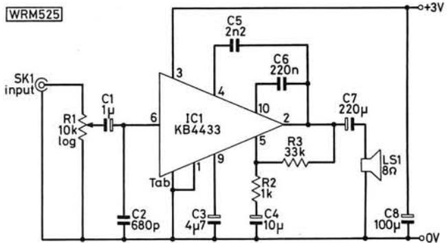
Fig. 2: A simple amplifier circuit using the KB4433 device
