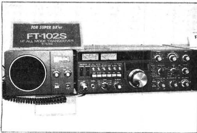
**The Yaesu FT-102S (the low-power version) plus the SP-102 loudspeaker with switchable a.f. filters**
