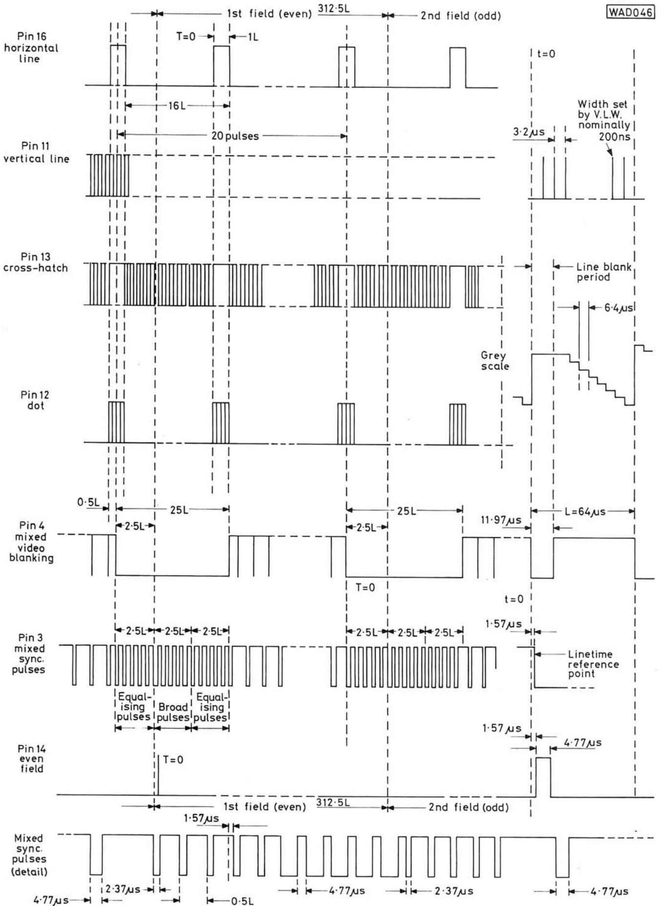
Fig. 3: Waveforms from the ZNA 234 in 625-line mode
