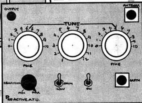
The unit described in this article is suitable for use over the approximate frequency range of 750kHz–25MHz, i.e. the greater part of both Medium and Short wavebands. A conventional antenna tuning unit (a.t.u.) enables almost any antenna, long or short, to be matched to a receiver, ensuring maximum transfer of r.f. energy from the antenna to the receiver's input stage.
