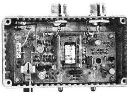
The review sample was tested on a rather ancient and "deaf" v.h.f. communications receiver, giving quite a worthwhile boost to performance, and also with an h.f. amateur bands transceiver. The extra gain was successful in lifting US f.m. repeaters around 29.6MHz out of the mush and turning them into readable signals. On the bench, gain was measured at 9dB with a ripple of less than 0.5dB up to just over 170MHz. At 190MHz gain was down by 0.5dB and at 200MHz by 1dB.
