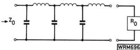
Fig. 1: Analogy of a transmission line
