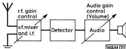
right-hand box is the audio section where speech and music are amplified before being applied to the loudspeaker. The arrow through the audio box means that the gain can be adjusted and this is the job done by the volume control. Audio gain is another name for volume control.
