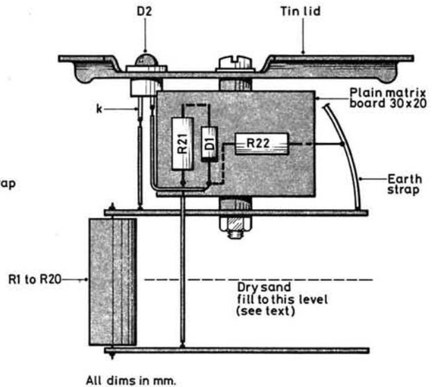
**Fig. 3: Full constructional drawings of the 50 ohm, 30MHz dummy load. Any suitable tin with a press-in air-tight lid can be used to house the completed resistor assembly. The earthing straps between the SO239 socket fixing screws and the top plate (Plate A) are important and should not be omitted even if brass pillars are used between the lid and top plate**
