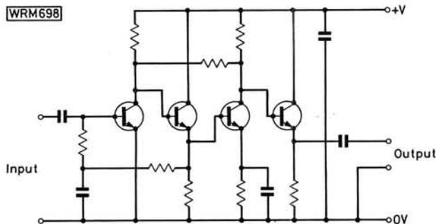
Fig. 1: Basic wideband gain-block
