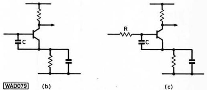
**Fig. 16: (a) Similarity between a diode detector circuit and an audio amplifier stage. (b) and (c) Adding suppression components to prevent "detection" taking place**
