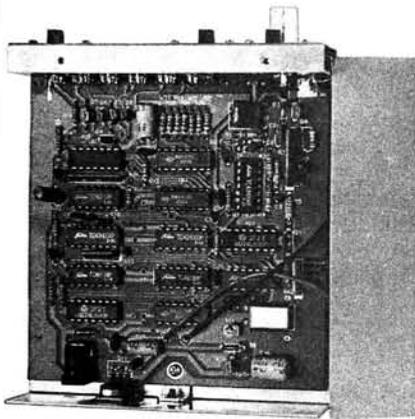
Accuracy, like that of the FC-841, was quite remarkable. The makers specify  $\pm 50$ p.p.m. from 0–40°C, and importers Holdings of Blackburn reckon  $\pm 3$ p.p.m. at room temperature. Checked against an ovened 1MHz standard over 24 hours in a room varying from 15° to 21°C, the readout varied by only 2Hz. The readout is not all that bright, and you'll need to find a shady corner, away from sunlight or a bench lamp.
