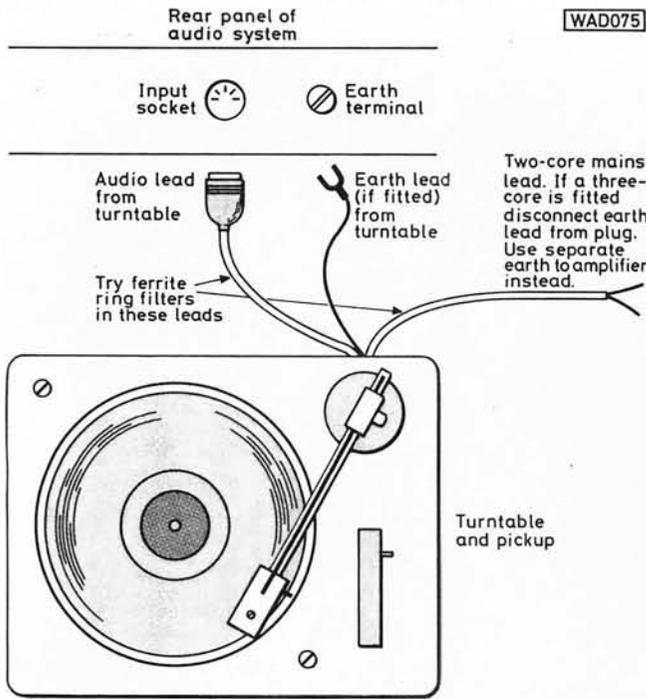
**Fig. 12: Correct method of wiring a turntable to an amplifier to avoid r.f.i. Tape recorders, tuners, etc., should be wired in a similar way**
