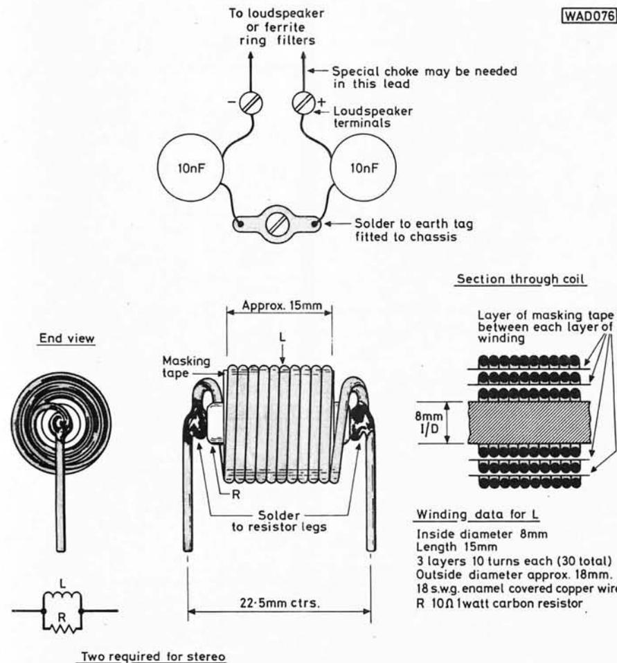
**Fig. 13: Correct methods of filtering loudspeaker leads ▲**
