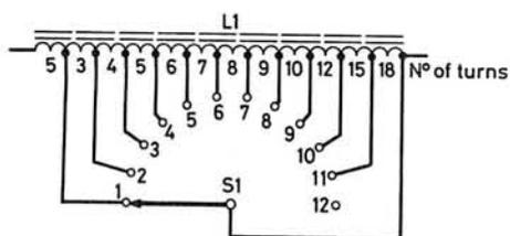
Fig. 2: (above) Details of inductor L1 and its selector switch
