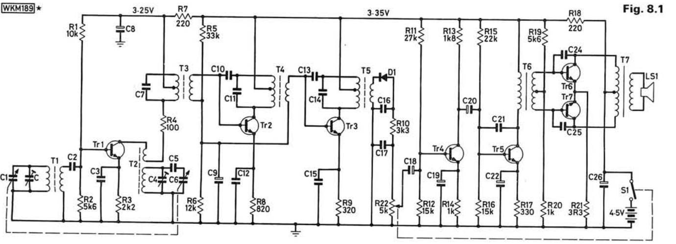
Transistors Tr6 and Tr7 voltages will be identical under no-signal conditions, since there is no resistance in T6 or T7 and the emitters are joined together.
