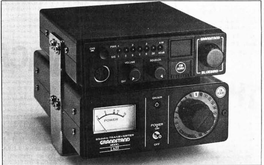
The photograph shows the LA83 transverter below, with a Bluebird 27MHz f.m. transceiver mounted above
