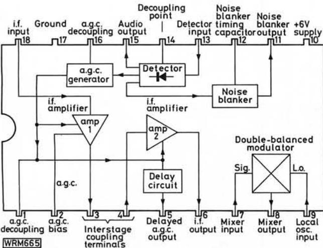
Fig. 1: The connections and internal block diagram of the SL6700C
