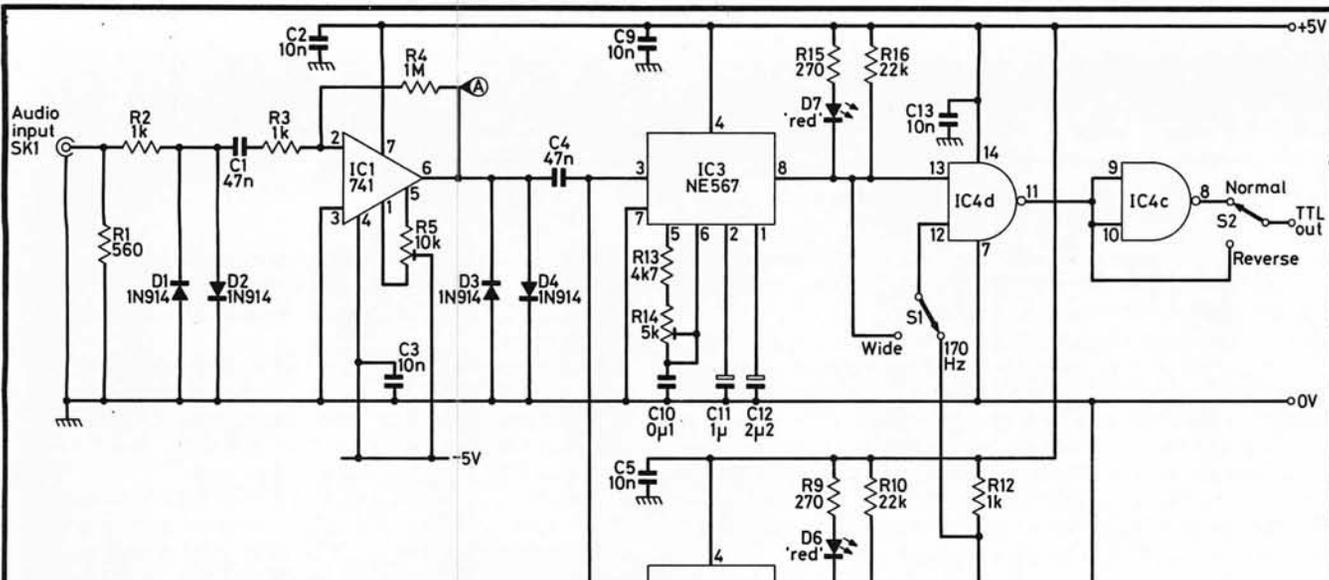
**Fig. 1.2: Circuit diagrams of the receive, transmit (a.f.s.k.) and power supply sections of the terminal unit**
