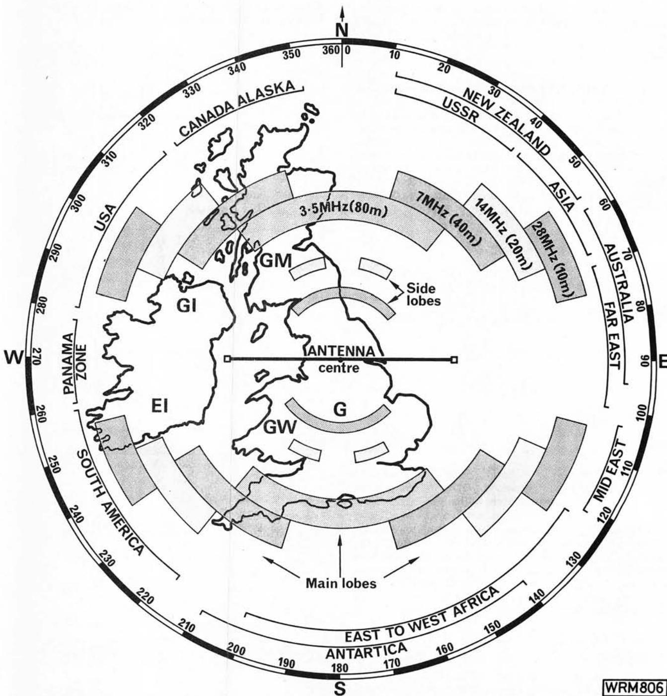
Fig. 5.5: Circle diagram showing approximate coverage with a 40.25m (132 feet) long wire antenna operating as a  $\lambda/2$  on 3.5MHz and for harmonic operation on 7MHz, 14MHz and 28MHz
