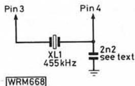
**Fig. 4:** This circuit may be used in Fig. 4 to obtain a sharply peaked selectivity characteristic
