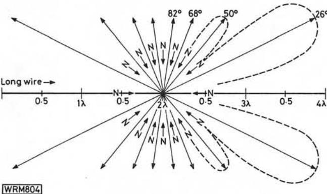
**Fig. 5.3: Formation of radiation pattern of a wire  $4\lambda$  long at operational frequency. Gain in main lobes approximately 3dBd**
