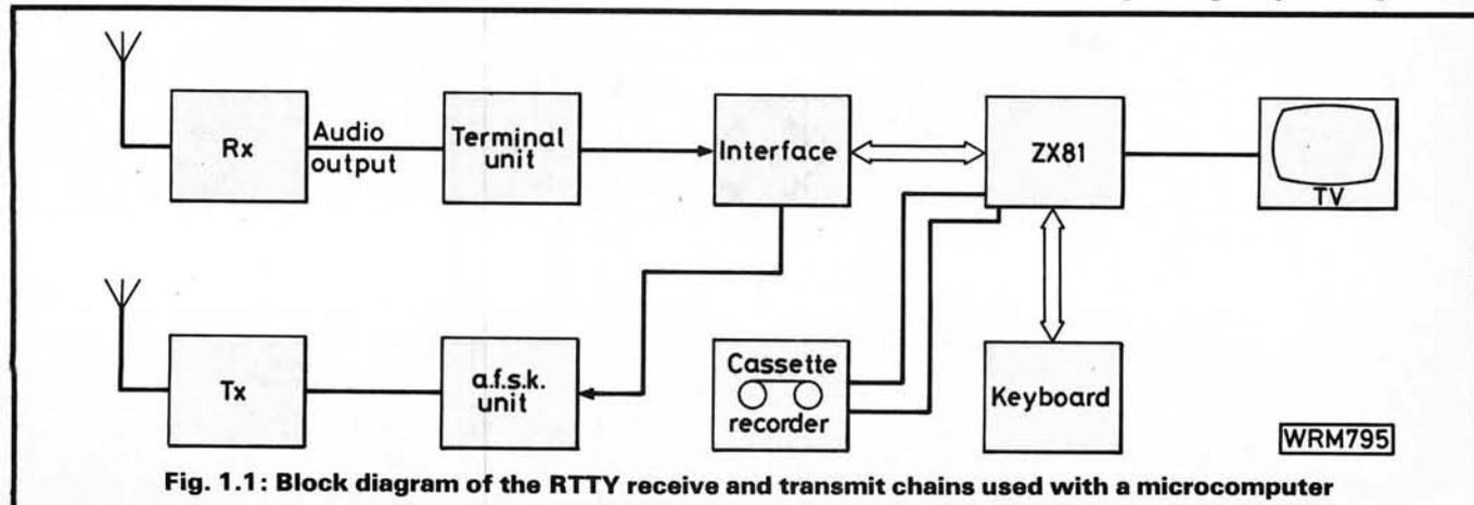
Fig. 1.1: Block diagram of the RTTY receive and transmit chains used with a microcomputer
