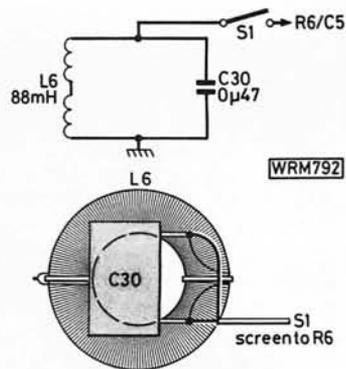
**Fig. 2.4: The circuit and construction of a suitable audio filter**
