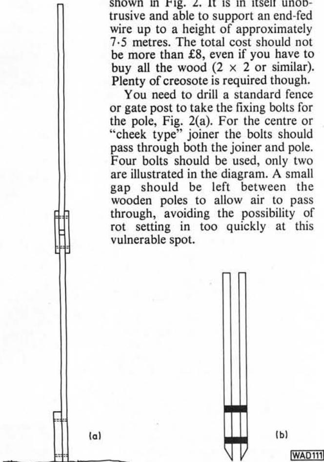
Fig. 2: Simple wooden mast and base
