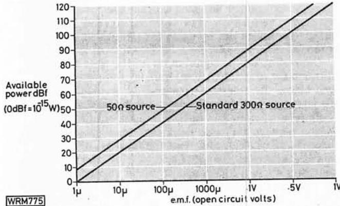
**Fig. 4.4: The relationship between e.m.f. and available power in dBf into a 300Ω standard impedance, with 50Ω plot shown for comparison. Note that for a given e.m.f. the power into a 50Ω impedance is 7.78dB (×6) more than for 300Ω. 1μV into 50Ω = 6.99dBf or -0.79dBf into 300Ω**
