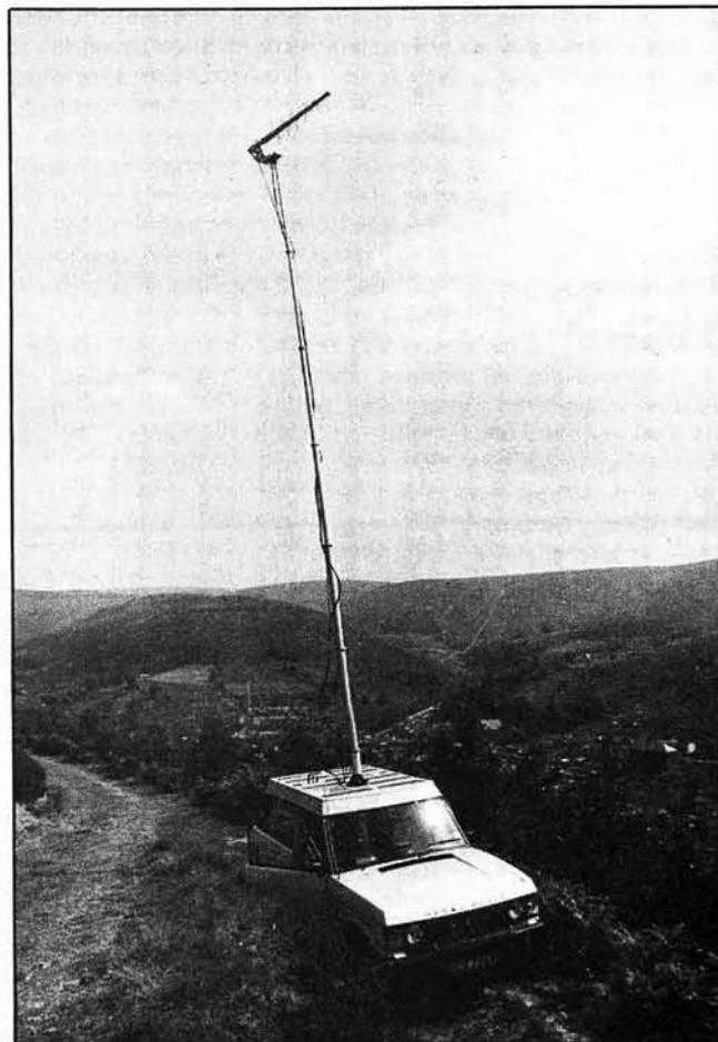
**Fig. 1: The Clark Masts Ltd. 10 metre mast being used during field strength tests**
