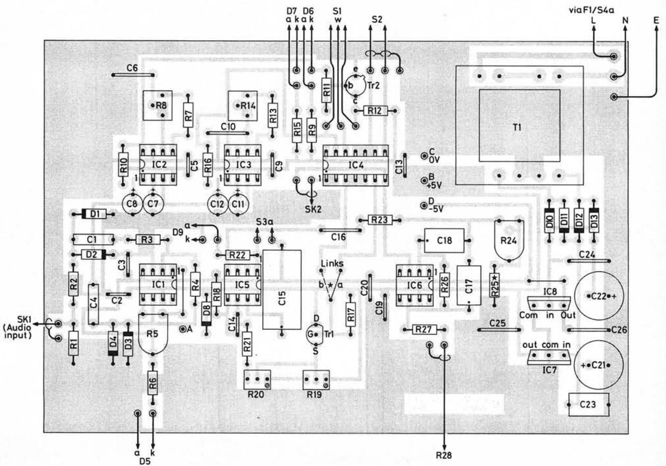
Fig. 1.3: The full-size copper track pattern for the p.c.b. together with the component placement drawing
