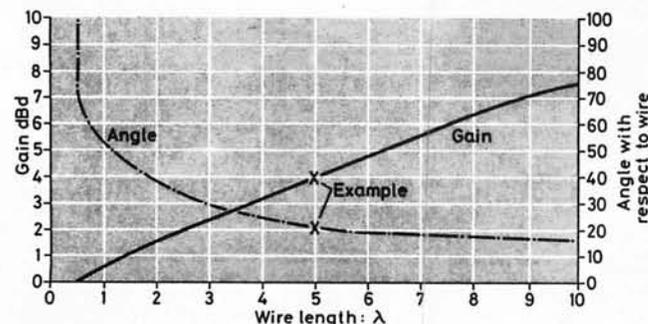
Fig. 5.1: Gain in main lobes relative to length of wire in wavelengths. Example gives gain in main lobes of 4dBd for wire  $5\lambda$  long. The angle of main lobes to wire is approximately 20 degrees
