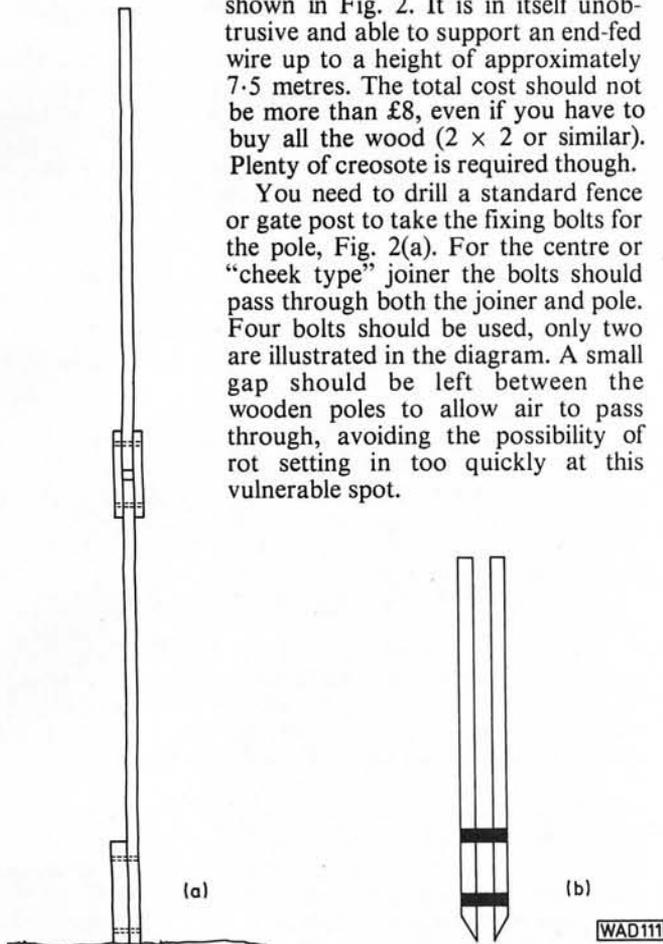
Fig. 2: Simple wooden mast and base
