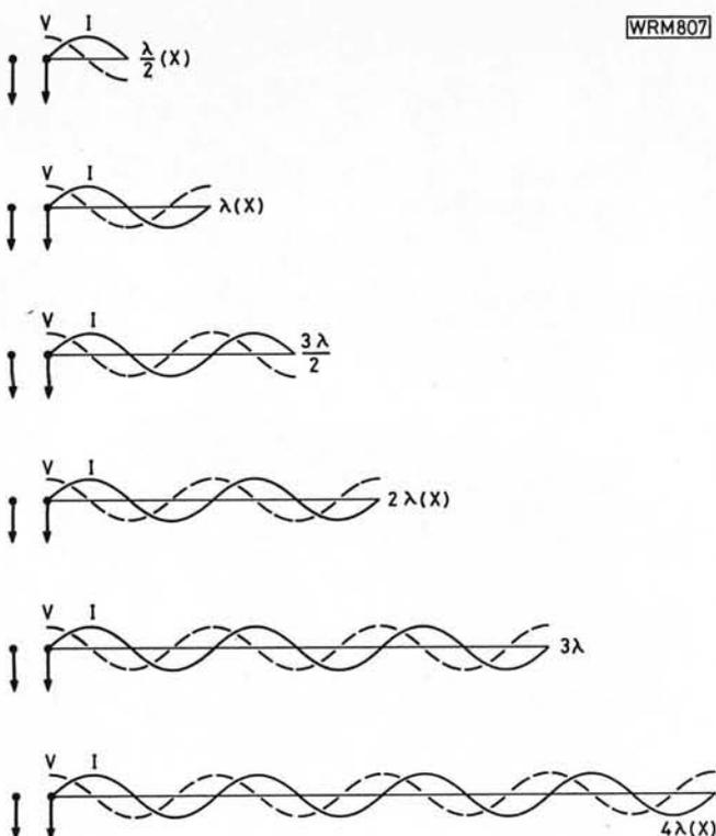
Fig. 5.6: Current and voltage distribution on long wire antennas of "N" number of half or full wavelengths when wire is end fed via a tuned feeder system (see text). Those marked X are directly harmonically related
