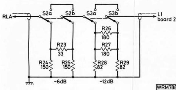
**Fig. 2.3: The circuit and constructional details of the switched input attenuator**
