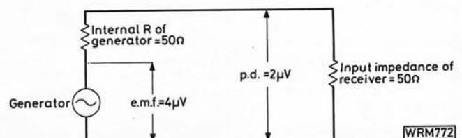
Fig. 4.1: The generator output is divided between the internal resistance and the external load
