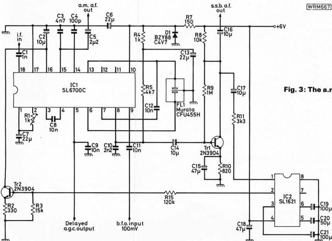
Fig. 3: The a.m./s.s.b./c.w. i.f. strip
