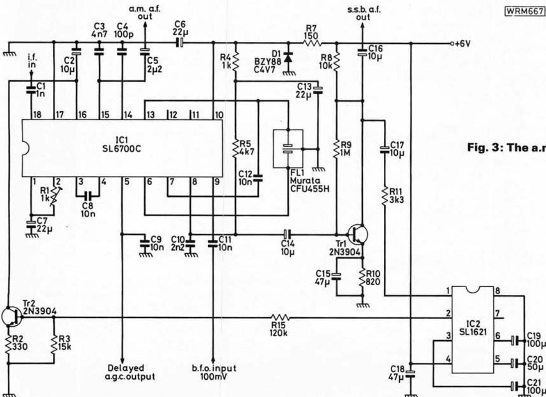
Fig. 3: The a.m./s.s.b./c.w. i.f. strip
