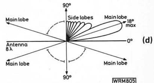
**Fig. 5.4: Radiation patterns related to long wire antennas of (a)  $\lambda/2$ , (b)  $\lambda$ , (c)  $3\lambda/2$  and (d)  $8\lambda$**
