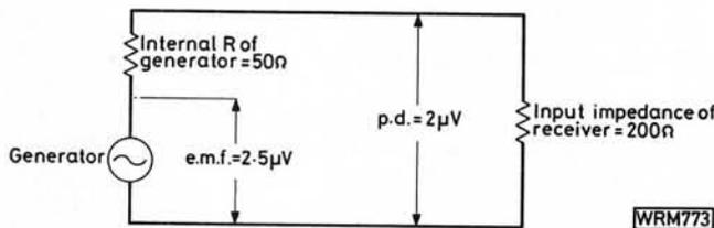
**Fig. 4.2:** When the impedances are not equal the ratio between e.m.f. and p.d. will vary depending on the value of the load impedance
