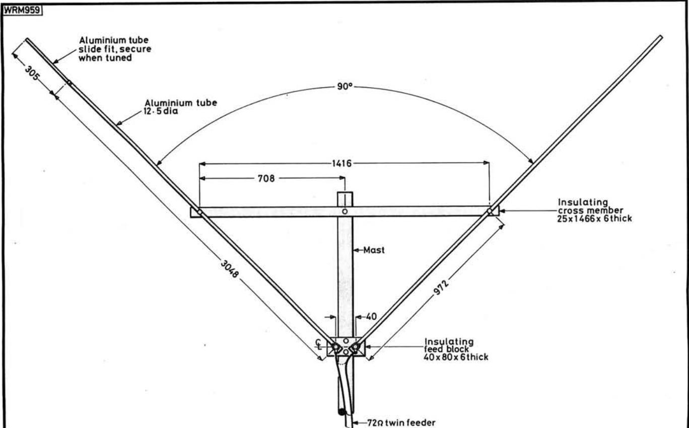
**Fig. 1: Constructional details of the Vertical V antenna for 21MHz. Both radiating elements are provided with length adjustment and for best results a 1:1 balun should be fitted at the feedpoint when using 50 ohm coaxial cable. Note that this drawing is not to scale**
