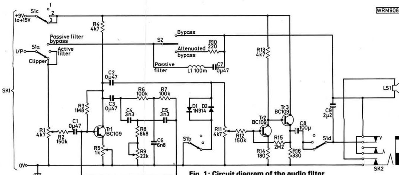
Fig. 1: Circuit diagram of the audio filter
