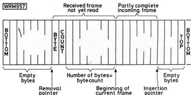
**Fig. 2.6: A typical data buffer, showing pointers, and order of placement data. The buffer shown is the packet input buffer, and is similar to the other buffers**
