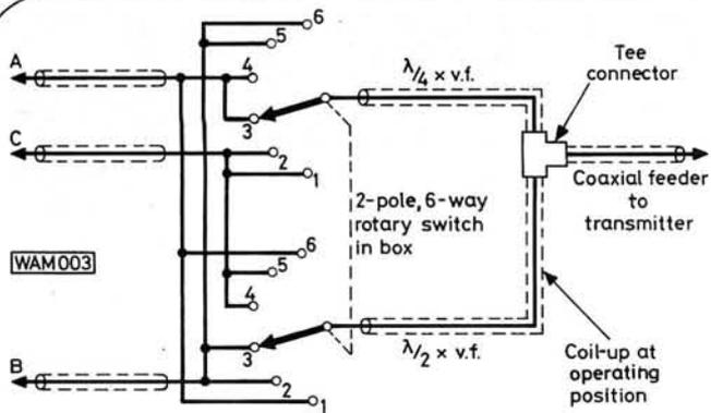
**Fig. 3: Direction switching arrangements. Allowance must be made for cable velocity factor (v.f.)**
