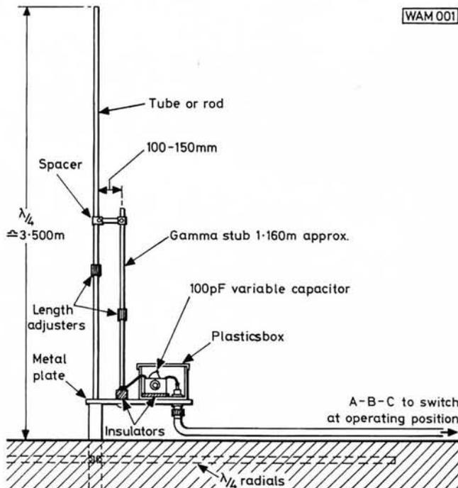
**Fig. 1: Constructional details of the  $\lambda/4$  gamma matched 21MHz radiating elements. The plastics box used by the author was a 2 litre ice cream container**
