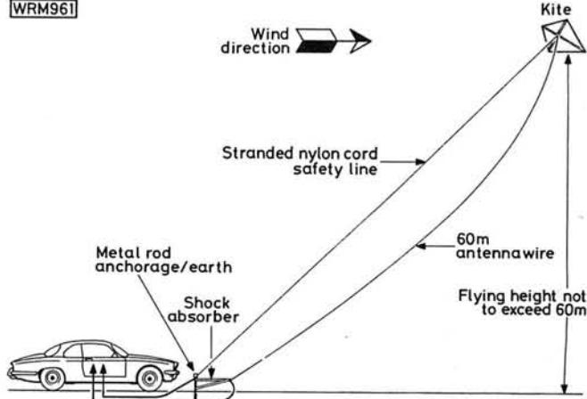
**Fig. 1: The basic layout of the Kite supported antenna system discussed in the text**
