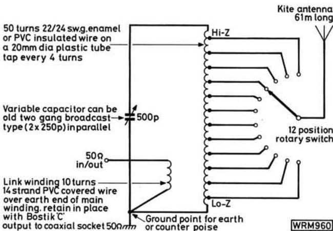
**Fig. 2: Circuit details of the a.t.u. used by the author for operation on the 1.8MHz band**
