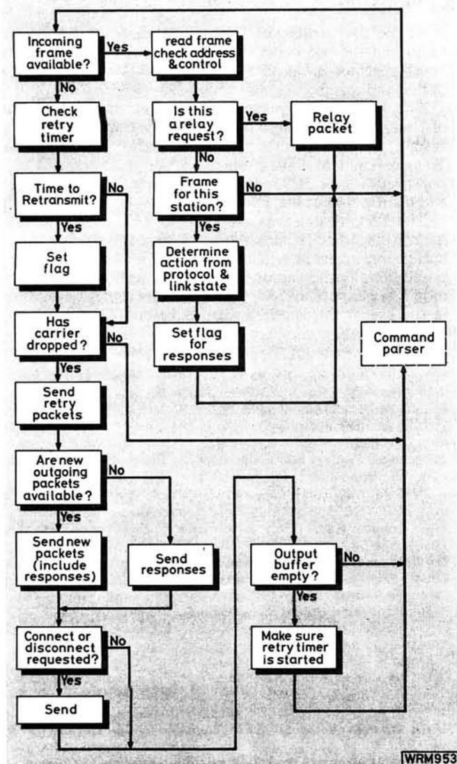
Fig. 2.5: Flowchart for operation of the packet protocol HLR routine
