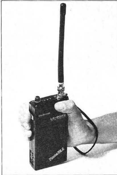
The 50Ω flexible antenna plugs into a BNC socket on the top panel where the volume/off switch, squelch and frequency selector switches are also located. Frequency selection is achieved with "thumb-wheel" switches and depending on the size of your fingers can be easy or difficult to operate.
