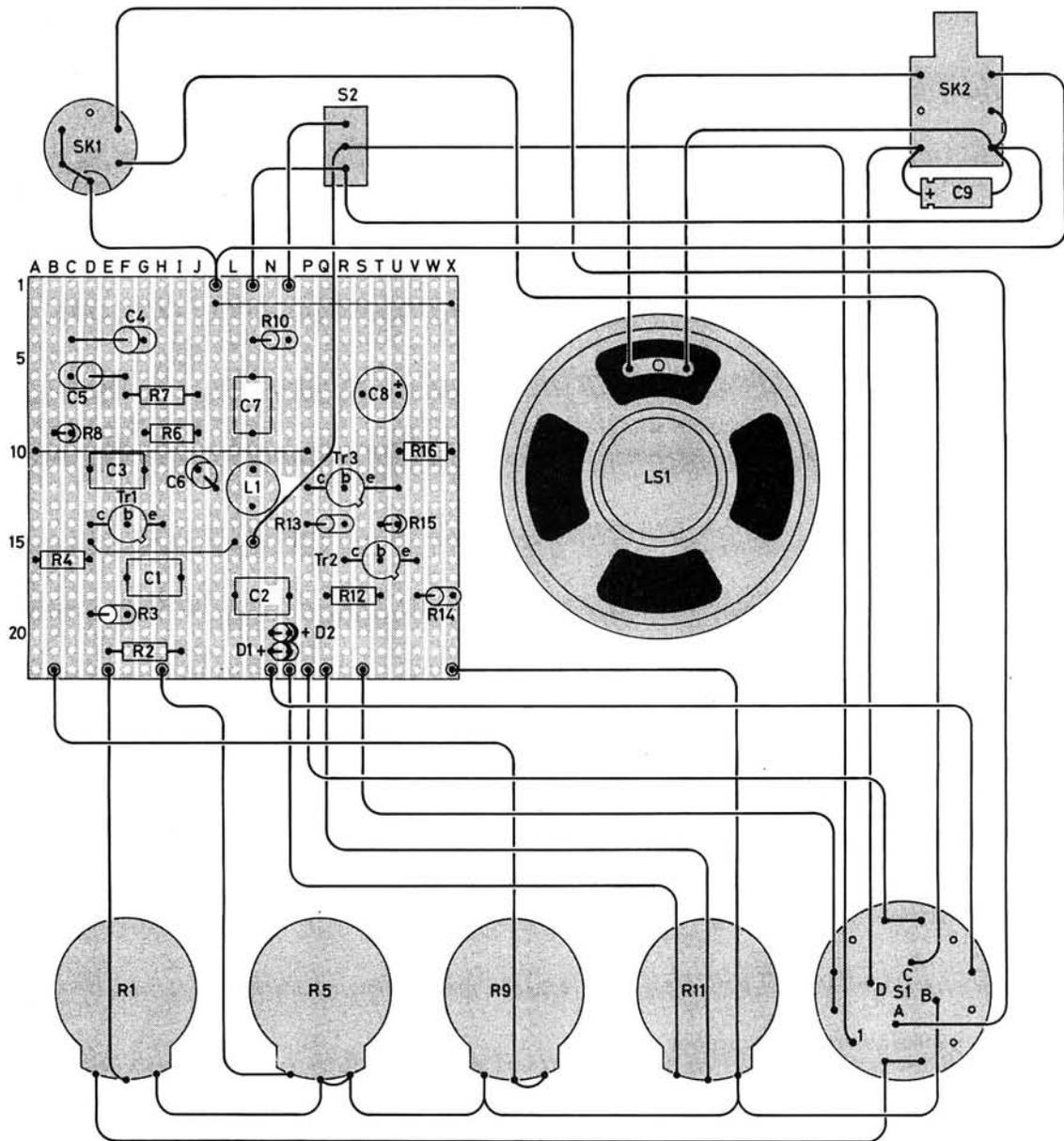
**Fig. 2: Component placement and interconnection details. Veroboard track breaks occur at M7, M12, O12, E19 and N18**
