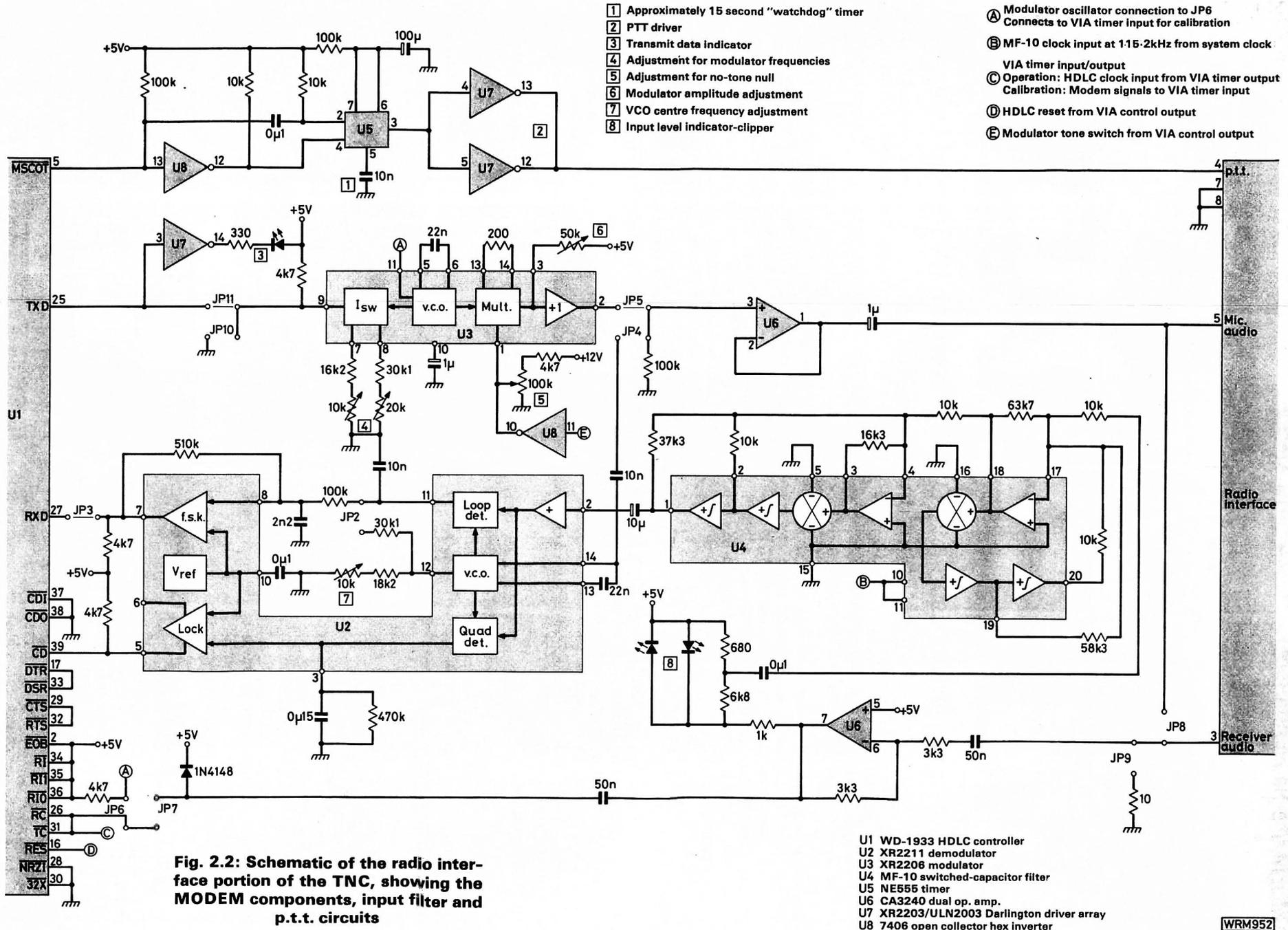
**Fig. 2.2: Schematic of the radio interface portion of the TNC, showing the MODEM components, input filter and p.t.t. circuits**
