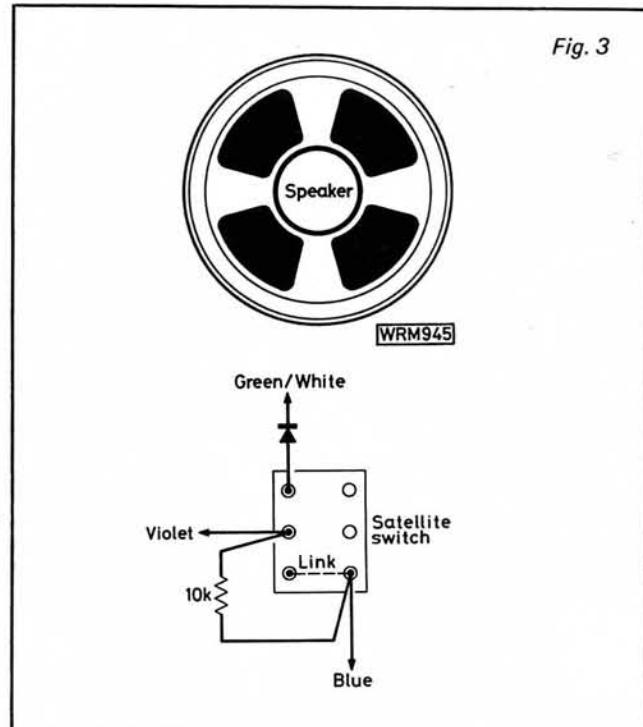
Next, unsolder the green/white wire from the topmost pin and solder a diode (1N914) to that pin. Then solder the green/white wire to the other end of this new diode. Now, whenever you are listening to a repeater, pushing the toneburst button on the microphone will cause the receiver to switch to the input.
