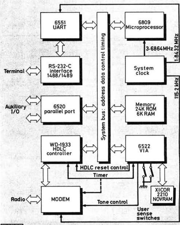
Fig. 2.1: Block diagram of the TAPR Beta TNC, showing system architecture
