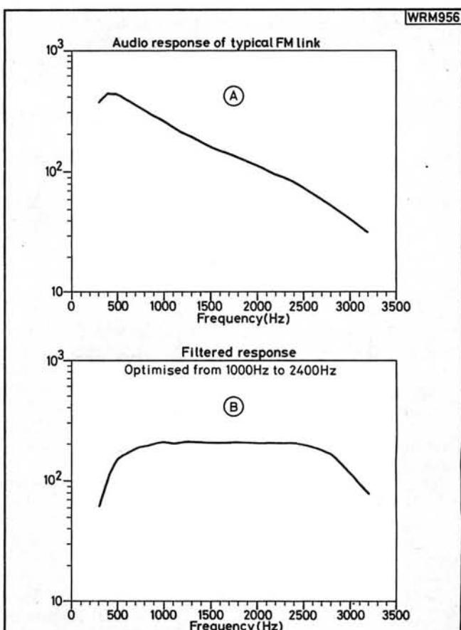
Fig. 2.4: (a) Measured frequency response using a pair of 144MHz f.m. transceivers. (b) The same frequency response after filtering. The filter design was optimised for the range 1000Hz to 2400Hz
