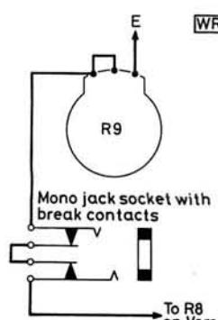
**Fig. 4: The modification needed to provide a Morse practice facility. The jack socket which should be a mono type, can be located on the rear panel of the filter housing**
