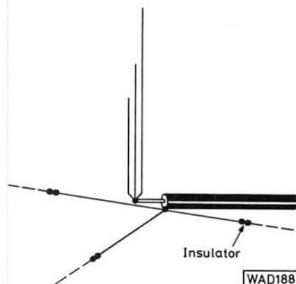
**Fig. 2:** If at all possible horizontal wires should be added as shown here, all soldered together and to the outer shield of the coaxial cable. The wires are the same length as those in the vertical elements, one for each band, but two or more per band are highly desirable
