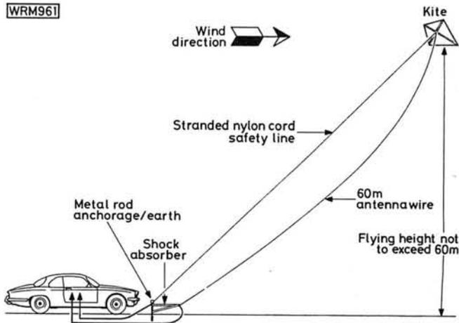
Fig. 1: The basic layout of the Kite supported antenna system discussed in the text
