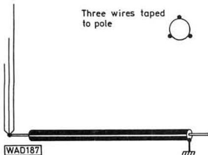
**Fig. 1:** Three pvc-insulated wires, 2-6m, 3-6m and 5-3m long respectively, are taped at intervals to a vertical wooden pole or bamboo cane. The bottom ends of the wires are soldered together to the inner conductor of the coaxial cable. The cable end should be sealed against the ingress of moisture. This antenna will cover the 28, 21 and 14MHz bands
