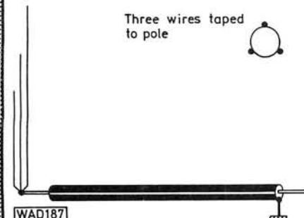
**Fig. 1: Three pvc-insulated wires, 2.6m, 3.6m and 5.3m long respectively, are taped at intervals to a vertical wooden pole or bamboo cane. The bottom ends of the wires are soldered together to the inner conductor of the coaxial cable. The cable end should be sealed against the ingress of moisture. This antenna will cover the 28, 21 and 14MHz bands**
