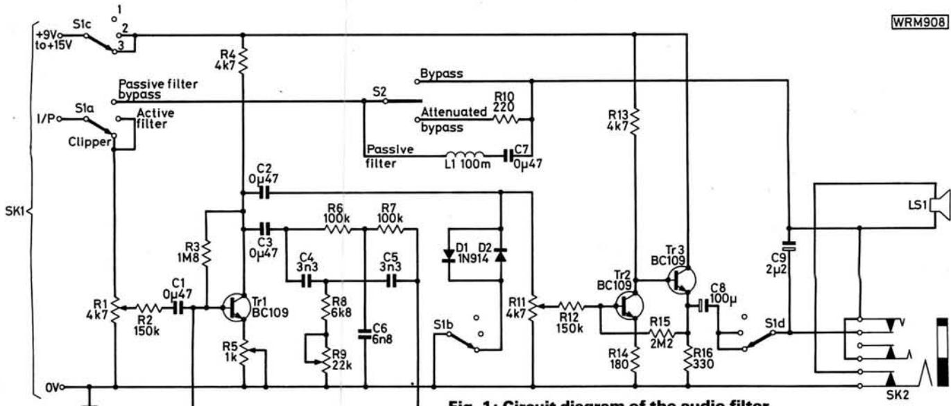
Fig. 1: Circuit diagram of the audio filter
