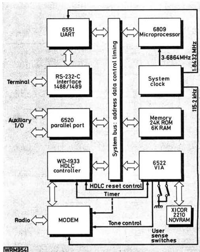
**Fig. 2.1: Block diagram of the TAPR Beta TNC, showing system architecture**
