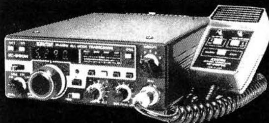
The recently introduced IC-290H has proved so popular that we have decided to concentrate on this (25W) model 2m multimode. With its bright green display, 5 memories, scan facilities on either memories or the whole band, tone-call button on the microphone and instant listen input for repeaters, this little box really is a beauty. The 70cm version, the IC-490E has similar features (although the output is only 10W in this case).
