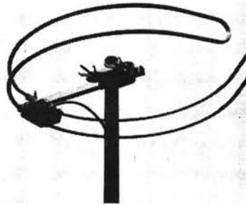
Gain is claimed to be between -2 and -4dBd and the folded element is
