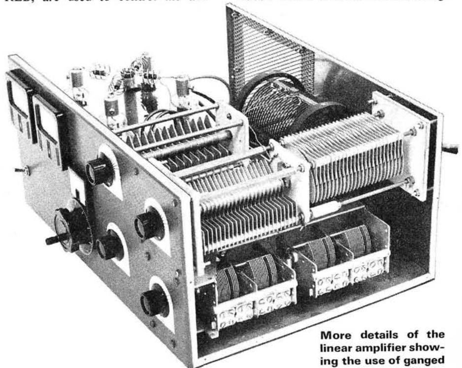
**More details of the linear amplifier showing the use of ganged variable capacitors**
