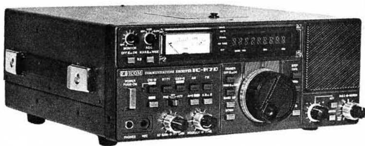
Icom's first h.f. receiver, the IC-R70 uses microprocessor technology to provide the alternatives of a general coverage receiver with 1MHz bands or an amateur bands receiver with rapid band selection.
