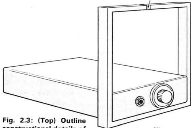
Fig. 2.3: (Top) Outline constructional details of the ferrite rod antenna. (Above) Frame antenna details
