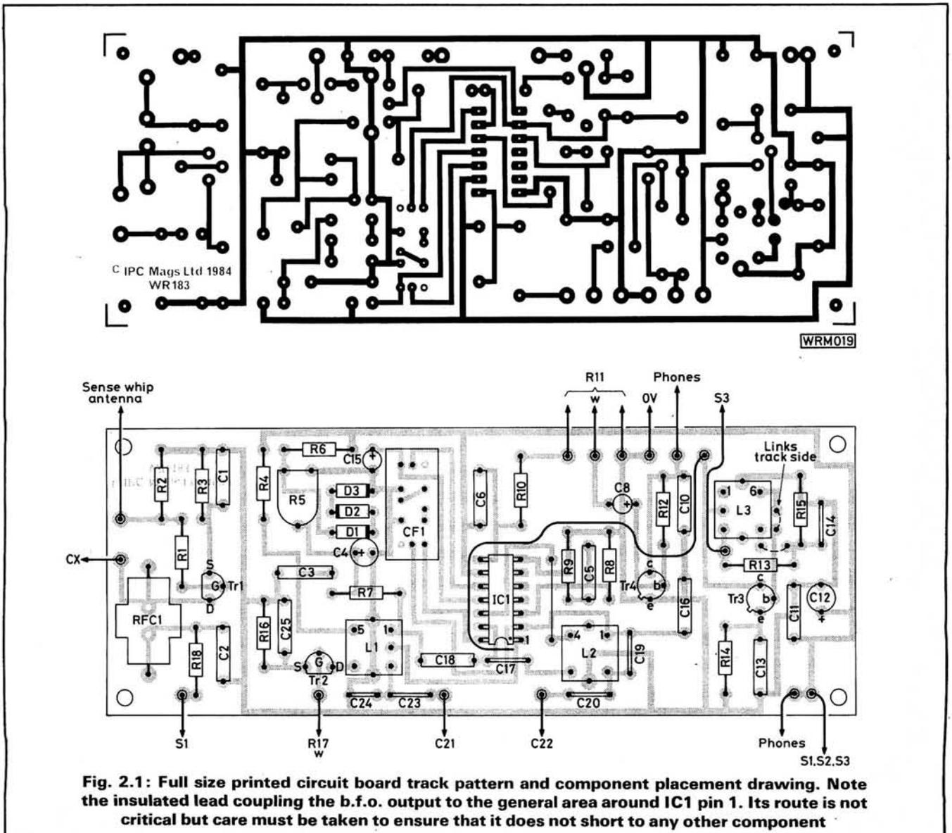
Fig. 2.1: Full size printed circuit board track pattern and component placement drawing. Note the insulated lead coupling the b.f.o. output to the general area around IC1 pin 1. Its route is not critical but care must be taken to ensure that it does not short to any other component
