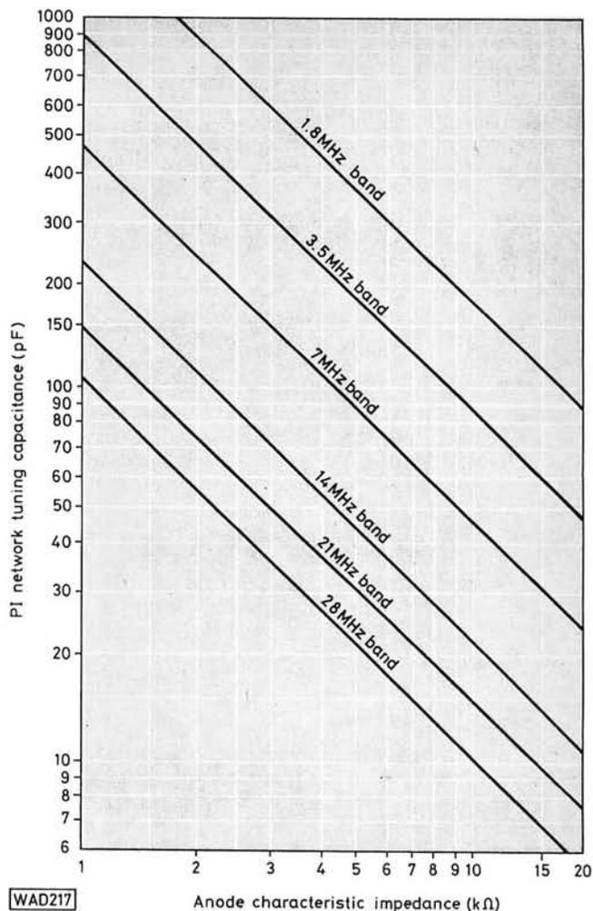
Fig. 1.2: Graph for determining the pi network tuning capacitance for the different amateur bands
