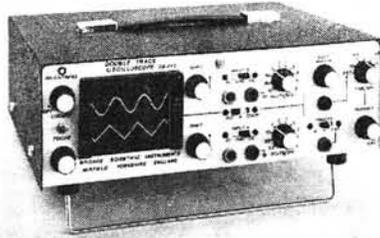
good trace readability on the 60 x 50mm display screen on which a calibrated graticule is superimposed. Considerable time savings in use may be achieved, utilising the trace location button which returns overscanned traces to the screen regardless of the setting of other operating controls and the auto brightline triggering system.
