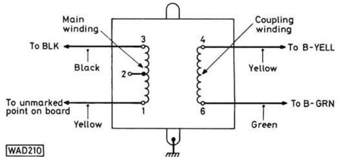
Fig. 3: Medium wave r.f. transformer connections
