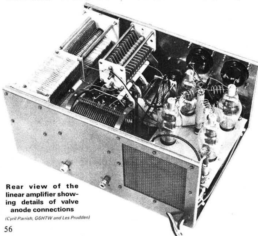
**Rear view of the linear amplifier showing details of valve anode connections**
