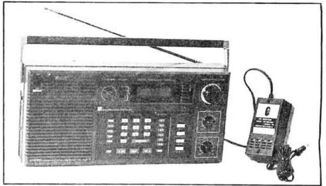
The Uniden CR-2021 is a fully synthesised receiver covering the long, medium and short-wave bands, plus the v.h.f. f.m. broadcast band (Band II).
