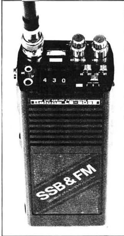
squelch; noise blanker; mode switch (f.m., u.s.b. and l.s.b.); external microphone and speaker; RIT and VXO, S-meter/battery meter; and thumbwheel switches. The meter and thumbwheel switches may be illuminated simultaneously, by an l.e.d. lamp, switched from the side panel.
