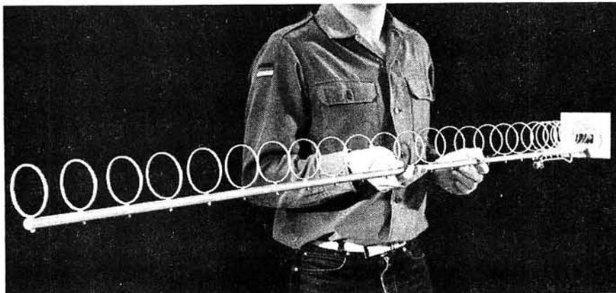
in both planes. The bandwidth should accommodate operations on the OSCAR 10 mode L uplink and 1.3GHz ATV. The 1296-46QL has a four metre boom (17λ) and a gain of 22dBi, with correspondingly reduced beamwidth.
