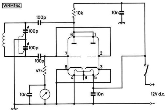
Fig. 1: Circuit of grid dip oscillator using a 12V d.c. supply for both valve heater and h.t. Other valve types which may be used, with similar pin connections, are the ECC81 and ECC83. Four or five plug-in coils may be used to cover 1.8 to 30MHz although the circuit will work into the v.h.f. range. Fixed capacitors should be silver mica or similar. The meter can be a 50 or 100 $\mu$ A f.s.d. type
