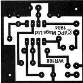
Fig. 2: Component layout and p.c.b. track pattern shown full size. The version shown uses an electret insert mounted in the enclosure wall within a rubber grommet. An appropriate socket/captive plug would be fitted in place of the insert if used with the original transceiver hand-held microphone
