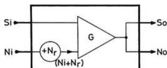
▲ Fig. 2: Hypothetical receiver showing noise adder and noiseless amplifier.
