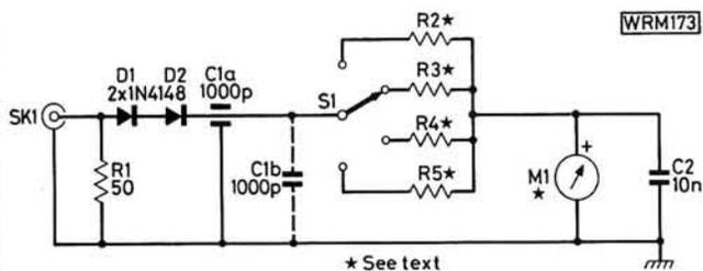
**Fig. 1: Circuit diagram of the r.f. power meter. Values of R2-5 (1-50W) are given in Table 1**
