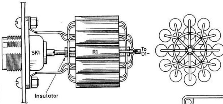
**Fig. 4: General layout details of the r.f. power meter. For h.f. band use only the screen and feedthrough capacitor C1a are not essential, however greater overall accuracy will be achieved by the use of these items which are incorporated to reduce the effects of induced currents/stray r.f. rectification within the d.c. meter assembly**
