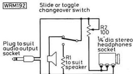
Fig. 1: Simple circuit for a unit providing rapid changeover from speaker to headphones when VR1 is adjusted for comfortable listening level
