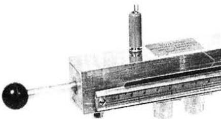
quency. A quarter wave line is formed by an adjustable plunger, running parallel to a millimetre rule used for the measurement. Applied r.f. is coupled into the cavity via a link probe across BNC or N-type sockets, allowing termination into a suitably rated load. A 3.5mm socket/jackplug fitted with
