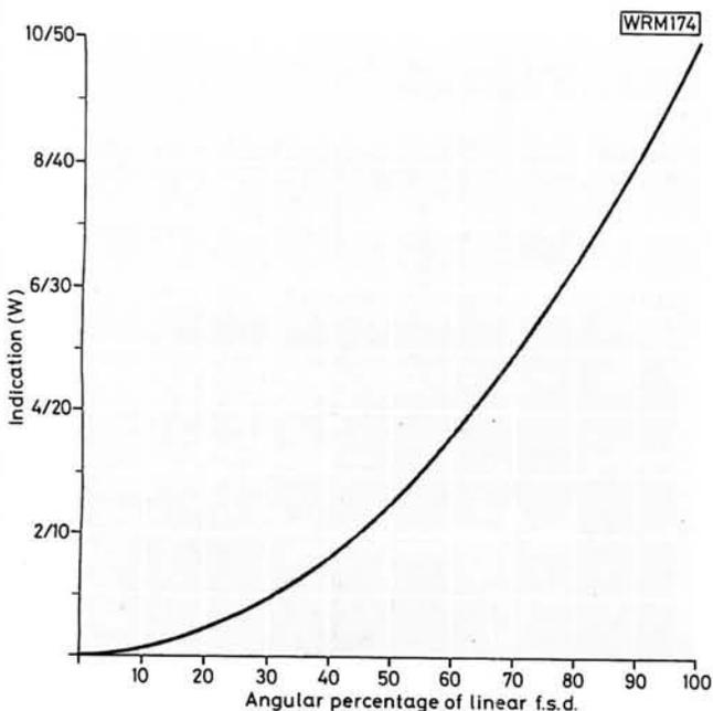
Fig. 2: Graph of indicated power against linear scale meter deflection to allow meter calibration
