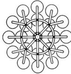
**Fig. 3: The constructional arrangement of the composite load resistor R1. For reliable operation the coaxial layout shown must be adopted, all lead lengths being kept to the minimum. The centre pin extension of SK1 is fitted with a sleeve insulator to avoid any possibility of shorting against the "earthy" side of R1**
