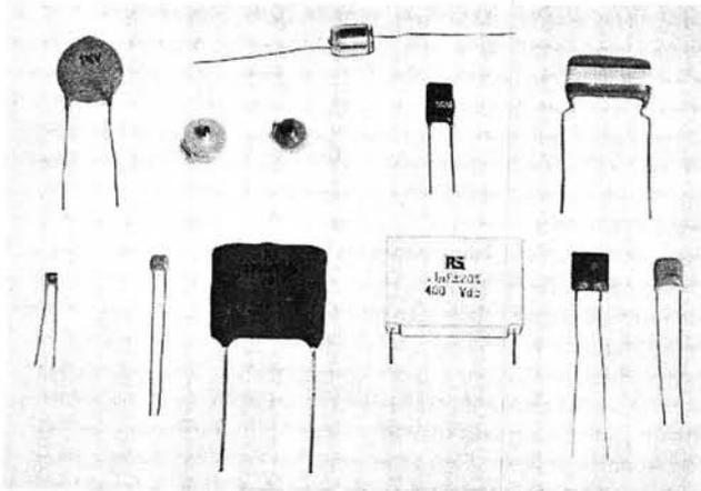
Capacitors should be chosen with a working voltage well in excess of what they will have to withstand
