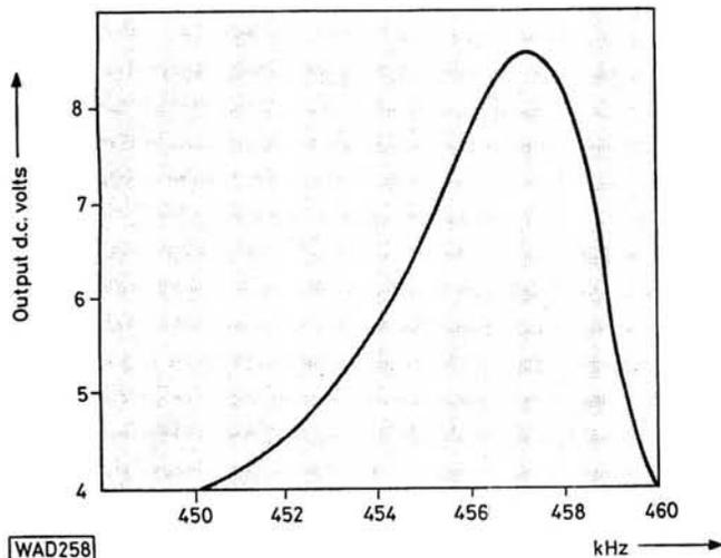
**Fig. 7: Response of the TBA120 with 8008 ceramic resonator**
