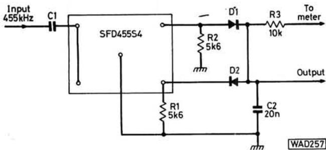
**Fig. 6: Ceramic ratio detector using the SFD 455S4 (Toko/Yaesu FT 227)**
