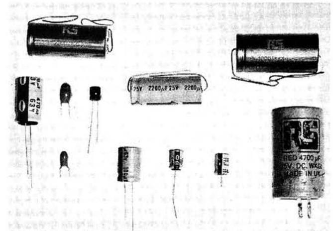
**Electrolytic capacitors usually have their capacitance value and working voltage printed on the body of the component**
