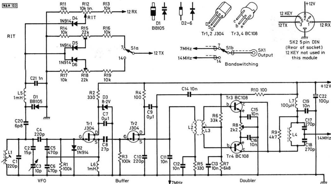
Fig. 2.1: Circuit diagram of Module 2, the VFO/Doubler
