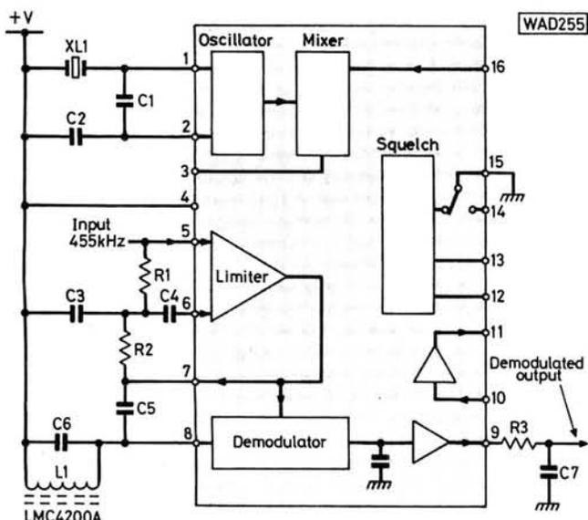
**Fig. 4: The MC3357/MP5071 demodulator system. Oscillator and mixer circuits are available to convert other i.f. frequencies to 455kHz**
