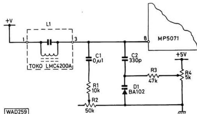
**Fig. 8: A tunable 455kHz demodulator using the MP5071**
