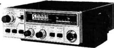
144 MHz, 12VDC FM Transceiver. 25W/5W Hi/Lo (both adjustable). Compact 2 1/2" x 6 1/2" x 7 1/2". 12 1/2 KHz steps (100 KHz fast QSY). Amber LCD 'Sunlight View'. Side Lit Display; 100's of Hz + channel number. Sensitivity <math>0.2\mu V</math> for 12 dB SINAD. Single knob frequency control "Dial". Endless or non endless dial options/RIT; 1 KHz steps, V.F.O. + memory. Two 5 slot memories A, B, A + B, A x B.
