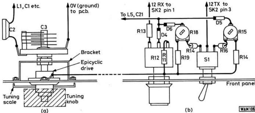
**Fig. 2.4: (a) Slow motion tuning drive assembly. (b) Wiring of the RIT and BANDSWITCH controls**
