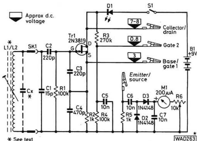
Fig. 1: Circuit diagram of the simple r.f. transistor tester
