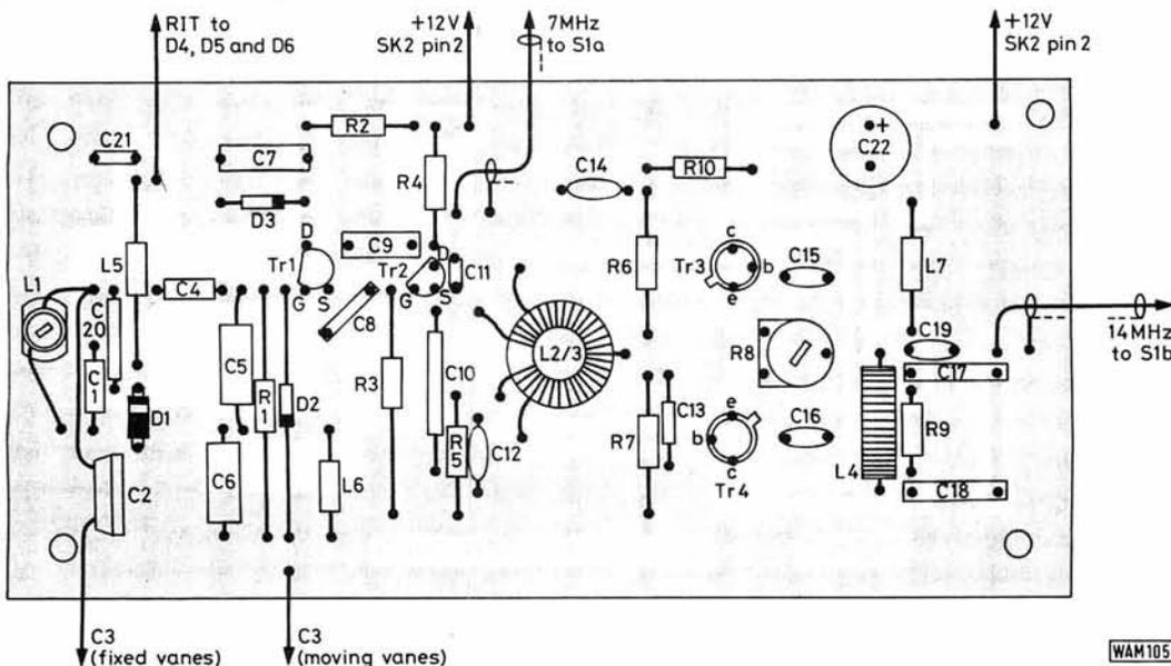
Fig. 2.3: Full size p.c.b. track pattern and component layout for Module 2, the VFO/Doubler
