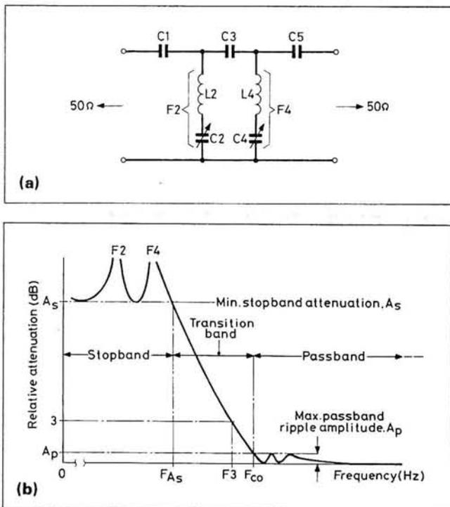
**Fig. 5.2: Circuit diagram and attenuation response of 5-branch Cauer highpass filter. Tune  $C2/L2$  to  $F2$ ,  $C4/L4$  to  $F4$**
