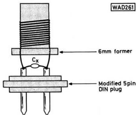
Fig. 3: (Above) Details of the plug-in coils. Fig. 4: (Below) Suggested layout of the unit in a plastics box
