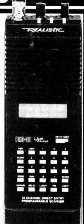
**Realistic PRO-30.** Scan up to 16 of your favourite channels continuously, or search a selected frequency range for new or unpublished channels. Scan and Search in two speeds. Two-second Scan Delay, selectable for each channel prevents missed replies. Has jacks for external antenna and earphones. Requires six "AA" batteries or mains or DC adapter. Memory backup requires four silver-oxide batteries. 20-9131
