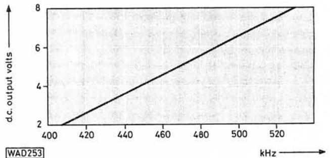
Fig. 2: Linear operating range of the 4046 demodulator
