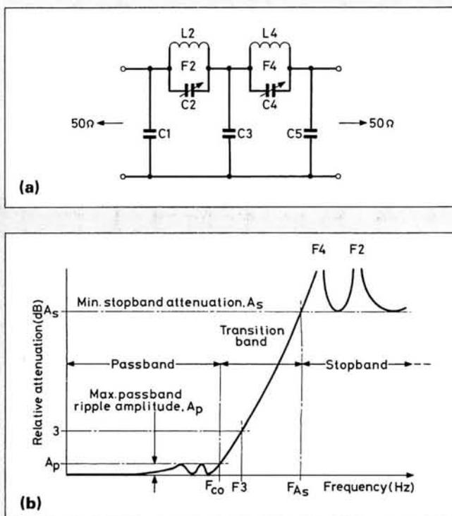
**Fig. 5.1: Circuit diagram and attenuation response of 5-branch Cauer lowpass filter. Tune C2/L2 to F2, C4/L4 to F4**
