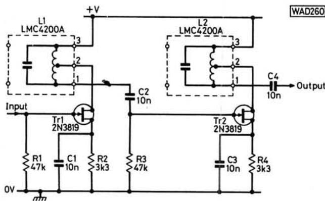
Fig. 9: Circuit diagram of a 455kHz i.f. amplifier
