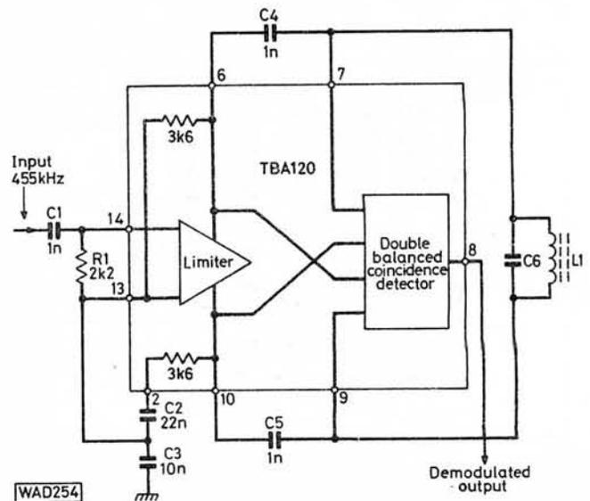
Fig. 3: The TBA120 demodulator
