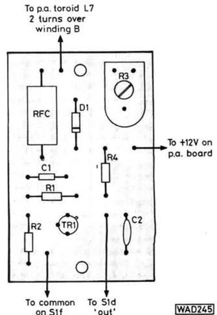
to simulate p.a. d.c. input which I have called an **r.f. Meter Monitor**. It is a variation of another G3RJV circuit (1) which consists of a diode detector and a single transistor d.c. amplifier. The meter did not give a full scale deflection without this extra amplification.
