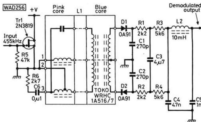
**Fig. 5: Discrete component ratio detector**
