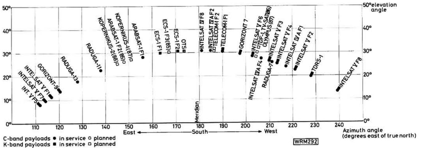
Fig. 2.2: The geostationary orbit as viewed from London
