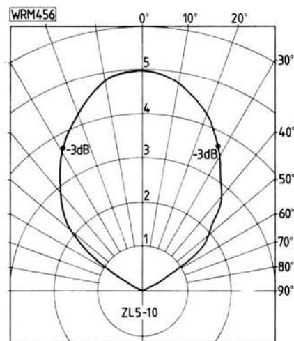
Fig. 4.3: Horizontal radiation pattern of the ZL5-10
