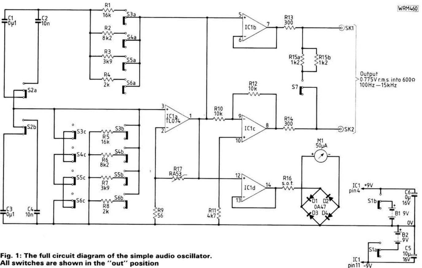
Fig. 1: The full circuit diagram of the simple audio oscillator. All switches are shown in the "out" position
