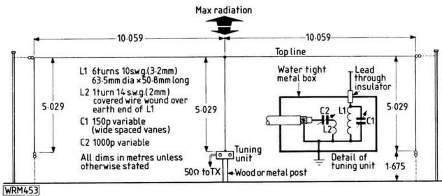
Fig. 4.4: Details of the 14MHz Bobtail antenna
