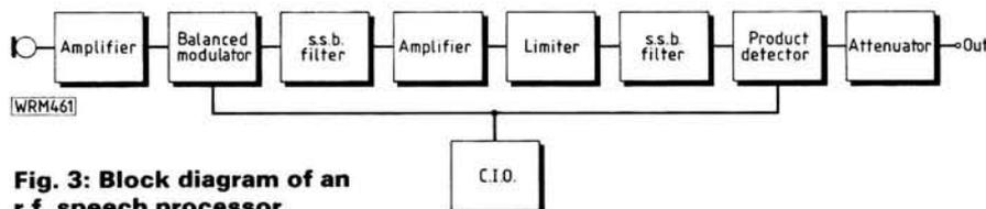
Fig. 3: Block diagram of an r.f. speech processor
