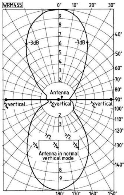
Fig. 4.5: Radiation pattern of the Bobtail broadside antenna
