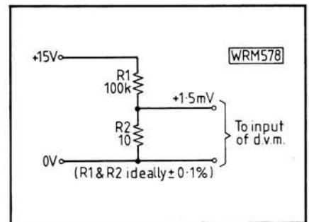
Fig. 1.6: Calibration circuit
