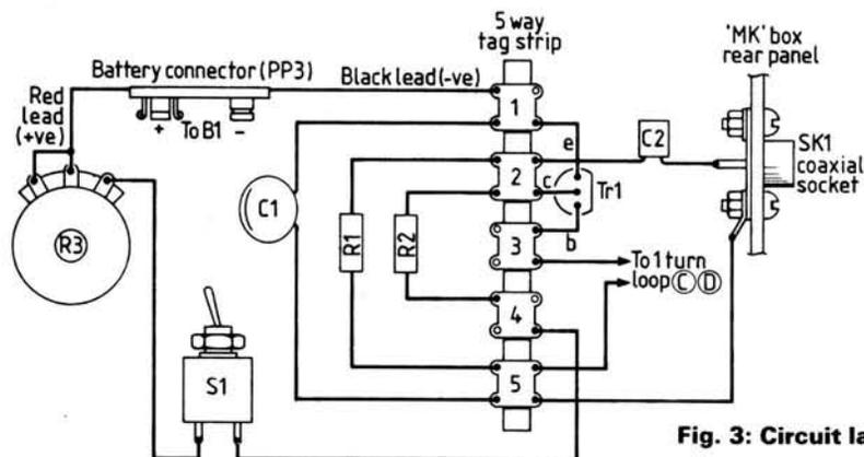
Fig. 3: Circuit layout
