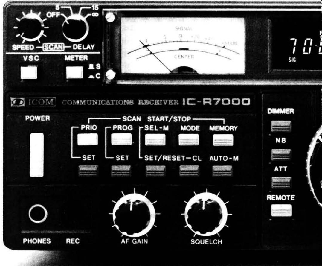
ICOM introduces the IC-R7000, advanced technology, continuous coverage communications receiver. It covers Aircraft, Marine, F.M, Broadcast, Amateur Radio, Television and Weather Satellite bands. The IC-R7000 incorporates FM wide/FM narrow, A.M., upper and lower SSB modes of operation with six tuning speeds: - 0.1, 1.0, 5, 10, 12.5, 25KHz. Frequency coverage 25-1000MHz and 1025-2000MHz (25-1000MHz and 1260-1300MHz guaranteed specification).
