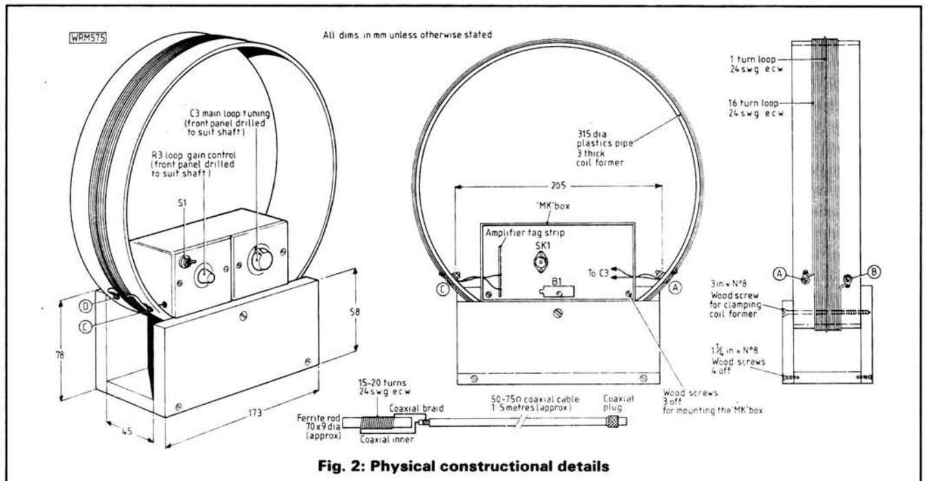
Fig. 2: Physical constructional details
