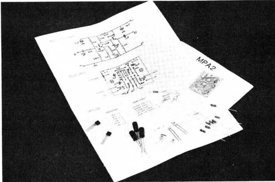
This month's kit is a very useful little microphone pre-amp from Wood & Douglas, the MPA-2. This is an improved version of their earlier and popular MPA1, the main difference being the addition of a buffered output. The unit's prime function is fairly obviously to boost the output of a low output microphone to a level suitable for feeding into a transmitter, as Elaine Richards G4LFM finds out.
