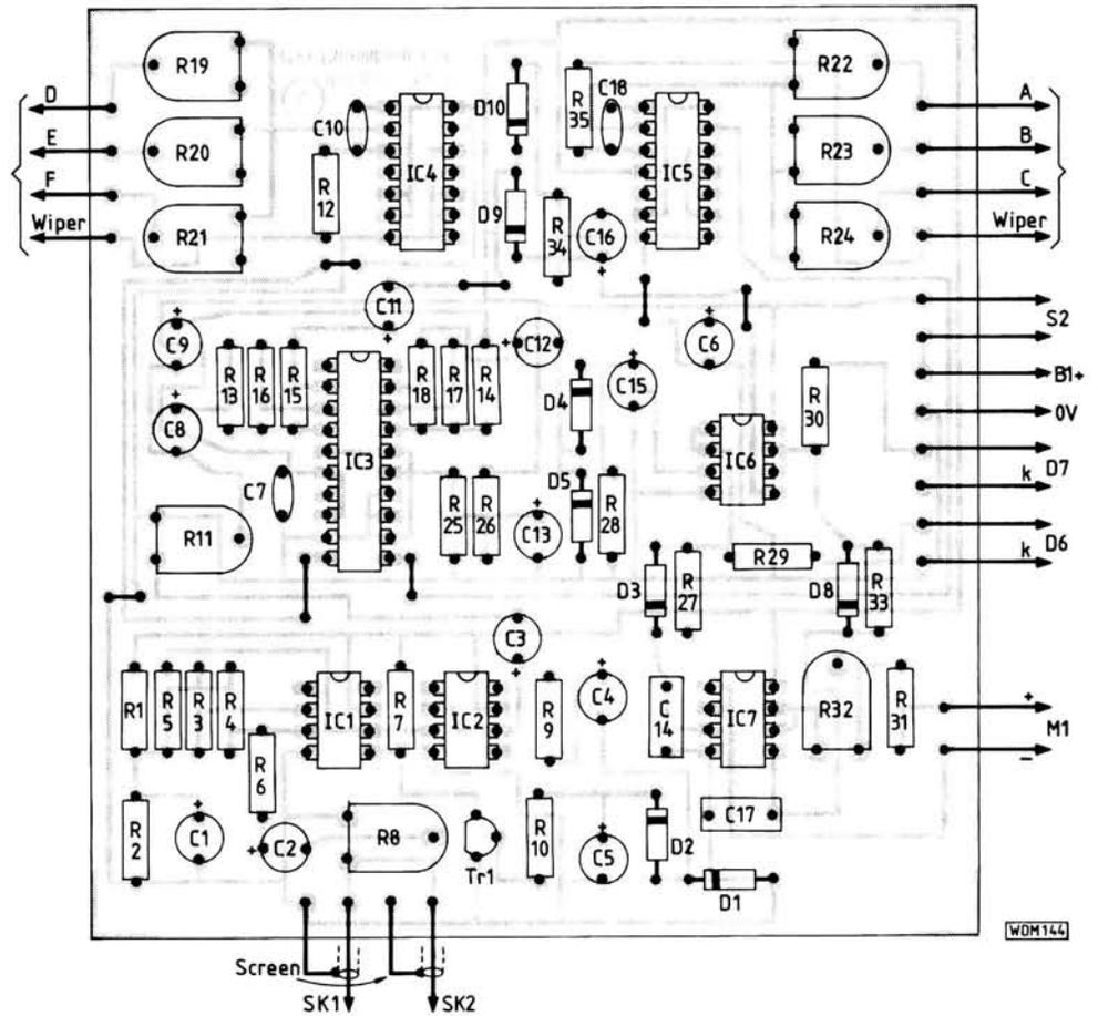
**Fig. 6: Single-sided p.c.b. track pattern and component overlay, shown full size**
