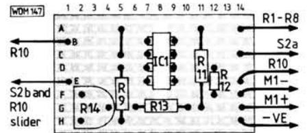
The Veroboard layout of the multimeter
