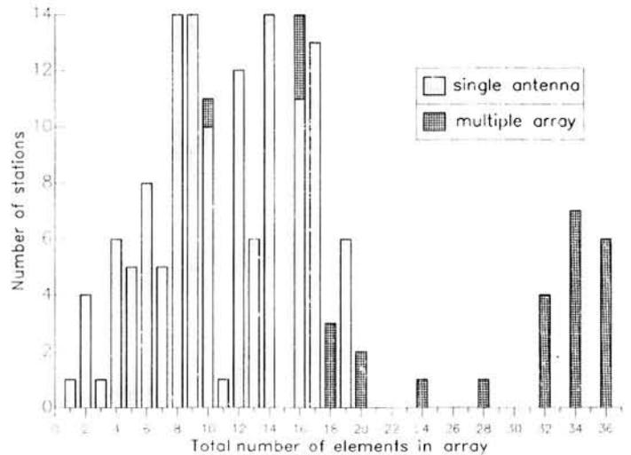
chart is only one 11-element antenna and a complete lack of any with 15-elements, and similarly no 22- or 30-element arrays corresponding to a pair of Yagis of this size. There was one other array not shown on the chart; one of 51-elements—G4BVY/P with 3 x 17-element Yagis.
