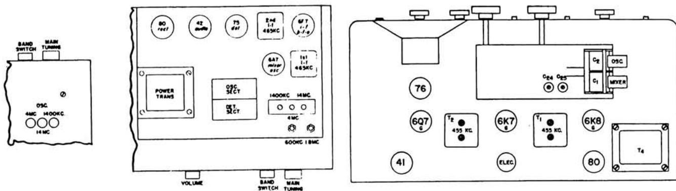
**Fig. 3: Location of trimmers, etc., on the Sky Buddy 5-T (above) and the S-19R (right)**
