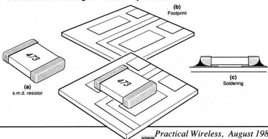
protected by layers of lacquer and a resinous coating. They are largely impervious to moisture and objectionable gases. Surface mount devices on the other hand have little or no protection. Prepared circuits can therefore be sprayed with a protective lacquer - not essential but good practice once a circuit is completed and de-bugged. A solder-through lacquer is the only choice here.
