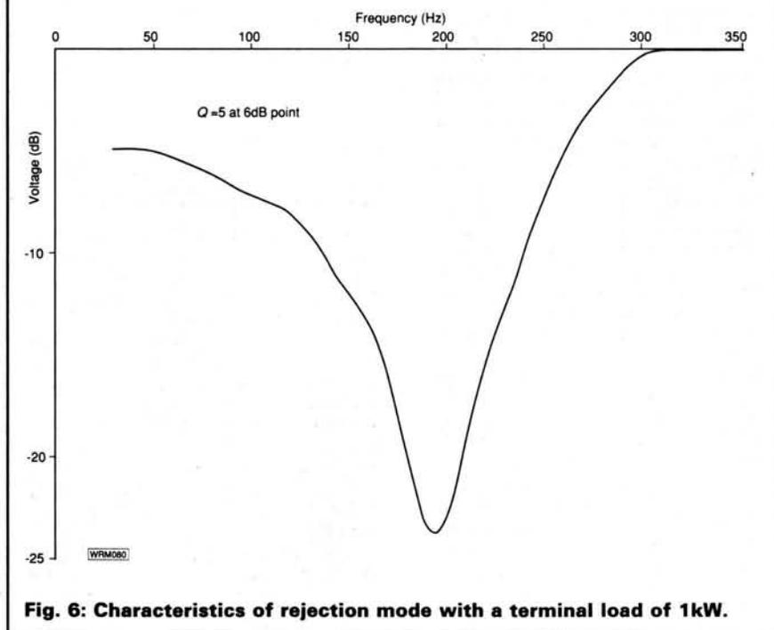
Fig. 6: Characteristics of rejection mode with a terminal load of 1kW.
