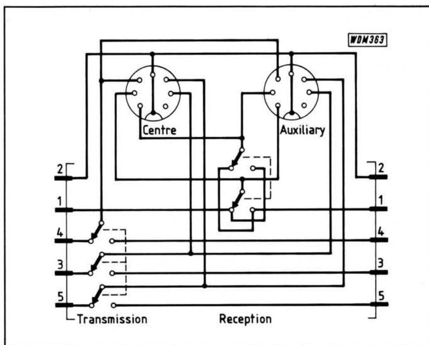
Fig.2.2: Wiring for the Dual Rig Selection Box
