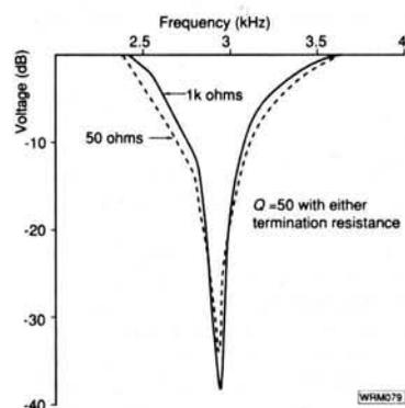
Fig. 5: Rejection mode filter characteristics. Centre frequency 2.95kHz
