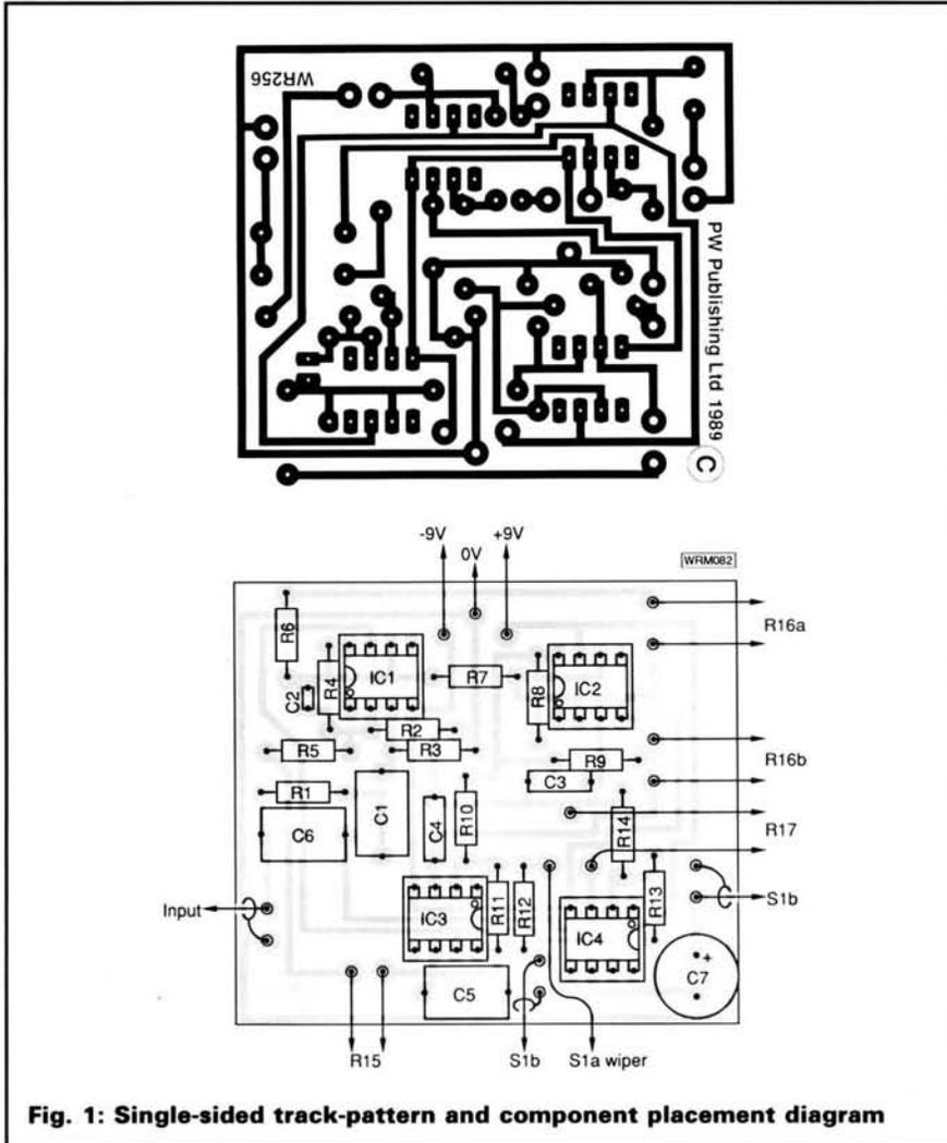
Fig. 1: Single-sided track-pattern and component placement diagram
