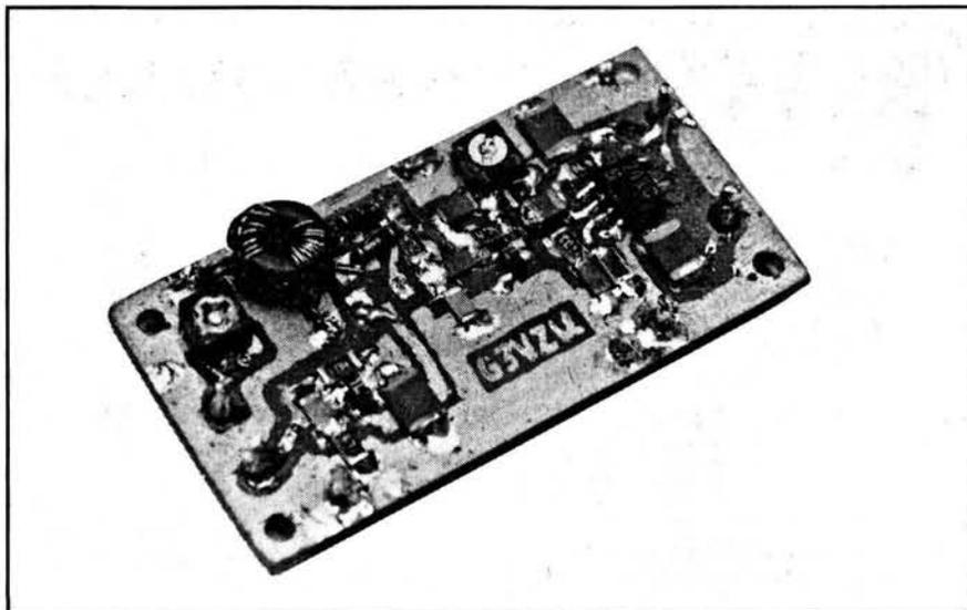
**A heavily re-worked prototype showing a variety of s.m.d.s in use**
