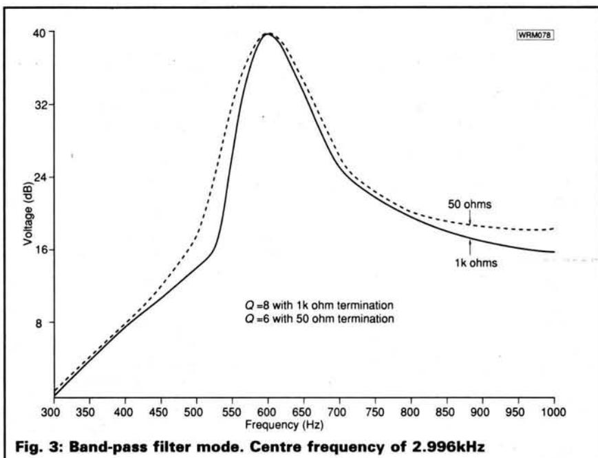
Fig. 3: Band-pass filter mode. Centre frequency of 2.996kHz
