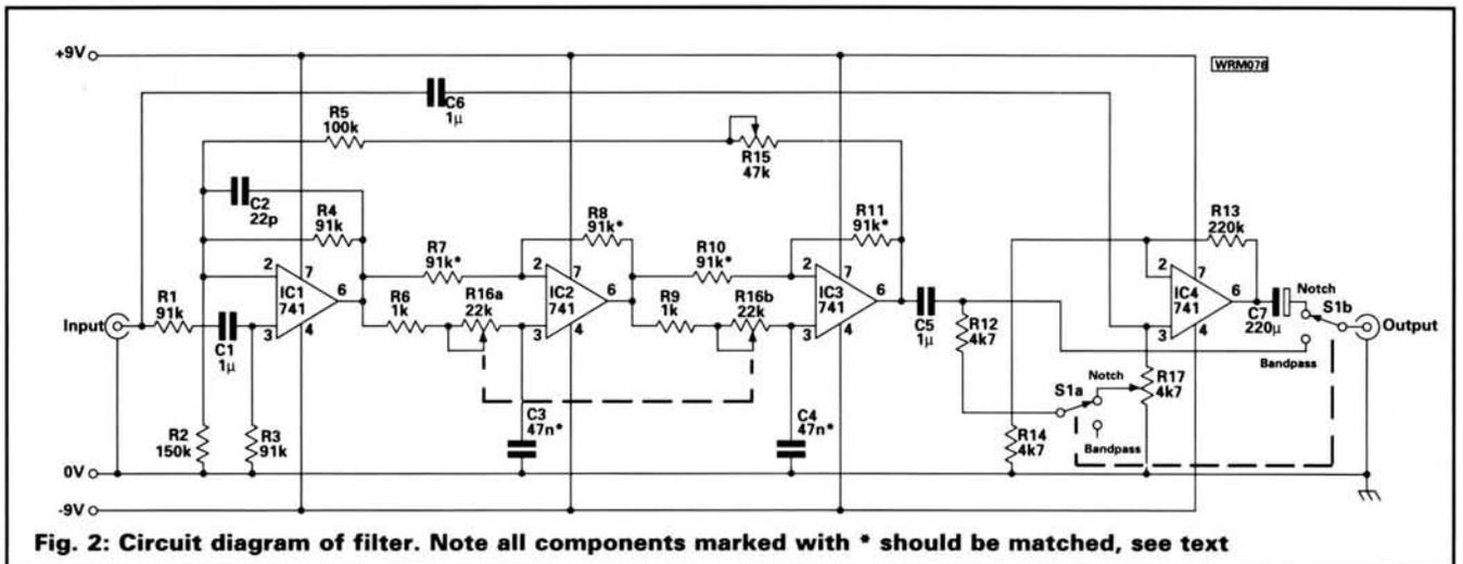
Fig. 2: Circuit diagram of filter. Note all components marked with \* should be matched, see text
