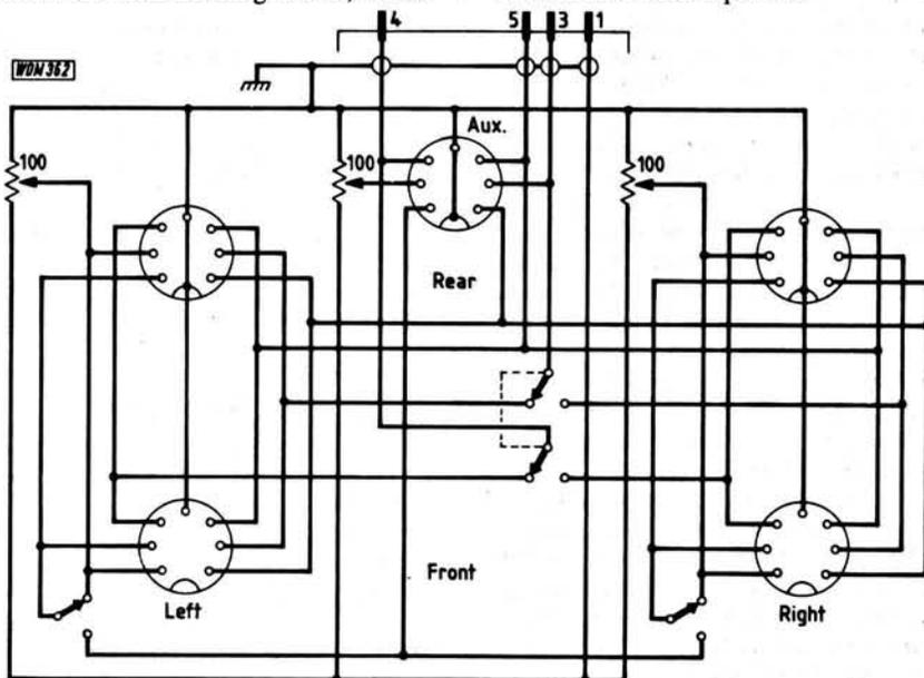
Fig. 2.1: Wiring for the Dual Operator Outlet Box
