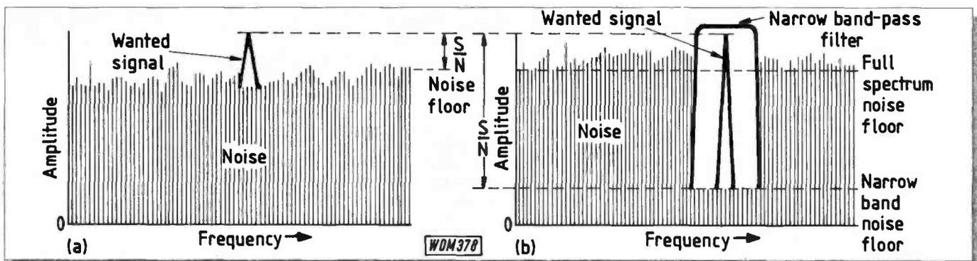
**Fig. 2: A wanted signal almost buried by noise over a relatively wide spectrum (a) resulting in a very poor S/N. Part (b) shows how the S/N can be greatly improved by passing the signal through a narrow band-pass filter**
