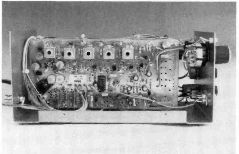
The *PW Cub* shown mounted in the Badger box. It may be seen that only one crystal has been fitted, although there is space for six. The screens are visible low down towards the left hand side of the board, separating the r.f. coils.
