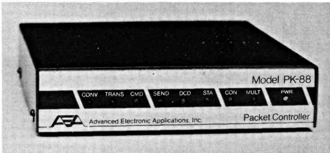
any of your packets are awaiting acknowledgement, 'SEND' showing p.t.t. status, 'DCD' indicating data is present on air, 'Connected' and 'Multiple Connect' modes, and Power On.
