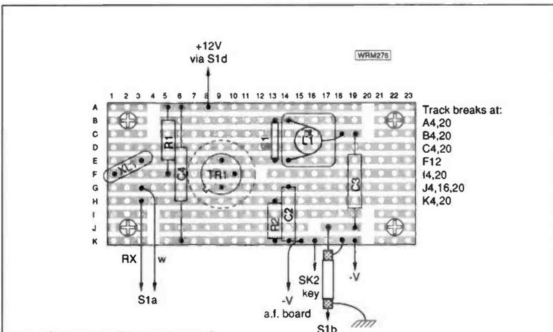
Fig. 2.1a: Oscillator board.
