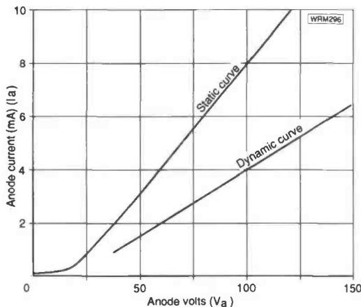
voltage is increased the space charge surrounding the heated filament (or cathode) begins to thin out and the electrons move toward the anode. This allows the migrating electrons to be replaced with more from the filament. Anode current increases as anode voltage is raised and eventually a point is reached where the number of electrons reaching the anode is matched by the number leaving the filament. This is the saturation point for the particular filament temperature. To increase anode current
