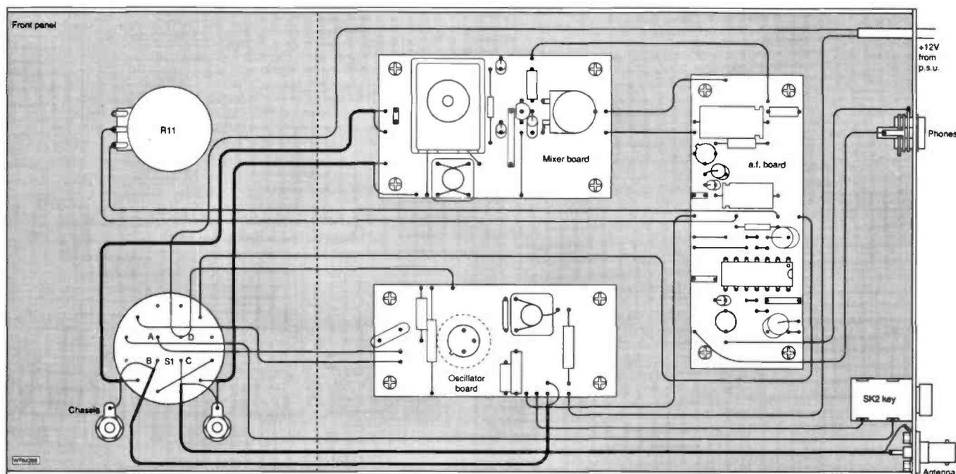
**Fig. 2.2: Overall interwiring. Note front panel 'bent' for clarity.**
