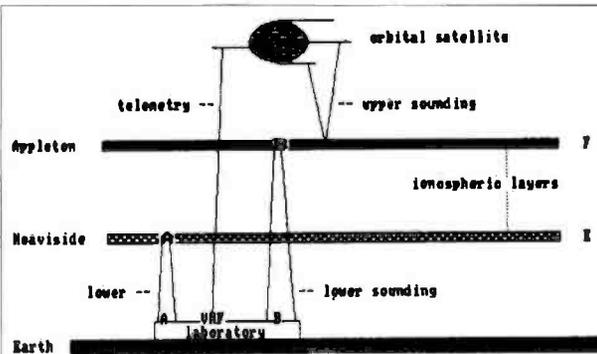
**Fig. 1: Using a satellite-borne ionosonde for upper layer sounding.**
