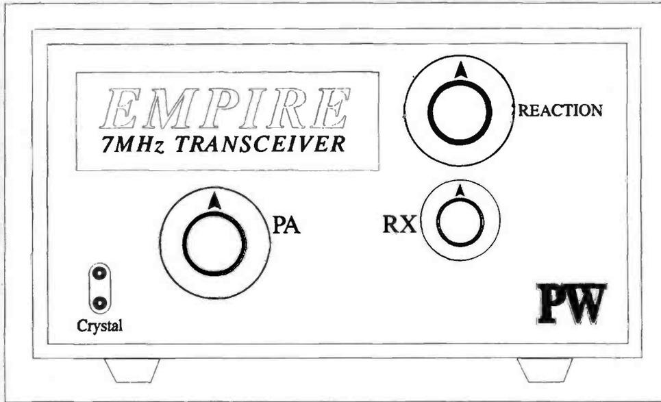
*This new 'old' transceiver has been specially developed for the 1000th issue. It uses 90V h.t. 1.5V heater valves and may be operated from the power supply described in the May 90 issue of PW*
