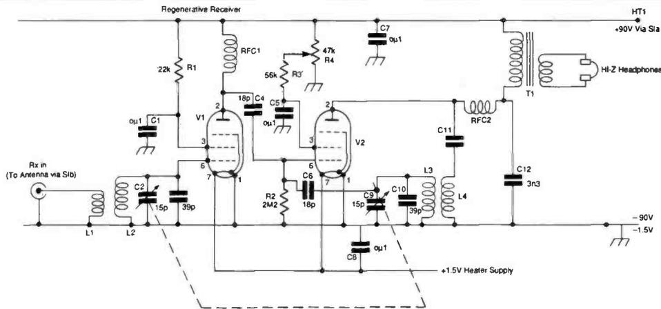
Fig. 1: The receiver circuit.
