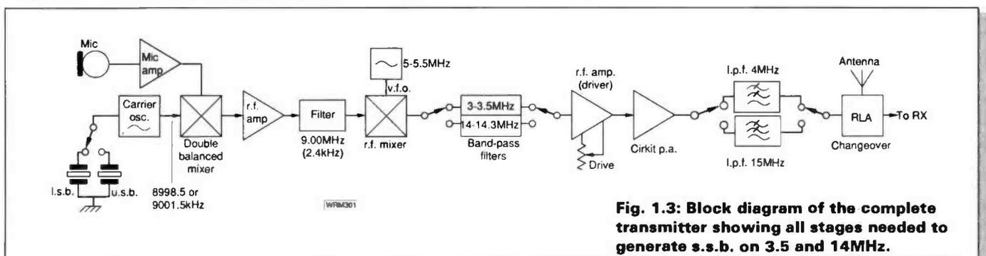
Fig. 1.3: Block diagram of the complete transmitter showing all stages needed to generate s.s.b. on 3.5 and 14MHz.
