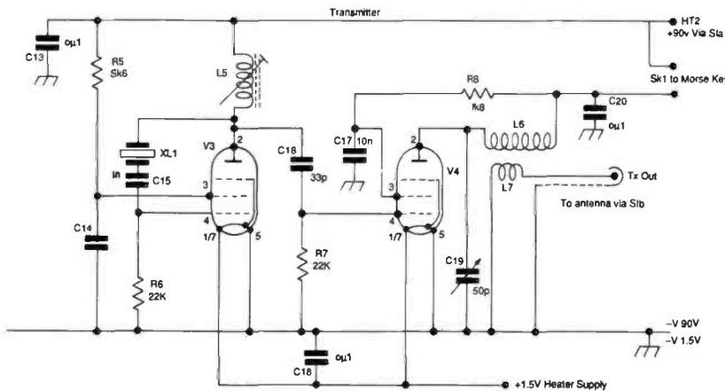
Fig. 2: The transmitter circuit.
