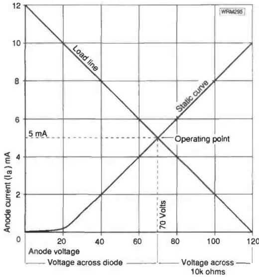
**[c] Static diode curve accompanied by the dynamic curve for an anode load resistor of 10kΩ**
