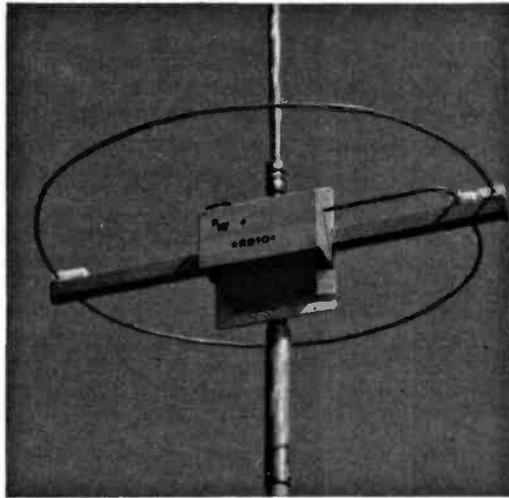
The RB10 stems from the 'Ring Base' antenna that I designed some years ago for 144MHz band operation. (*PW*, September 1982, subsequently reprinted in *Wires and Waves*) which employed a half-wave radiating element.
