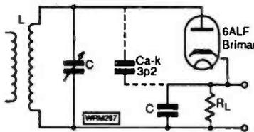
**Fig. 1.5: This shows the simple circuit for a diode detector that would demodulate a.m. signals found on the broadcast bands. In addition the means of arriving at the best value for the diode load and the value of capacitor has been described**
