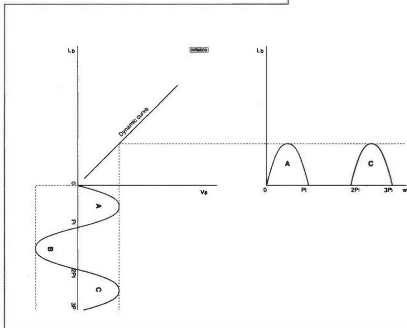
**Fig. 1. 6a. Showing a.c. input and half wave rectified d.c. output.**
