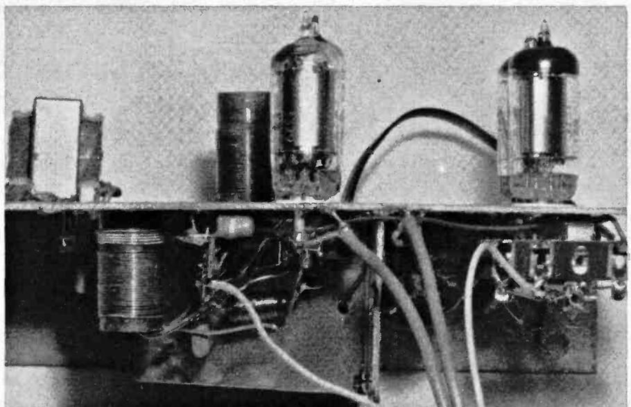
A new technique for valve equipment — using P.C.B. material for the 'chassis' construction.
