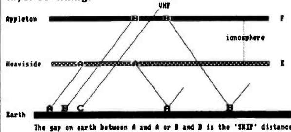
**Fig. 2: Ionospheric sounding signals penetrating the Heaviside layer, led to the discovery of the Appleton Layer.**
