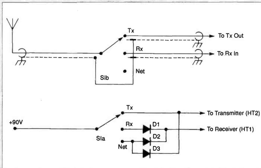
Fig. 3: The Empire transmit-receive switching circuitry.
