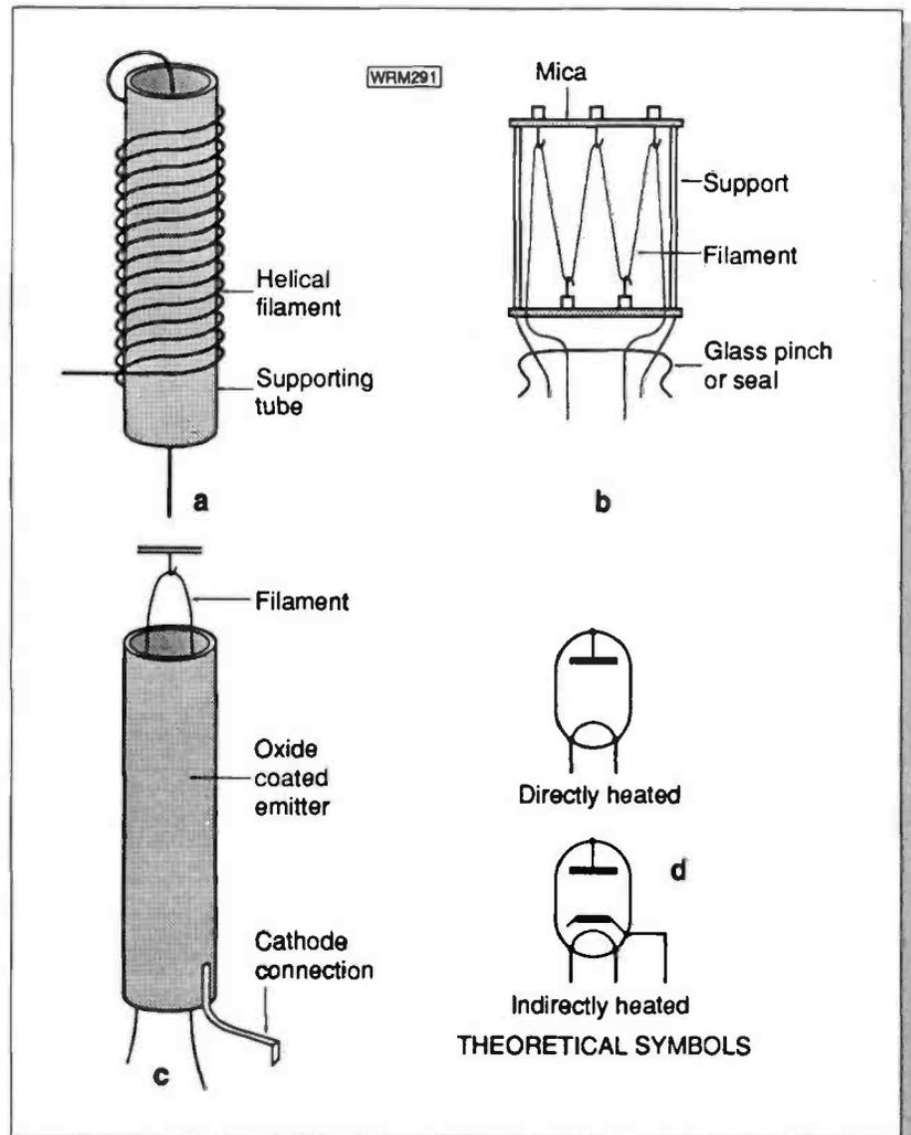
Fig. 1.2: [a] Helical wound filament on supporting insulated tube. [b] Zig-zag filament supported on mica bridges held apart by insulating tubes. [c] Indirectly heated emitter or cathode. The cathode is coated with oxide to increase emission. [d] Diode valve symbols for directly and indirectly heated cathodes
