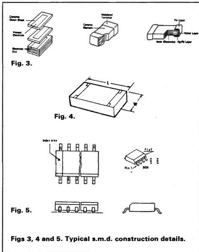
Figs 3, 4 and 5. Typical s.m.d. construction details.
