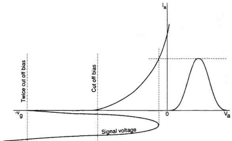
**Fig. 5.5: Almost full drive under class 'C' operation showing how the drive voltage has increased.**
