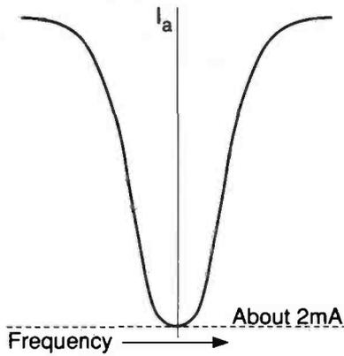
**Fig. 5.3: The unloaded anode current as the frequency is swung about the resonance point of the circuit. This shows a distinct fall of  $i_a$  to about 2mA at resonance,  $R_D$  is about 125k $\Omega$ .**
