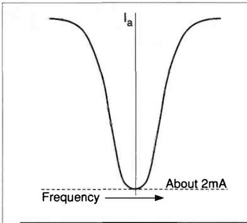
**Fig. 5.3: The unloaded anode current as the frequency is swung about the resonance point of the circuit. This shows a distinct fall of  $i_a$  to about 2mA at resonance,  $R_D$  is about 125k $\Omega$ .**
