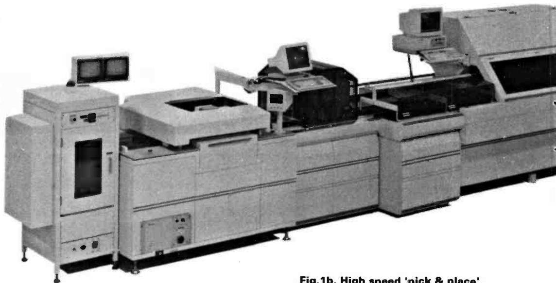
Fig.1b. High speed 'pick & place' production line, working at 14 000 placements per minute.
