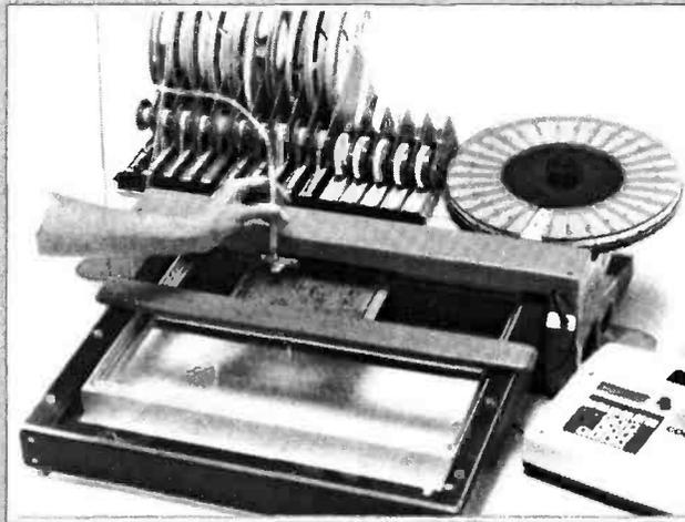
**Fig. 2b.** An advanced, manual 'pick & place' machine.
