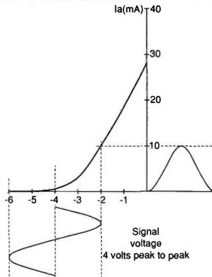
**Fig. 5.4: At the new bias level of -4V showing the 'peakiness' of the anode current.**
