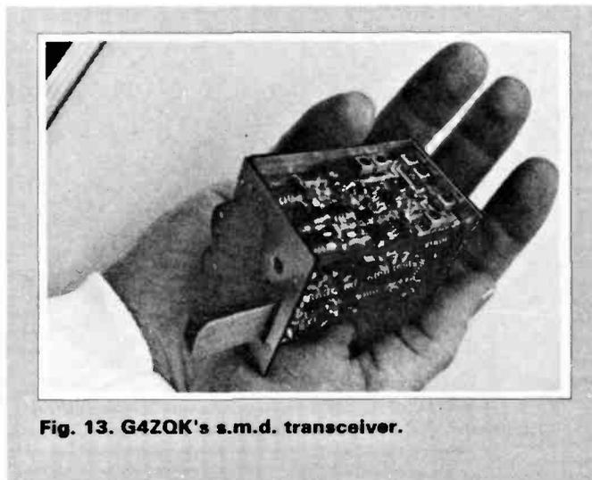
Fig. 13. G4ZQK's s.m.d. transceiver.
