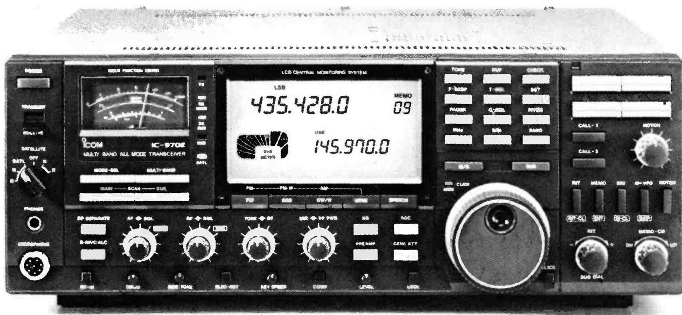
Designed for the serious operator on the 144, 430 and 1200MHz bands, Icom's new IC-970E has up-to-date technology for DX, digital and satellite communications.
