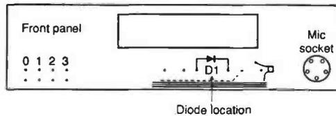
**Fig. 1:** This modification gives 12.5kHz step on the band 136-179MHz.
