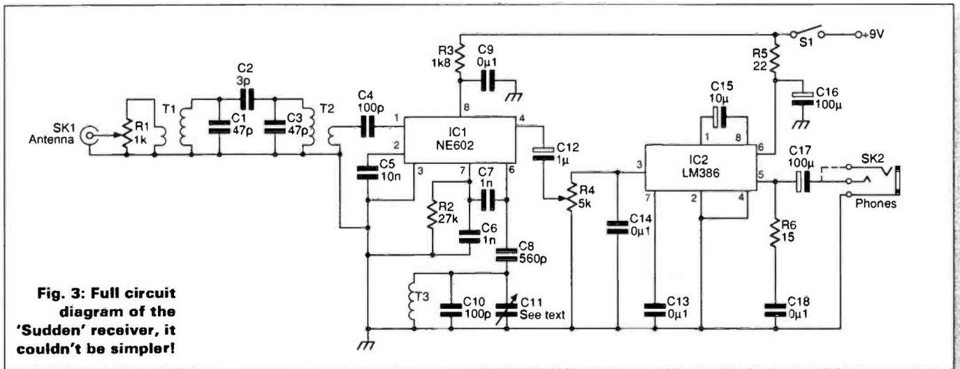
**Fig. 3: Full circuit diagram of the 'Sudden' receiver, it couldn't be simpler!**
