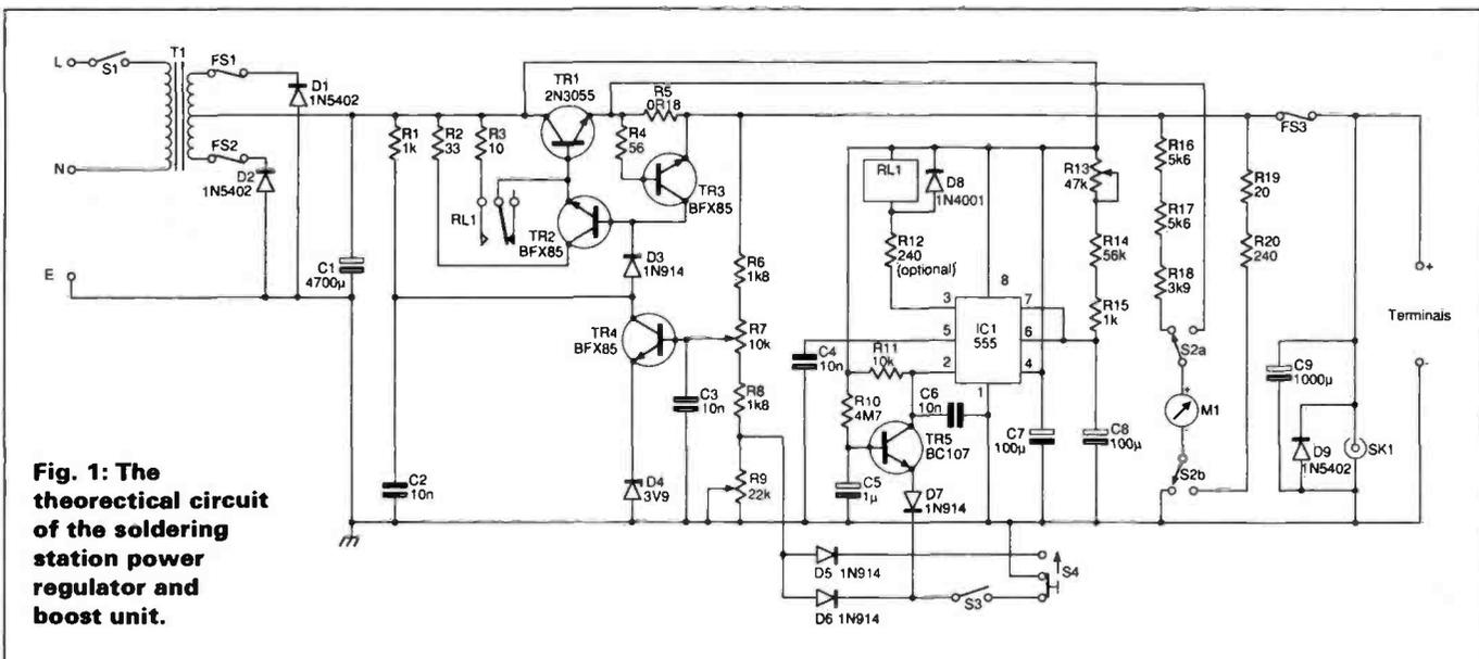
**Fig. 1: The theoretical circuit of the soldering station power regulator and boost unit.**
