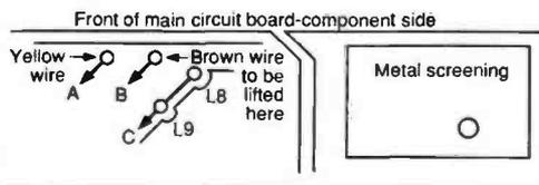
**Fig. 2:** The brown wire, gives user-selectable a.m./f.m., when removed and taken via a switch and resistor to the regulator output.
