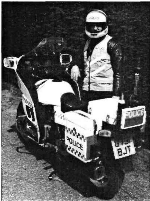
Fig. 1: PC 919 ready for action! The audio and radio control leads run between Bill French's helmet and the handlebars while the associated transceiver and antenna are at the very rear of the 'bike.
