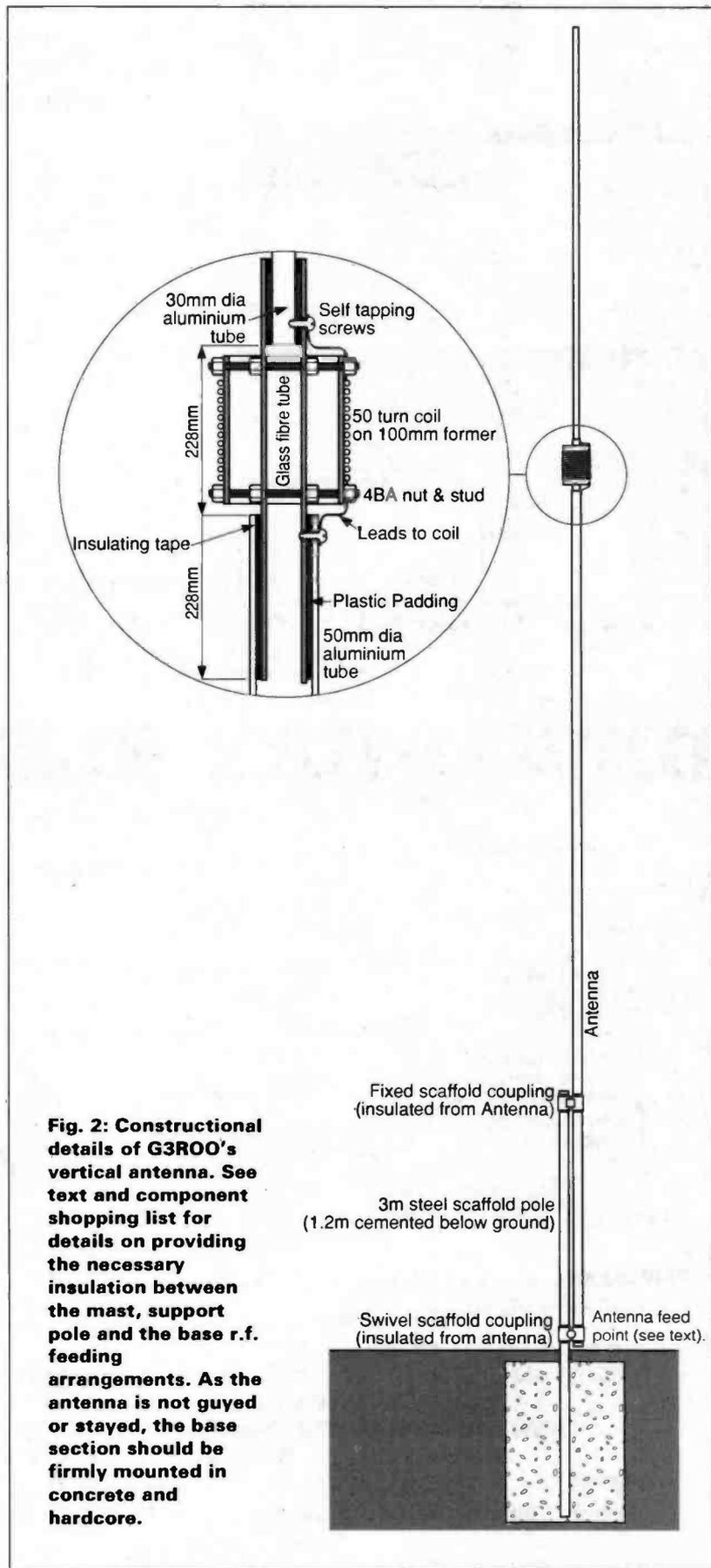
**Fig. 2: Constructional details of G3ROO's vertical antenna. See text and component shopping list for details on providing the necessary insulation between the mast, support pole and the base r.f. feeding arrangements. As the antenna is not guyed or stayed, the base section should be firmly mounted in concrete and hardcore.**
