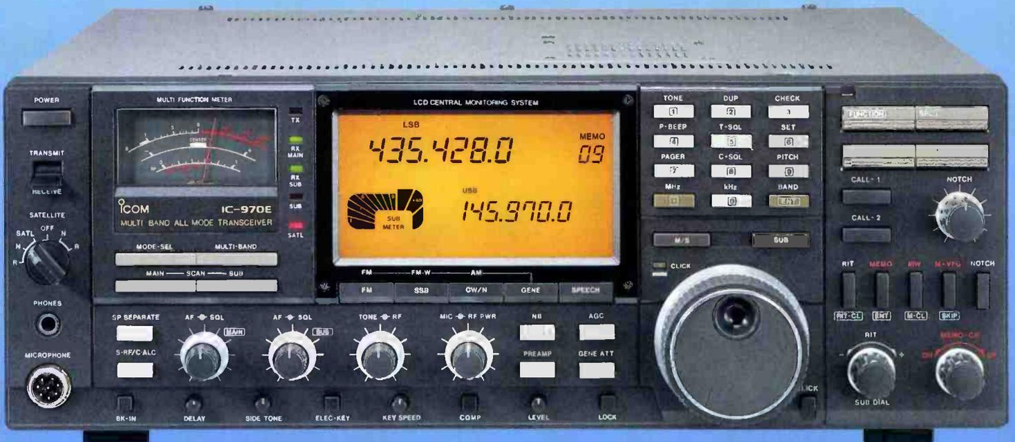
Designed for the serious operator on the 144, 430 and 1200 MHz bands, Icom's new IC-970E has up-to-date technology for DX, digital and satellite communications. The IC-970E is supplied as an all mode dual-bander for 144MHz and 430MHz bands. Optional units expand its capabilities to 1200MHz or wideband receiving from 50-905MHz.
