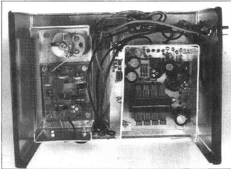
**The completed Chatterbox transmitter section. The v.f.o. section is to the left, with the variable capacitor for frequency control visible in the top left hand corner of the picture. The power amplifier and modulator stages are to the right, with the modulation transformer shown located in the middle of the 'u' shaped combined heatsink and screening panel (see text).**
