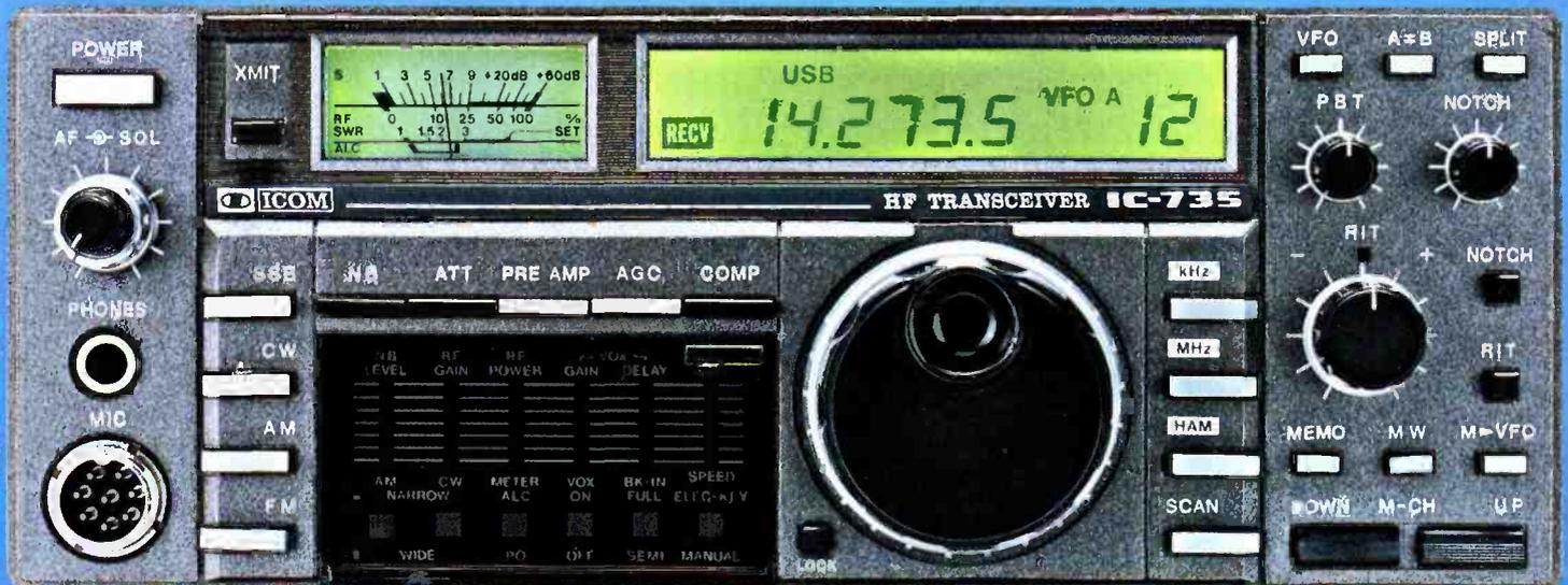
As predicted the Icom IC-735 has rapidly gained the reputation it deserves. This compact transceiver is ideal for mobile, portable or base station operation. It has a general coverage receiver from 0.1Mhz to 30Mhz with superb sensitivity in all modes; SSB, CW, AM and FM.
