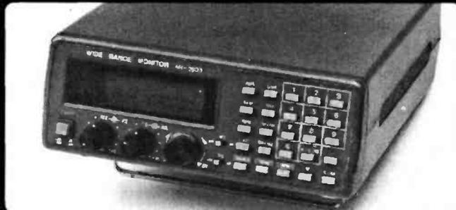
AR2800 Scanning Receiver with SSB 500kHz - 1300MHz
