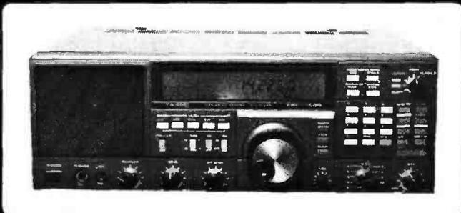
Yaesu FRG8800 HF Receiver 150kHz - 30MHz
