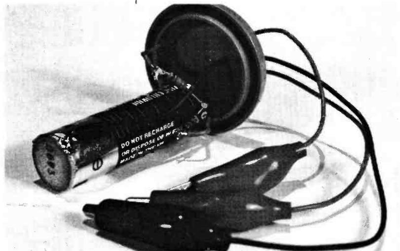
so that deflection of the coil (and the needle) is to the right. As the current passing through the coil increases, the needle moves more towards the right, indicating the increase in current flow.
