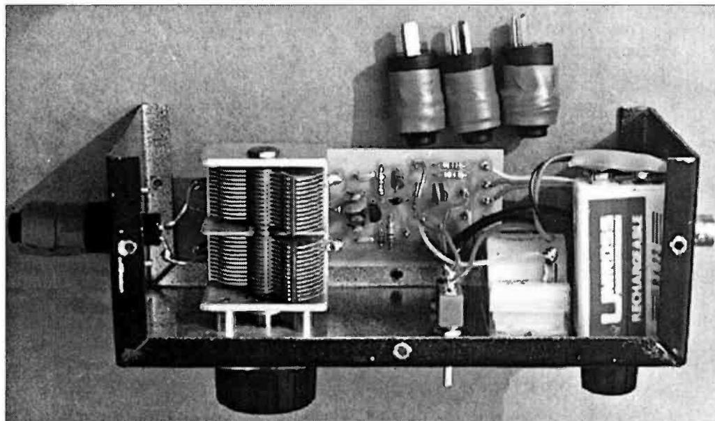
Fig. 3: The Jandek dip-meter and its associated tuning coils, tried out and discussed by G3LDO (see text).
