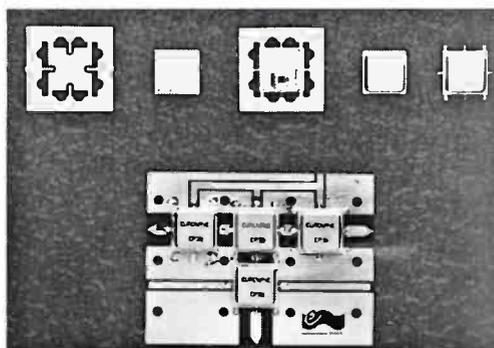
applications. The v.c.o.s are available in both the lead type and surface mounting formats.
