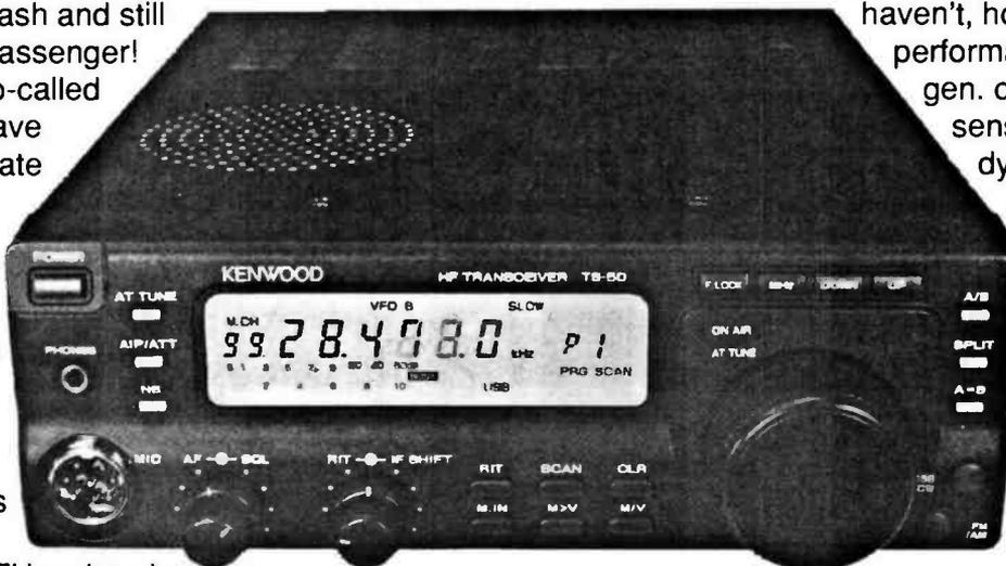
Quite how Kenwood have squeezed so much into such a tiny package, I can only marvel at. They haven't, however, skimped on performance: All modes, gen. cov. RX, 0.25µV sensitivity on ssb, a dynamic range of 105dB and a full 100W output.
