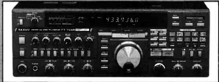
**YAESU FT-736R** This transceiver from Yaesu incorporates up to 4 band modules covering the 50, 144, 430 and 1200MHz Ham bands. The standard model provides 25 watts RF power output on the 144 and 430/440MHz bands in SSB, CW and FM modes with any 2 of the remaining 3 bands as options (10 watts output on the 50 and 1200MHz bands). An 8-bit CMOS main micro-processor and 4-bit I/O coprocessor provide exceptional digital integration and control.
