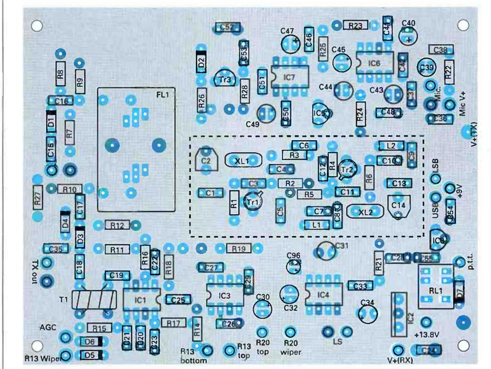
**Fig. 3.1:** The printed circuit board design, ground plane and associated overlays for the main 9MHz i.f. and filter used in the PW Jubilee 14MHz s.s.b. mobile transceiver. The dotted line surround XL1, 2 and Tr1 and 2 indicate where screening of the section could be applied (see text for comments).
