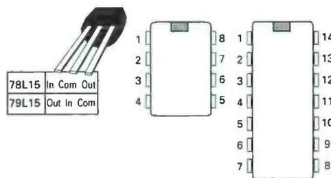
**Fig. 7: Pinouts for the three i.c.s used. Both the '741 and '747 i.c. pins are counted from above.**
