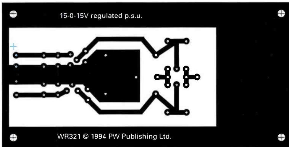
**Fig. 6: The track and overlay of the simple dual 15V p.s.u.**
