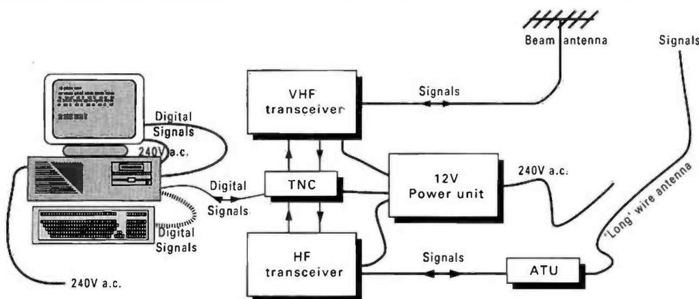
**Fig. 1: Typical interconnections in an amateur radio/computing installation (see text).**
