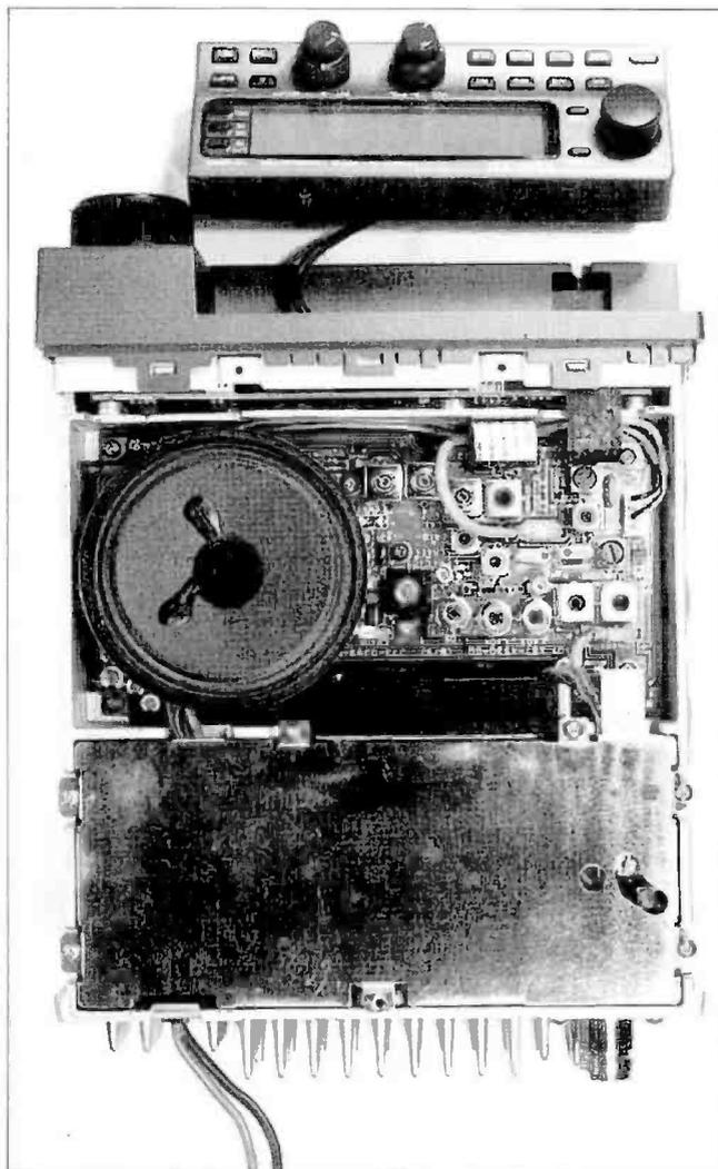
**The TM-255E transceiver shown with the removable main front panel detached. With the optional accessory remote control cables (see text) the transceiver can be mounted as far as 7m from the operating position. The relatively large speaker incorporated into the Kenwood TM-255E assists in providing excellent audio reproduction (see text for comments).**
