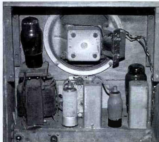
**Fig. 5: The 'Utility' set employed a 'Westector' detector, which can be seen between the potentiometer and the large capacitor (see text).**
