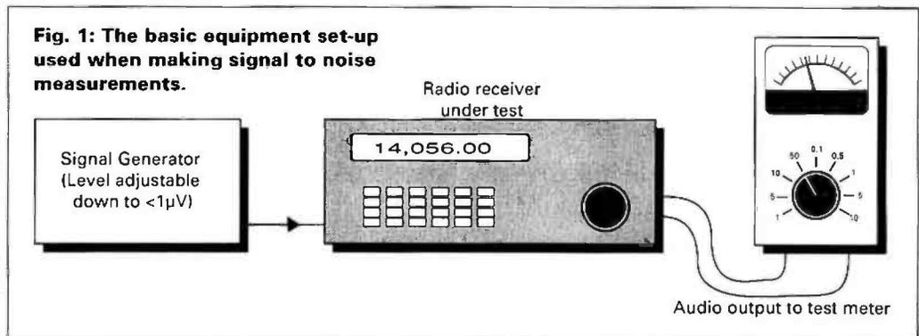
Fig. 1: The basic equipment set-up used when making signal to noise measurements.
