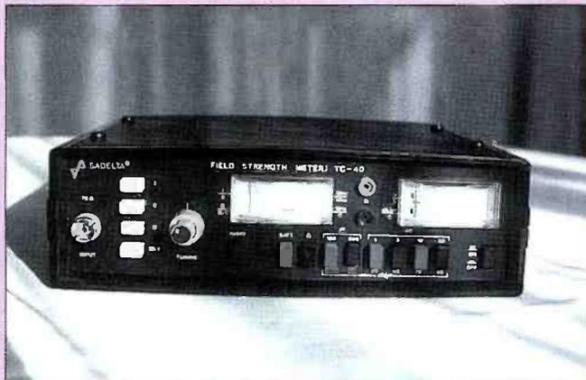
**Fig. 1: Designed originally for domestic v.h.f. radio and TV signal strength metering, this f.s.m. from Sadelma is nonetheless very useful for amateur frequencies.**
