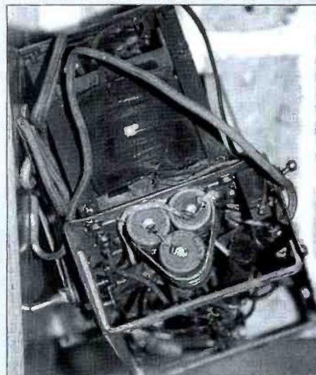
**Fig. 4: Illustration showing the smoothing capacitors in the power supply of the wartime 'Utility Receiver' (see text).**
