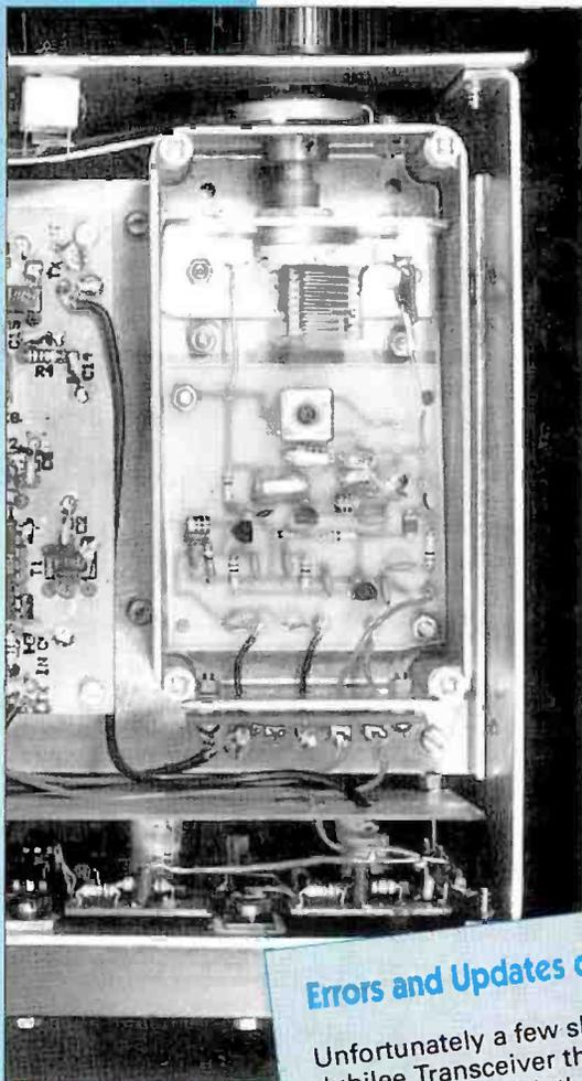
**Fig. 3.4:** Close up view of the v.f.o. section of one of the prototype Jubilee transceivers. To ensure the best possible stability in the circuit G3RJV recommends that care is taken when assembling the v.f.o. and the best quality variable capacitor is used (see text).
