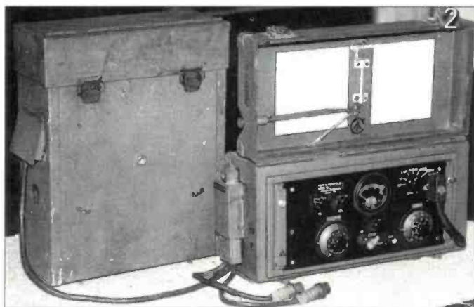
Fig. 2: The Canadian 58 set with its associated back-pack vibrator power supply unit (left).
