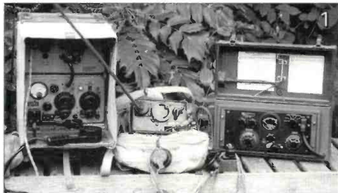
Fig. 1: A trio of Second World War military radio equipment. The 18 set (left), 38 set (centre) and the lesser known Canadian 58 set (see text).
