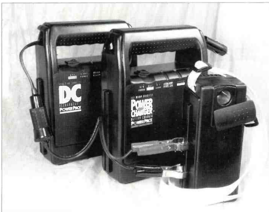
The Innova Electronics Corporation's PowerPack portable battery system tested by Tex Swann G1TEX.
