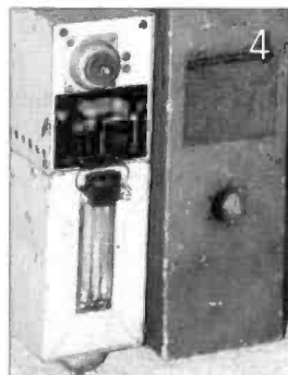
Fig. 5: The 58 set used 2V accumulators for primary power. The built-in 'floating ball' hydrometers can be seen on each cell (see text).
