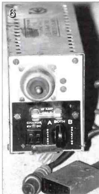
Fig. 6: The control panel on the 58 set enabled the operator to select either 'A' or 'B' or both accumulators by the central switch. They could be charged from a 6V d.c. source via the adjacent 4-pin socket.
