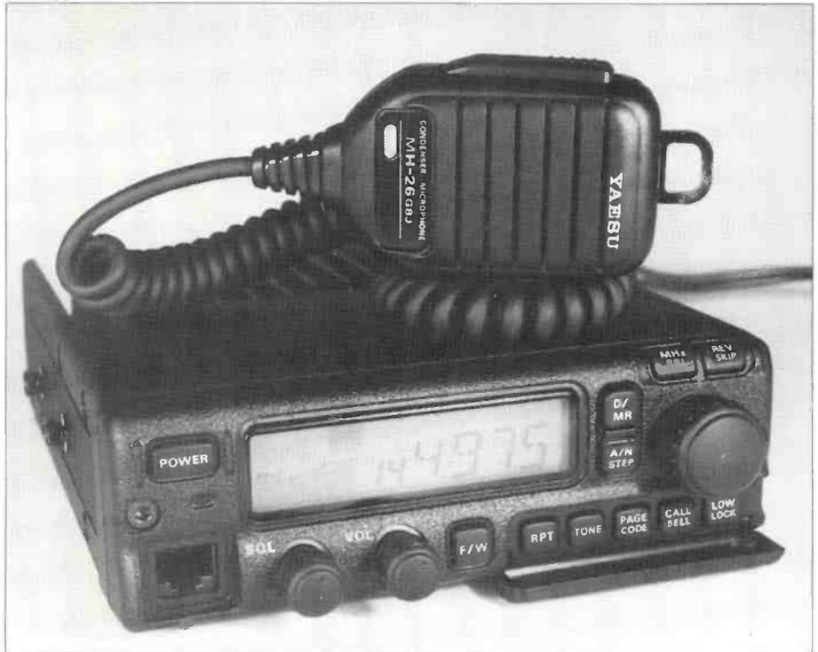
The Yaesu FT-2500M mobile transceiver.
