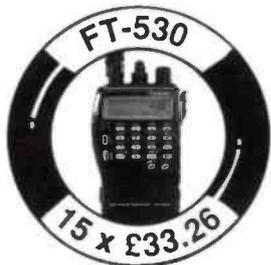
Dual band handheld 2m/70cms c/w 7.2V 700Ma. Ni-Cad & charger
