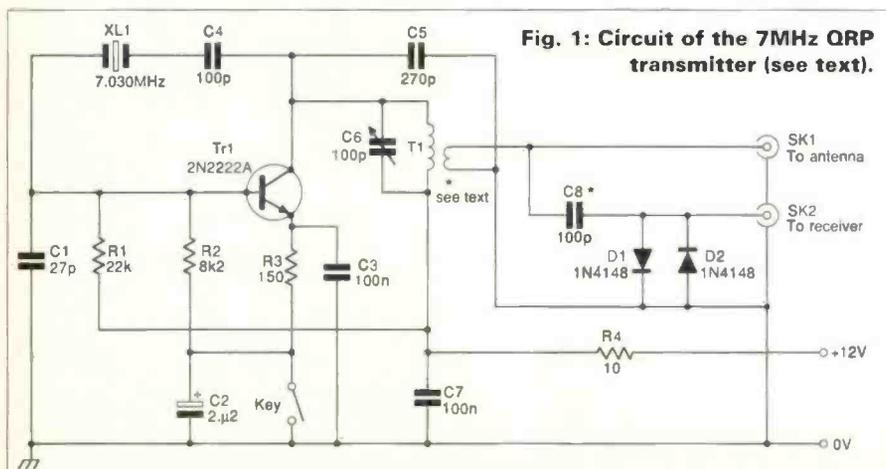
Fig. 1: Circuit of the 7MHz QRP transmitter (see text).
