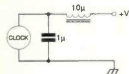
**Fig. 6: Circuit for vehicle clocks, suitable for analogue or digital types (see text).**
