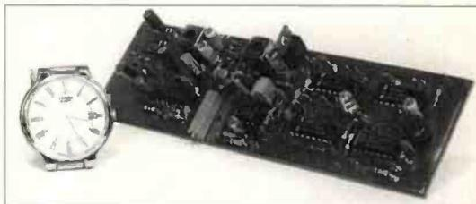
Walford Electronics have recently added a new kit to their range which designer Tim Walford G3PCJ says will be of interest to keen home constructors and designers. The **Reference** kit has been designed to provide a range of highly accurate reference frequencies for use in counter timebases with an optional wide bandwidth **Input** h.f. amplifier and u.h.f. prescaler. The Reference kit can be used on its own, or with the Walford Electronics two channel Frequency Counter.
