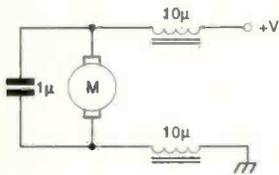
**Fig. 3: Alternative circuit for interference suppression (see text).**
