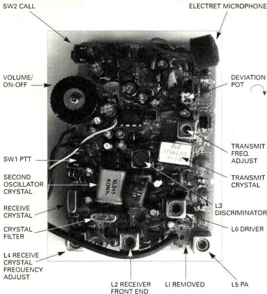
**Fig. 1: The main transceiver p.c.b. removed from its case. (See text for details on the 49 to 50MHz conversion process). Annotations show major components involved in modifications. The coaxial cable (see G4SLU's text) connected in place of L1, is the antenna input/output.**
