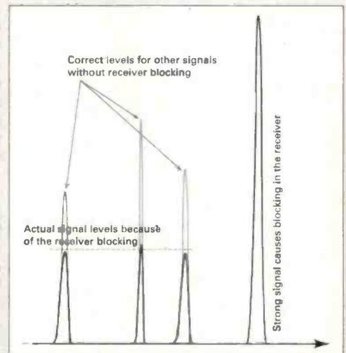
**Fig. 2:** Illustrating the 'Capture' effect (see text).
