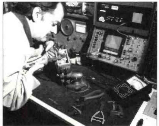
**Ben Nock G4BXD hard at work on his workbench. The 'third hand' being provided by the portable vice on the bench. Note the rubber bands on the hand-tools, to provide necessary grip (see text).**
