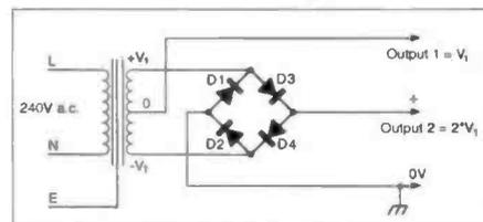
Fig. 1: A 'two rail' h.t. powers supply design used by G4JGS (see text).
