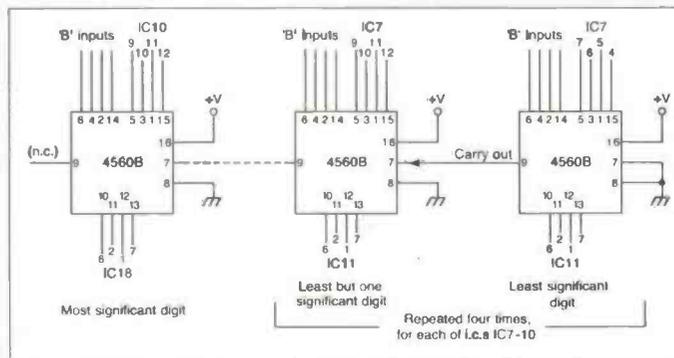
Fig. 3: The skeleton circuit of the adder circuit to give a frequency offset. The right hand pair must be duplicated for each of the counter i.c.s in the original PW Robin.
