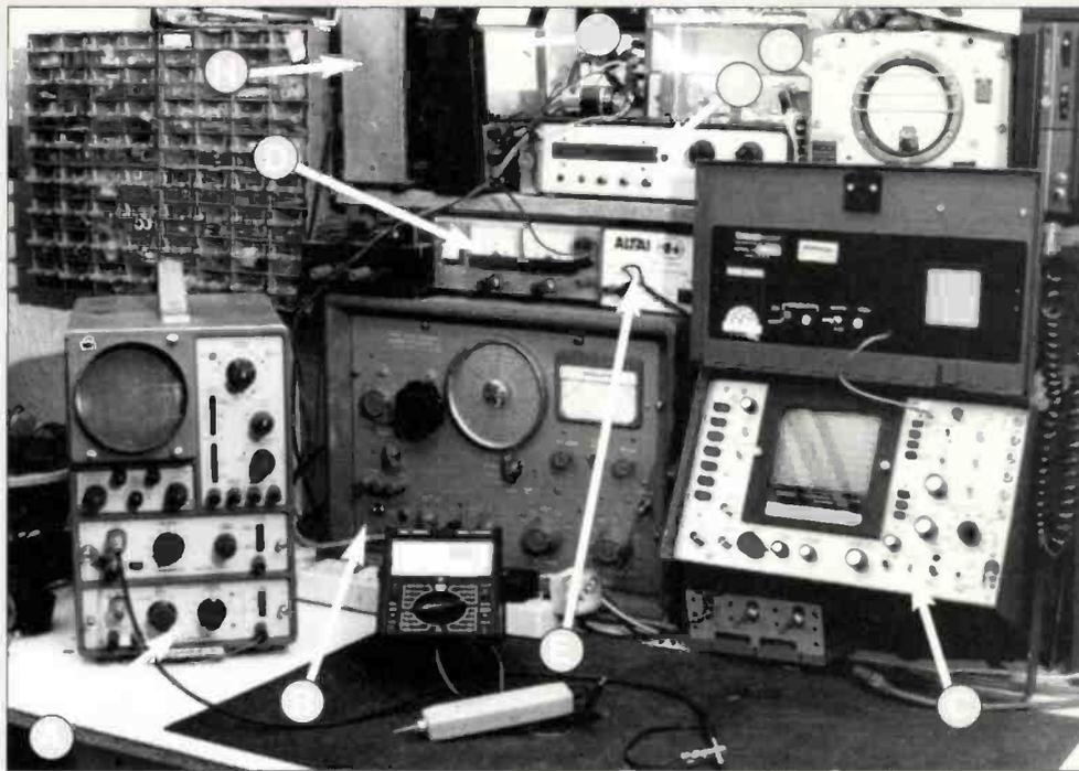
**Annotated photograph showing Ben's workshop Equipment Index: (A) 'scope 20MHz or better; (B) signal generator 1 -220MHz a.m./f.m.; (C) spectrum analyser 0-1GHz; (D) 2 - 30V p.s.u./A; (E) 13.8V 4A p.s.u.; (F) frequency counter 600MHz; (G) power meter using v.h.f./u.h.f.; (H) a.f. signal generator; (I) f.e.t. multimeter. (see text for recommendations on equipment.)**
