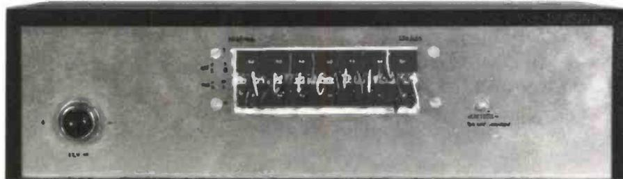
**On the back panel is a patch panel to allow any offset to be quickly programmed into the adder inputs.**
