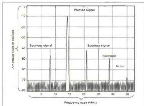
Fig. 1: A typical spectrum analyser plot.
