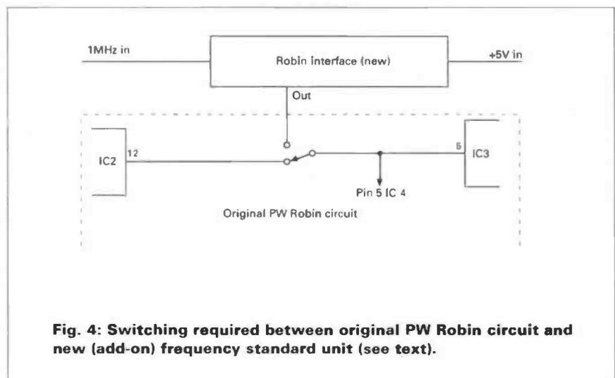
**Fig. 4: Switching required between original PW Robin circuit and new (add-on) frequency standard unit (see text).**
