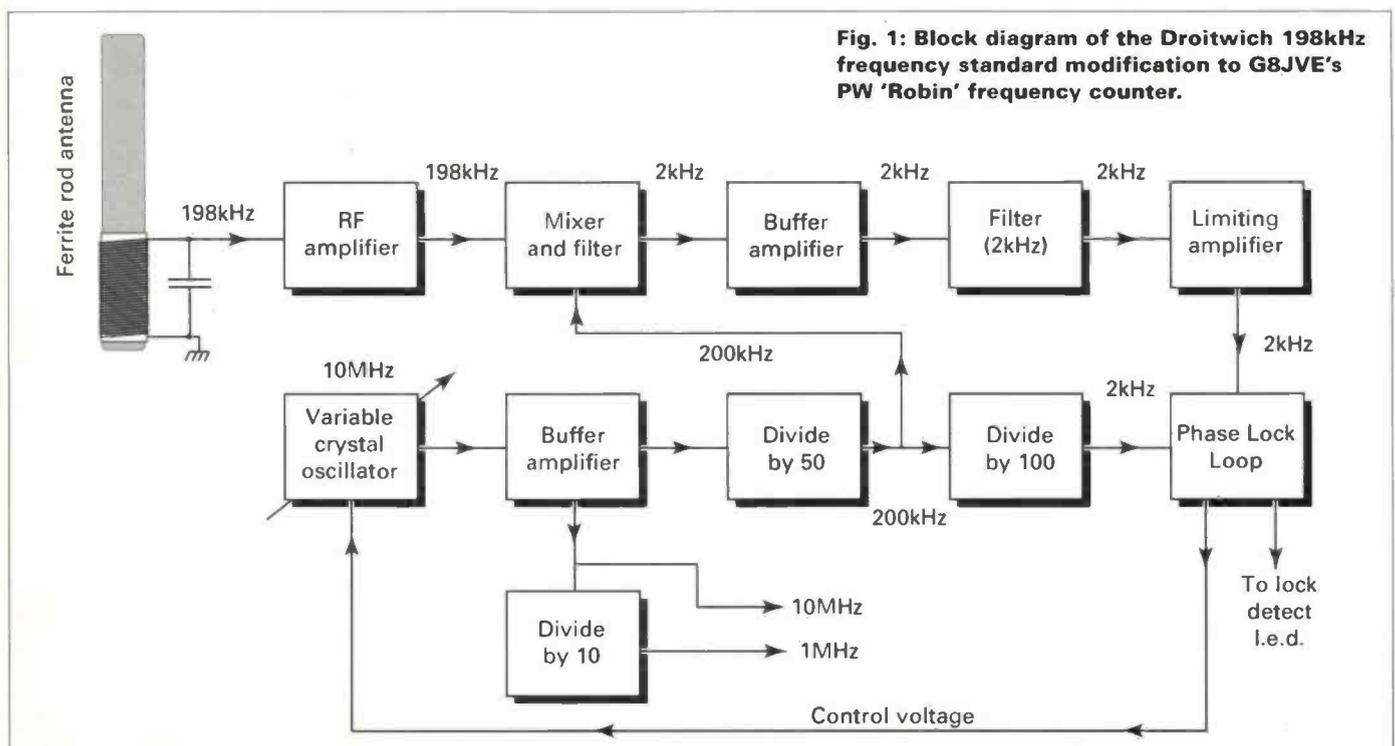
Fig. 1: Block diagram of the Droitwich 198kHz frequency standard modification to G8JVE's PW 'Robin' frequency counter.
