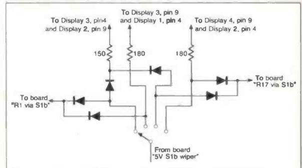
Fig. 2: A new range and resolution switch. Made by combining the simple switch of Fig. 1 and the function of the original Robin range switch.
