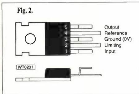
Fig. 2: Pin-out configuration of IC1.
