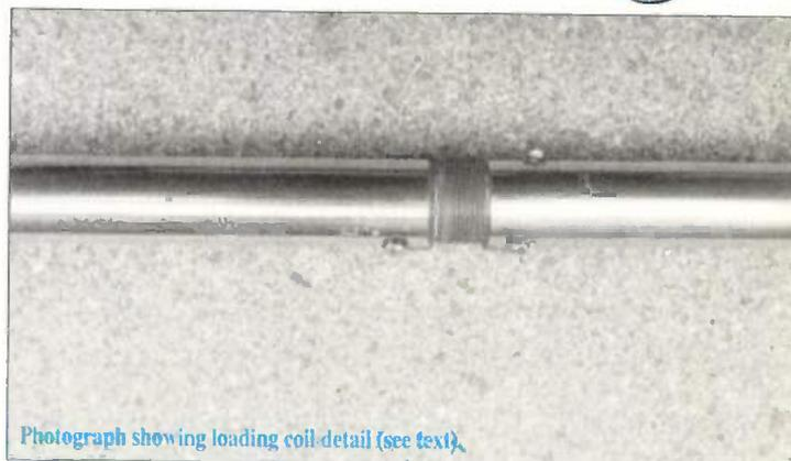
Photograph showing loading coil detail (see text).
