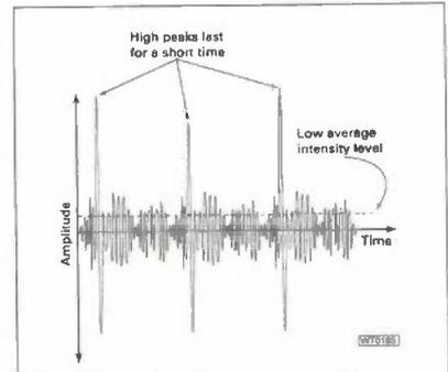
Fig. 1: A typical speech waveform.
