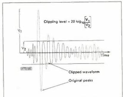
Fig. 2: Action of clipping a signal.
