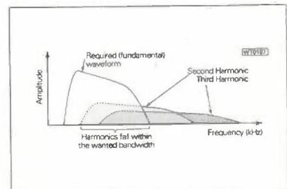
Fig. 3a: Clipping at a.f. showing the position of harmonics.
