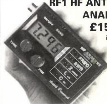
This pocket-sized analyser revolutionised antenna checking. Connected to any antenna it instantly reads out Impedance/SWR/Inductance/Capacitance at any frequency 1.2 to 35MHz.
