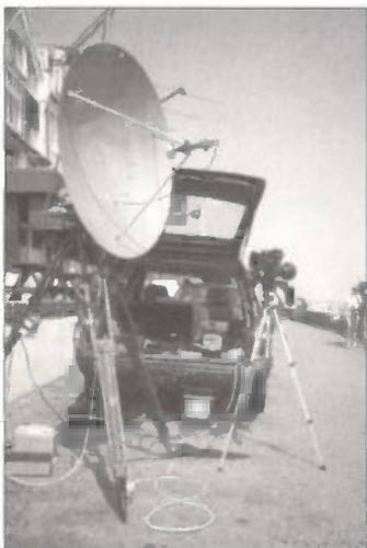
Gunn diodes make very simple and cost effective power sources for 3cm. Feed a 10mW Gunn diode into a small ex-satellite dish with a typical gain of 24dB and you achieve an effective radiated power of about 4W!
