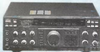
The Yaesu FT-990 has been a world best seller since its introduction a few years ago. Thousands world wide are used daily by Radio Amateurs who want a simple to use, beautifully built HF Transceiver. No other is built using plug-in boards for example, allowing servicing to be quick and easy. The FT-990 was the first to offer Digital Filters allowing high and low cut to the received signal.
