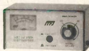
MFJ-816 MFJ-816 HF wattmeter lets you read forward and reflected power on 2 scales -- 30 and 300 watts -- and SWR from 1.8 to 30 MHz. Toroid current pickup gives uniform sensitivity. Easy push-button operation. Sturdy eggshell white and black aluminum cabinet. SO-239 connectors. 2-color meter scale. Compact size -- 4 1/2 x 2 1/4 x 3 inches -- makes it ideal for portable use.
