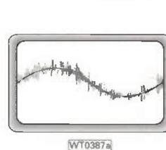
Fig. 1a: Typical ripple as seen on a linear regulator.
