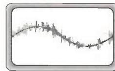
Fig. 1a: Typical ripple as seen on a linear regulator.
