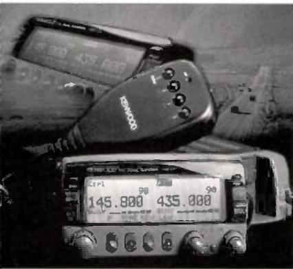
A feature which will be of interest to many v.h.f./u.h.f. mobile operators is the TM-V7E's 'Auto Simplex' checker facility. This checks whether or not it's possible to achieve simplex, rather than repeater, communication.
