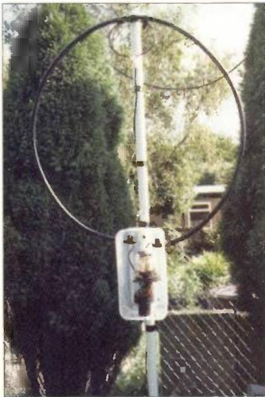
Perspex sheet 800x400mm. To aid tuning a 10:1 slow motion drive and tuning control was then added.
