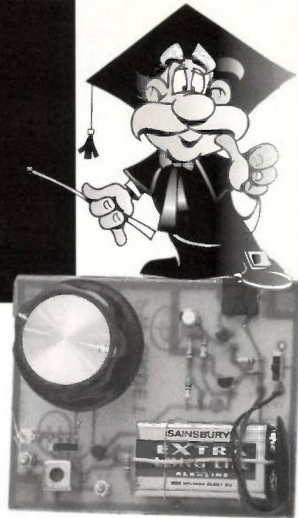
At the end of the assembly stage Barry had learned (thanks to the comprehensive and clear instructions provided in the kit and some help and reassurance from me) how to identify the resistors and capacitors and their associated values. He also learned how to handle the transistors and to solder them correctly.
