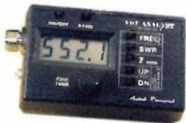
bands, over which it will measure frequency, s.w.r. or impedance automatically, displaying the result on a four digit display. Like its low frequency partner, the RF5 runs from a single 9V battery and has a series of small push-buttons to select the desired function to be displayed.
