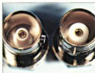
Fig. 1: Two BNC sockets. The 50Ω version is on the right and the other is a 75Ω socket.
