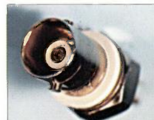
Fig. 4: Bought at a rally - is this BNC socket a 50 or a 75Ω type? (See text).
