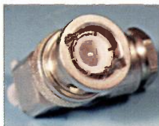
Fig. 3: Bought at a rally - is this BNC plug a 50 or a 75Ω type? (See text).
