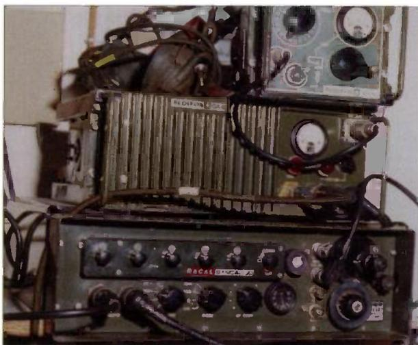
The Racal Syncal 30 connected to the Redifon amplifier. The large knob on the lower right of the Syncal 30 is the control for the internal 'Roller Coaster' type antenna tuning unit.
