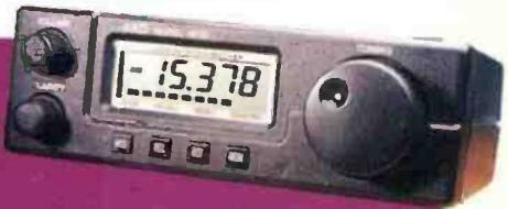
The long established range of AKD budget British-made fm. transceivers includes the 2001 for 144MHz, which is now available with 1.2.5kHz channel spacing. The 50MHz version, the 5001 is now provided with CTCSS tone and full repeater facilities. (A kit is also available for customer upgrading for older transceivers).
