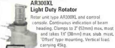
Rotor unit type AR300XL and control console. Continuous indication of beam heading. Clamps to 2" (52mm) max. mast and takes 1" (38mm) max. stub. mast. 'Offset' type mounting. Vertical load carrying 45kg. Special offer £49.95.
