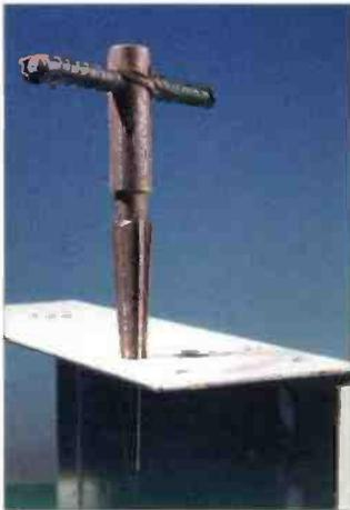
**Fig. 4:** A fluted reamer is useful for circular holes up to 12mm diameter.
