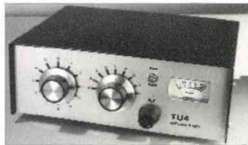
**Fig. 3: The Lake Electronics TU4 Antenna Tuner unit.**
