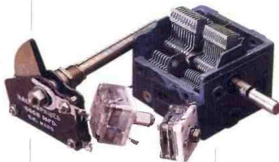
**Fig. 2: Photograph showing common types of variable capacitor. Solid dielectric type, often available as surplus (left), modern Polyvaricon types (centre) and traditional double ganged 'air spaced' from a broadcast receiver.**
