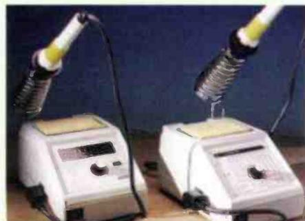
**A pair of temperature controlled soldering irons. The SL30 on the left with its digital display, the SL20 with a simpler bargraph on the right.**
