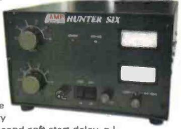
Features of the 'SIX' include an in-built heavy duty p.s.u., 3 second soft start delay, π-L input/output circuit and heavy duty by-pass relay. The amplifier can be keyed from most modern transceivers.
