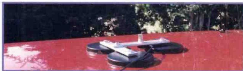
Fig. 1: Close up view of the MM-3401 triple magnetic mounting which proved more than capable of withstanding gale force winds (see text).
