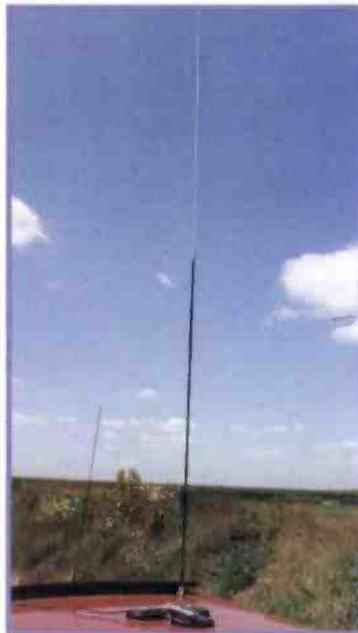
Fig. 2: The Pro-Am mobile whip antenna (the PHF-40B in this case) is over two metres long).
