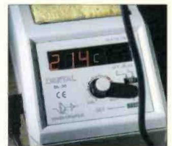
**The temperature setting is digitally displayed on the SL30 solder station.**
