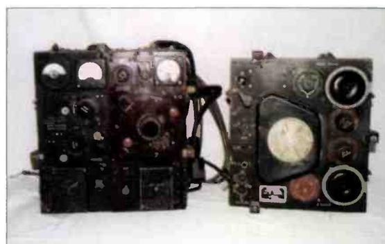
Fig 2: The RAF's T1083 and R1082 transmitter and receiver combination.
