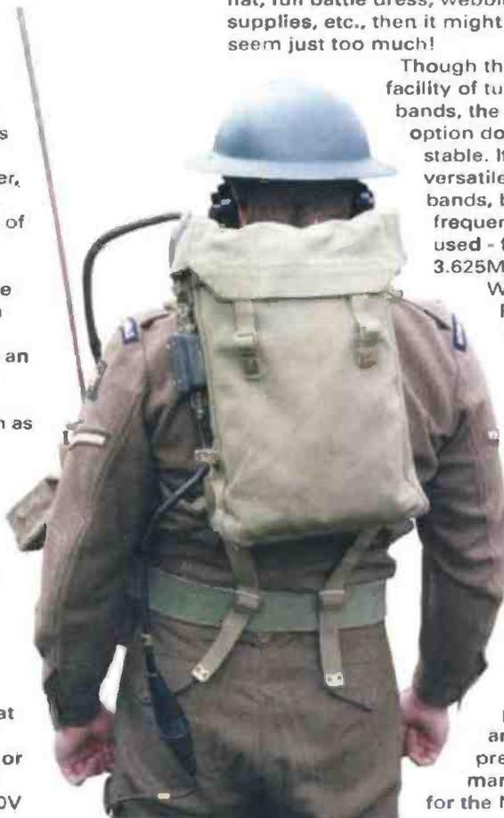
Fig. 5: The rear pack housing the battery. Note the headphones/microphone rubber connector.
