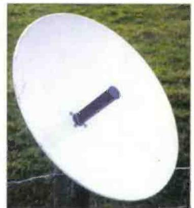
Fig. 6: The 460mm dish on a convenient fence post.
