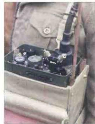
Fig. 4: The antenna unit for longer whips and wires. Note the rubber boot over the rear connector.
