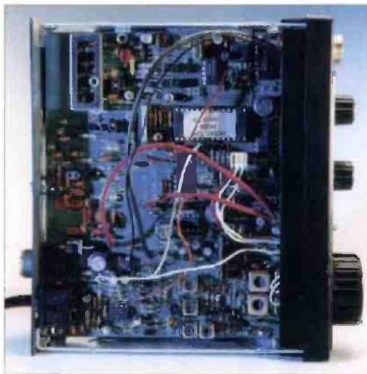
Fig. 8: Underside view of completed transceiver kit.
