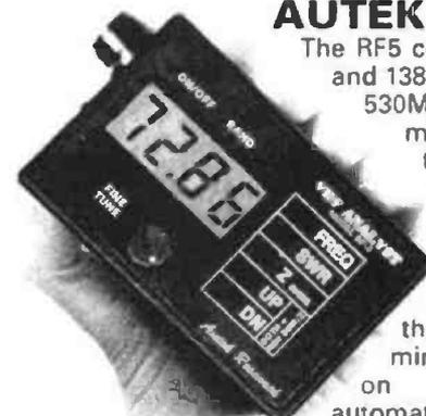
The RF5 covers 35 to 75 MHz, and 138 to 500MHz (typically 530MHz) in 3 bands. It measures RF values of true impedance (0-600Ω), SWR (1 to 6:1). It has no direct L & C as the RF1 but an INSTANT SWR mode which finds the frequency of minimum SWR (or Z) on command automatically. The RF5 fits in the pocket, and runs on a standard 9v battery.
