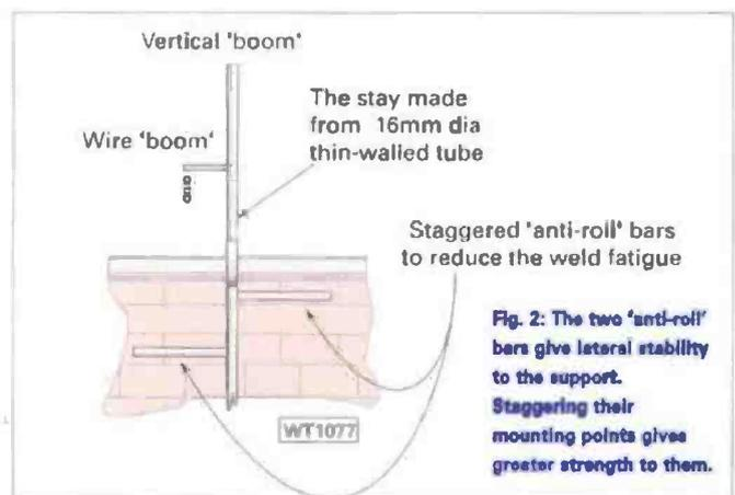
Fig. 2: The two 'anti-roll' bars give lateral stability to the support. Staggering their mounting points gives greater strength to them.
