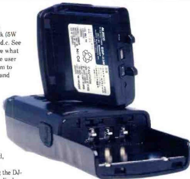
Fig. 3: The Alinco DJ-G5 with its "4.8V d.c. 700mAh battery pack".
