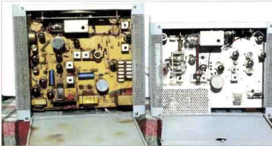
Internal view of the KW201 (left of picture) and of the KW 'Vespa' (right of picture). In the KW201 note the v.f.o. box (top centre), power supply (bottom right), calibrator (lower left) and s.s.b. filter below and to the left of the v.f.o. box. In the Vespa the p.a. compartment is on the lower left, with the v.f.o. in the top centre, the s.s.b. filters are glass valve-base types mounted on the centre left.
