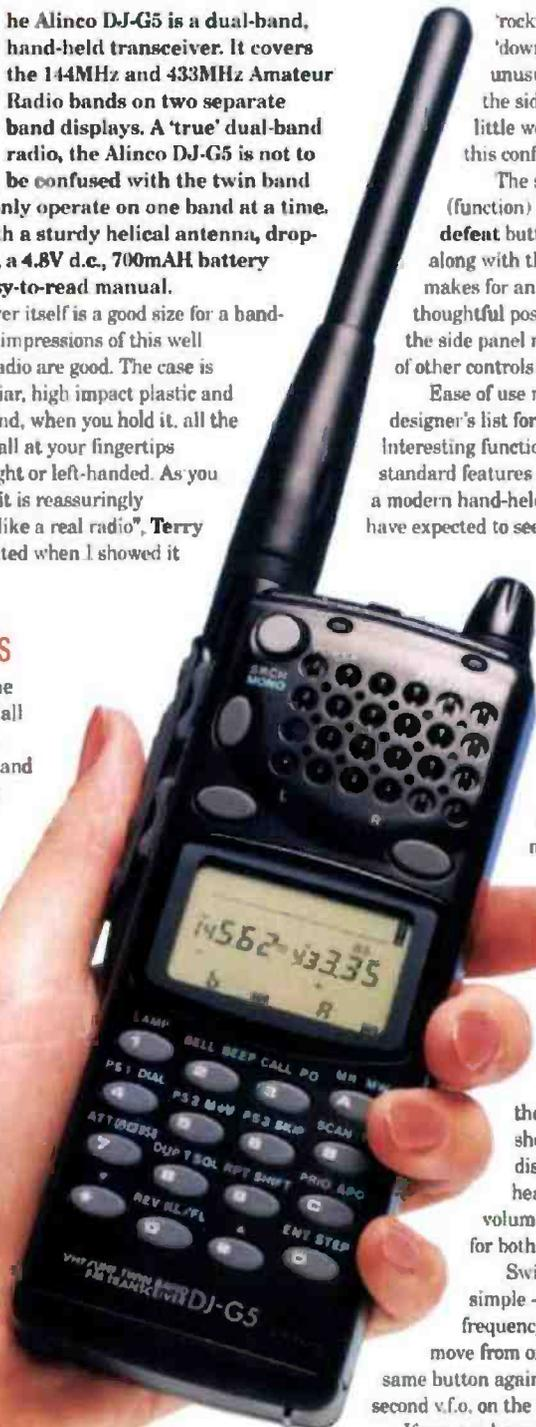
The Alinco DJ-G5 v.h.f./u.h.f. twin band f.m. receiver: "A 'true' dual-band radio".
