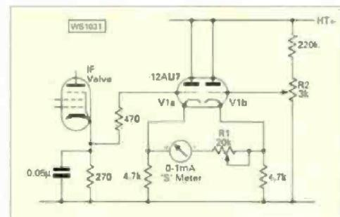
Fig. 3: An example of a bridge circuit form of S-meter using a double triode (see text).
