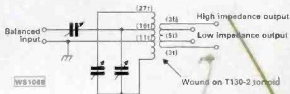
Fig. 2: Circuit of the antenna tuner unit. Note that the two variable capacitors shown side-by-side are actually a twin ganged (double 500pF) single unit.
