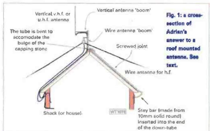
Fig. 1: a cross-section of Adrian's answer to a roof mounted antenna. See text.
