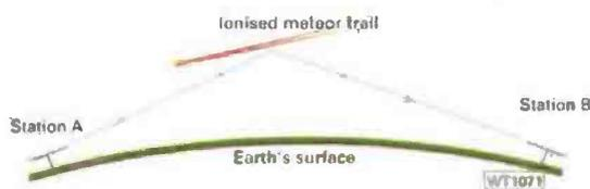
Fig. 1: Diagram illustrating one station transmitting towards the station being contacted via m.s. - forward scatter. (See text).
