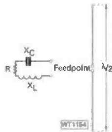
Fig. 1: The equivalent circuit of a centre-fed half wave dipole. At resonance  $X_L$  and  $X_C$  are equal and cancel, leaving only the resistance.
