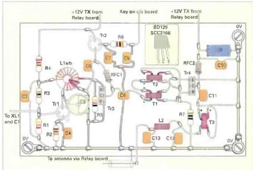
Fig. 3: A suggested layout for the transmitter board.
