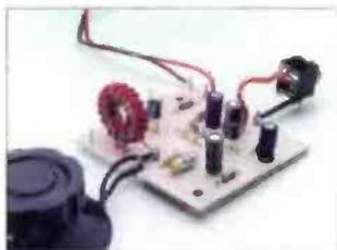
**Fig. 8: The built-up Novice Receiver from Lake Electronics. See text for more details.**
