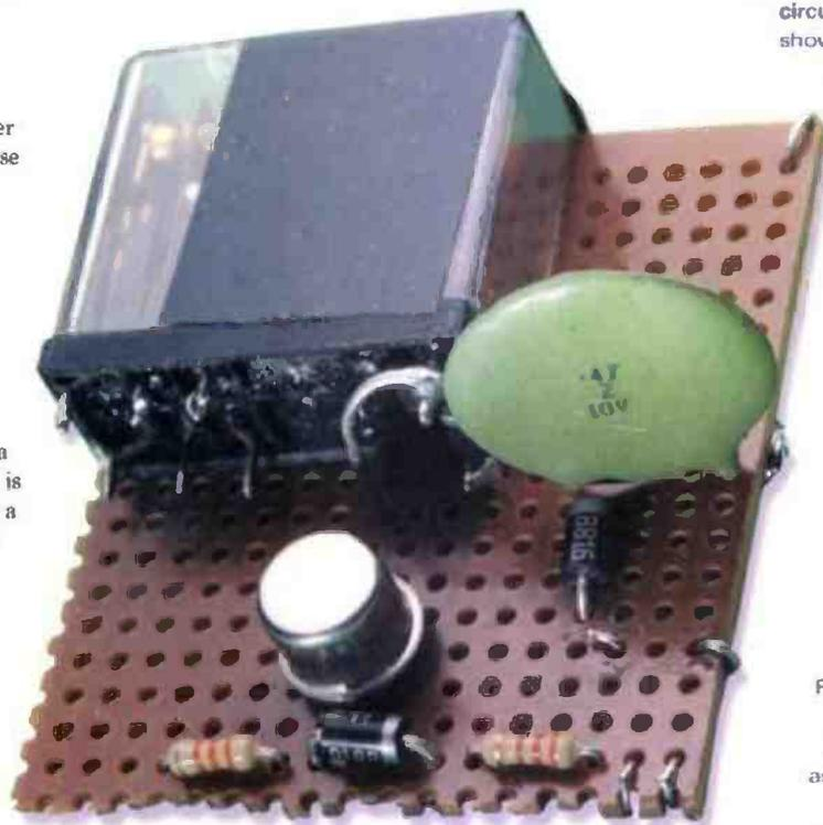
Fig. 3: The change-over unit assembled using perforated matrix board (see text).
