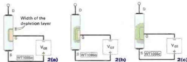
**Fig. 2 (a, b & c): Effect of gate voltage on the depletion layer.**
