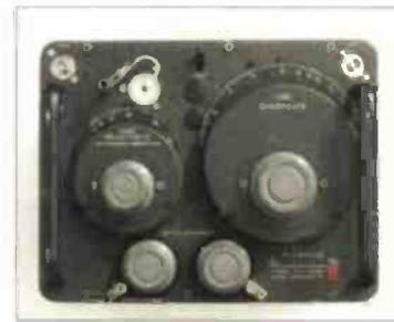
**Fig. 4:** A commercial r.f. impedance bridge, from the General Radio Company. This instrument needs a signal source, such as a signal generator and a receiver to detect when the bridge is balanced.
