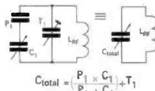
**Fig. 7:** How to calculate the total equivalent capacitance of a series parallel combination.
