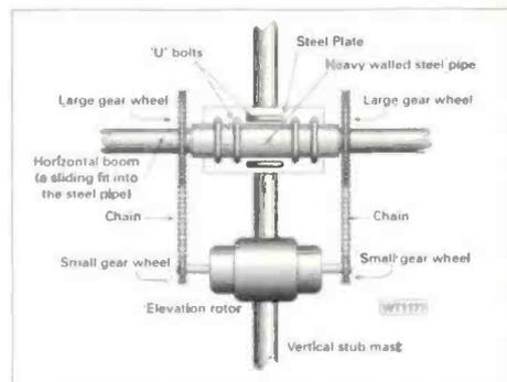
**Fig. 3a: Utilising a simple sliding-fit bearing (as explained in text) and chain wheel reduction gearing a small elevation rotator can elevate quite a large antenna array such as the 'H' frame of **Fig. 2**.**
