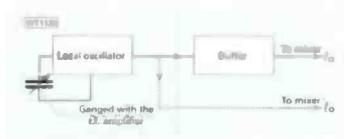
Fig. 1: Block diagram showing the possible presence of a buffer stage between the l.o. and mixer stages
