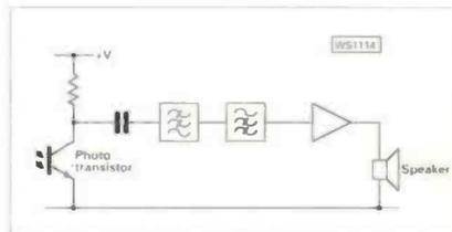
Fig. 2: Block diagram of basic laser receiver.
