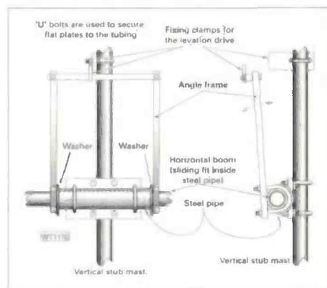
**Fig. 3b: This system again uses a simple sliding-fit pivot, but this time driven by an extension arm drive, which may be cheaper and easier to set up than the system of **Fig. 3a**.**
