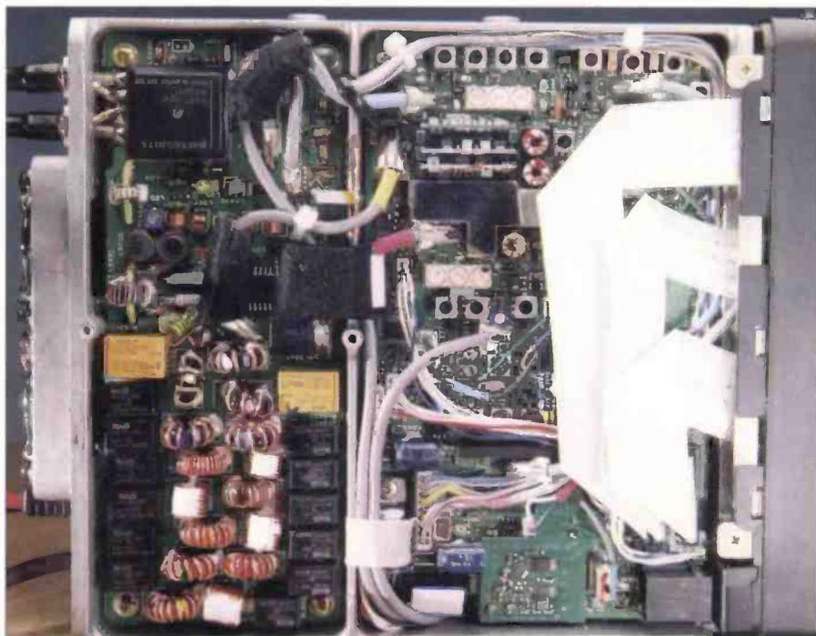
Fig. 8: Inside view of the upper chassis unit of the transceiver illustrating the complex ribbon-wiring assemblies on the right. The twin cooling fan housing can be seen on the far left.
