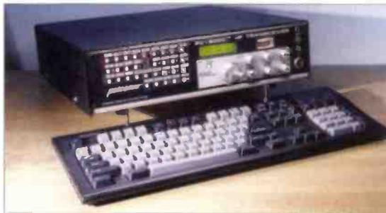
The Patcomm PC-16000 h.f. transceiver comes complete with a keyboard as standard.
