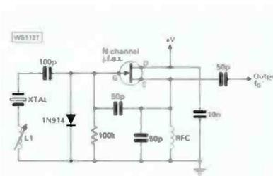
Fig. 3: A simple VCO based on a quartz crystal whose output frequency can be reduced a few kHz below the crystal's fundamental frequency by adjusting the inductance of L1.
