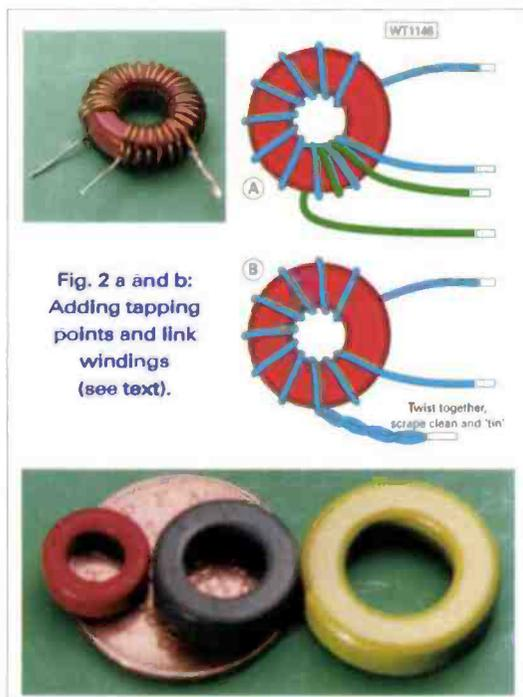
Fig. 2 a and b: Adding tapping points and link windings (see text).
