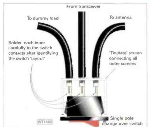
**Fig. 1:** A simply made changeover switch design, 'doodled' by Steve GM0PCD.
