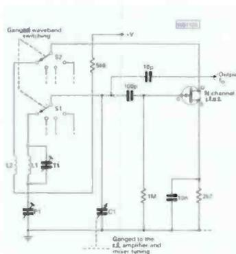
Fig. 2: The l.o. of a four band receiver based on an n-junction f.e.t. The tuned circuit and feedback of only one band is shown. The other three are similar except for component values. This v.f.o. is tuned over the selected band by C1.
