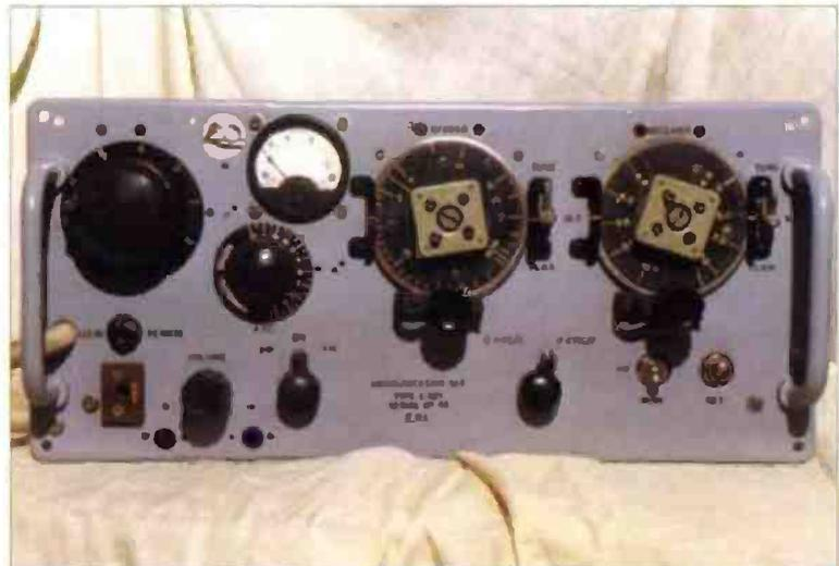
Fig. 4: The front panel of the X32D after a week's restoration work. Not quite finished but at least it's now starting to look like a military set.
