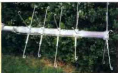
Fig. 3: The resonator adjusters: The resonator elements, showing construction of the resonators with their spokes and adjusters.
