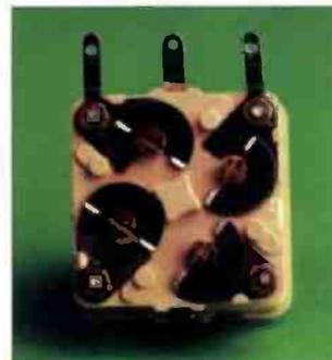
Fig. 2: Example of a miniature solid dielectric capacitor with fitted 'trimmers' (see text).
