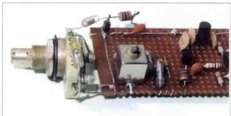
Fig. 6: Close-up photograph showing the simple modifications using the B105B varicap diode (see text).
