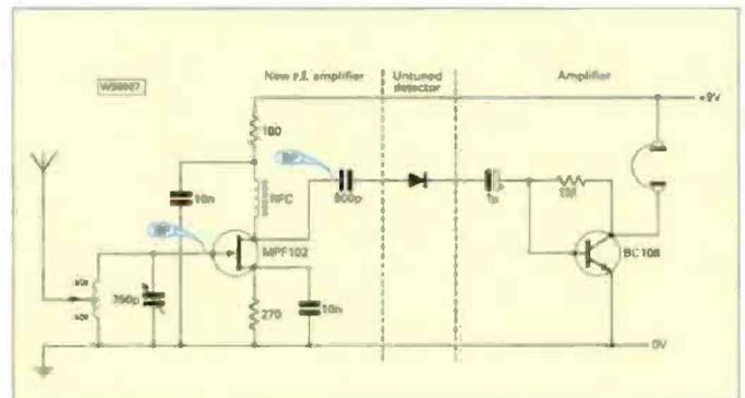
Fig. 2: Testing the r.f. amplifier on Receiver 2 (see text).
