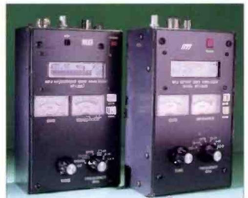
The MFJ-269, on the left side-by-side with the MFJ-259B. Although the limit on s.w.r. readings at u.h.f. is only a maximum of 5:1, it is extremely useful nonetheless.
