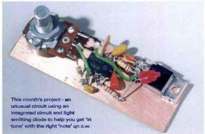
This month's project - an unusual circuit using an integrated circuit and light emitting diode to help you get 'in tune' with the right 'note' on c.w.
