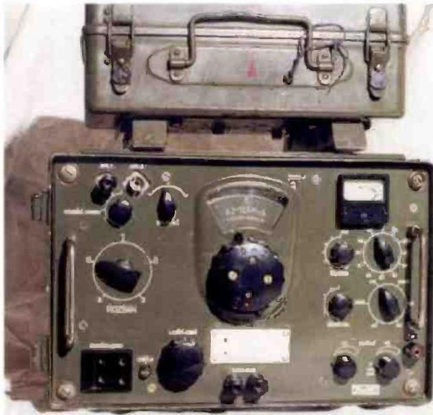
Fig. 2: The R-4C receiver, main tuning lower left, with headphone sockets bottom left and S-meter/voltmeter top right. (The p.s.u. plugs in at the rear).
