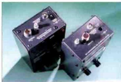
The MFJ-269 on the left with the MFJ-259B to its right shows that the modifications are more noticeable on the top panel. Note that the output socket is now an N-type rather than the SO-239 of its forerunners.
