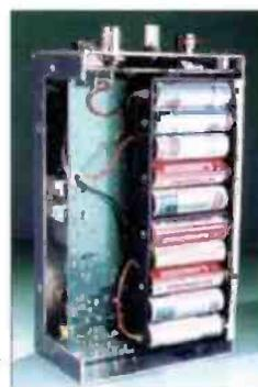
There are eight countersink-headed screws to remove to gain access to the battery holder (similar to the MFJ-259). So, rechargeable NiCad or NiMH batteries are now the order of the day.
