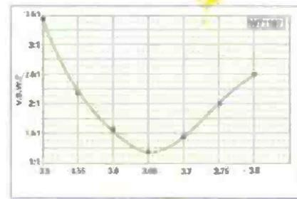
Fig. 4: SWR of the 3.5MHz dipole across the band referred to 75Ω
