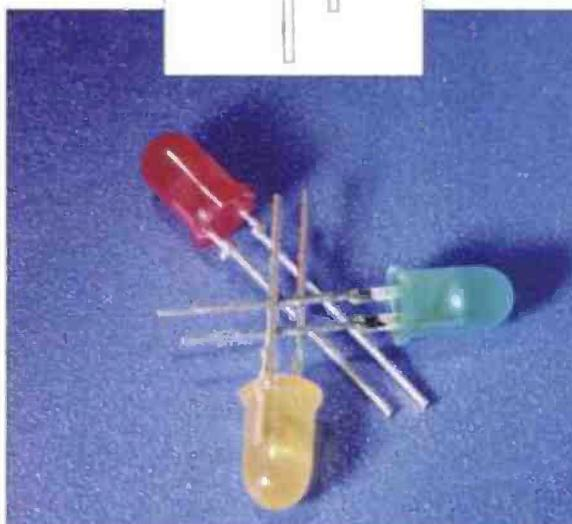
Fig. 3: You can use a colour of your own choice for the i.e.d. in the circuit ... but remember that the longer lead goes to the positive (+) supply).
