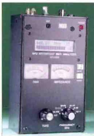
Looking very like its predecessor the MFJ-259B, the new MFJ-269 measuring from h.f. to u.h.f., is altogether a rather more capable unit.
