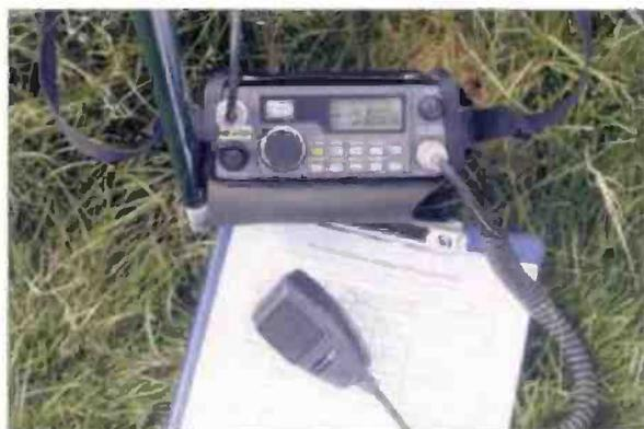
Fig. 2: Phil M0AYB uses a Yesu FT-290 MkII 2.5W portable transceiver for his portable contesting.
