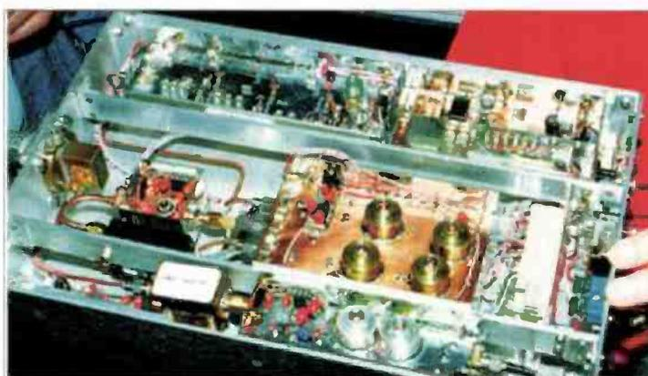
Fig. 1: The G3WDG/G4DDK 10GHz transverter kit.
