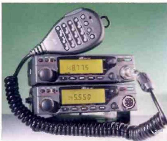
The new ADI AR-147 transceiver (top) and older AR-146 (bottom). The AR-147 covers 144MHz and provides 'receive only' on the 'Air Band'.
