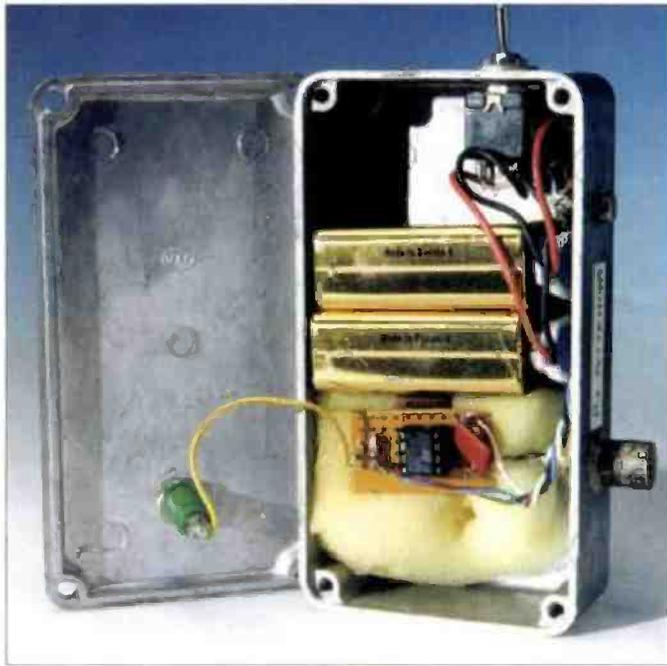
Fig. 4: ... and a diecast box to put the amplifier and batteries in. Then you have your v.p.a.
