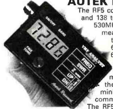
The RF5 covers 35 to 75 MHz, and 138 to 500MHz (typically 530MHz) in 3 bands. It measures RF values of true impedance (0-600Ω), SWR (1 to 6:1). It has no direct L & C as the RF1 but an INSTANT SWR mode which finds the frequency of minimum SWR (or Z) on command automatically. The RF5 fits in the pocket,
