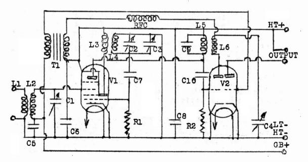
The circuit consists actually of three stages. The first. using a triode-hexode frequency changer such as the 6K8, converts all incoming signals to a fixed frequency which is fed to the second stage. This is one half of a twin triode (608 or similar) which is wired as a leaky grid detector with preset reaction. The other half of the twin triode is an audio amplifier stage.
