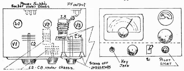
It must be noted that the spindles of C8 and C14 are at full HT potential. The coils used at present are the Premier range for 320, 160, 80, 40, and 20 metres. The VFO coil, L1, should be one band lower in frequency than the desired output, except in the case of 20 metre working when the oscillator is run on 80 m, L2 on 40 m and double in the PA.
